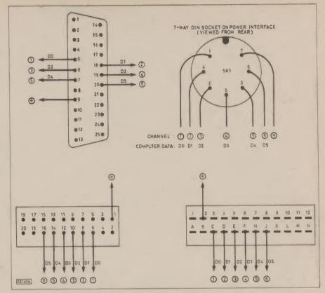
Fig. 6. Connections to DIN socket and user ports.
