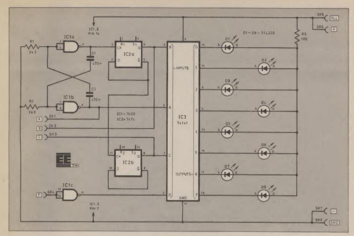
Fig. 1. The circuit diagram of the Truth Table Display
