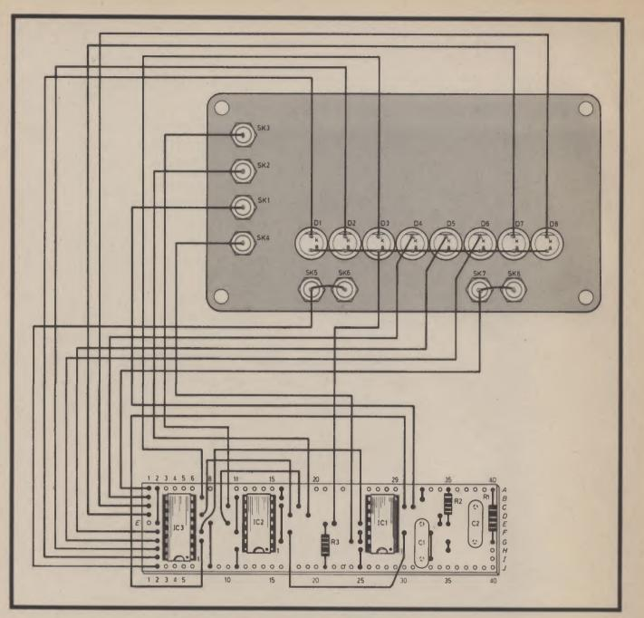
Fig. 8. Wiring diagram and component layout of the Truth Table Display
