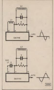
Fig. 2. Capacitive effect with LI o/c.
