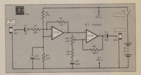
Fig. 1. Circuit diagram of the Microphone Preamplifier.
