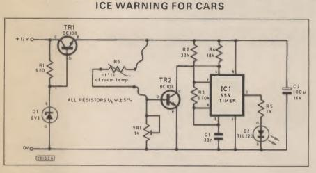
T HIS is a very useful device, especially in the winter, as it gives a visual warning of icy conditions. The unit should be placed at the front of the car in a position best suited for exposure to the elements. When the circuit is built it can be calibrated by placing the thermistor, R6, in a bucket of icy water and the l.e.d. can be made to light by adjusting VR 1.
