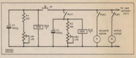
(variable up to about 10 seconds by the pre-set VR1) the relay RLA is "on" and the washer motor will be in action.
