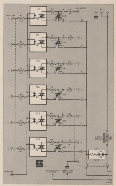
Fig. 1. Circuit diagram for the Power Lighting Interface.
