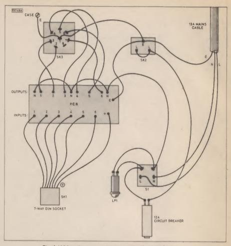
Fig. 4. Wiring diagram for the Power Lighting Interface.
