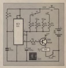
Fig. 1. The complete circuit diagram of the Games Timer.
