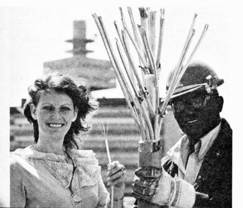
Optical fibre cable (left) that will replace the old style metal conductor and metal sheathed coaxial cable (right) in modern telecommunications networks are shown for comparison in this British Telecom picture. Optical fibres have a much greater transmission capacity than traditional coaxial cables. Pulse rates in excess of 140 million per second have been achieved over distances of 100km without intermediate amplification.
