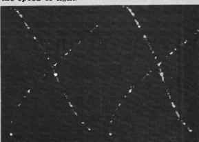
Stereoscopic photo of electron tracks using a cloud chamber.
