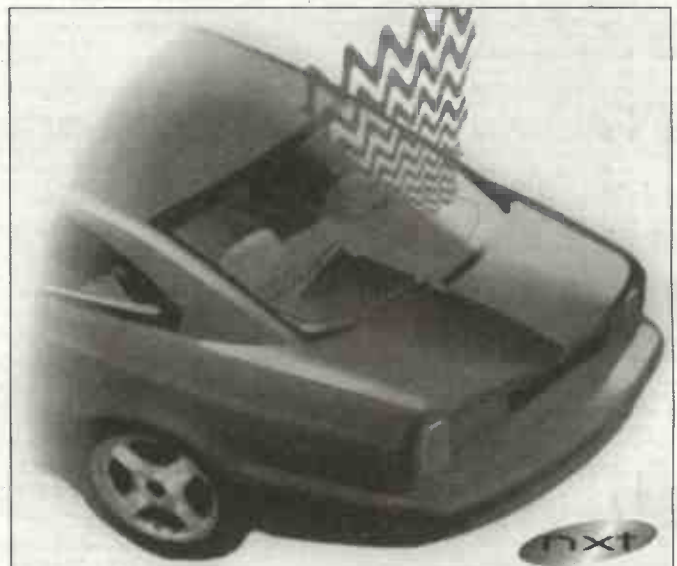
NXT speakers integrated with rear parcel shelf of a car, acting as a structural member. The nature of NXT sound provides uniform sound distribution in the car environment without any hot spots.
