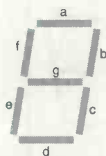
Figure 2: the segments of the LED display
