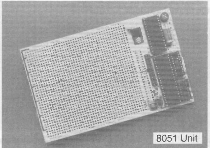
The 8051 series board has provision for an RS232 port (you just need to insert 1 chip). It can be used with processors with inbuilt EPROMs (such as the 8751 or 8752) or external program memory (such as the 8031 or 8032). For use with external memory, it has the address latch tracked in so you just add a 74HC573. It can be used with any 40 Pin standard Pin Out device in the range. Can be used with the training system on page 11.
