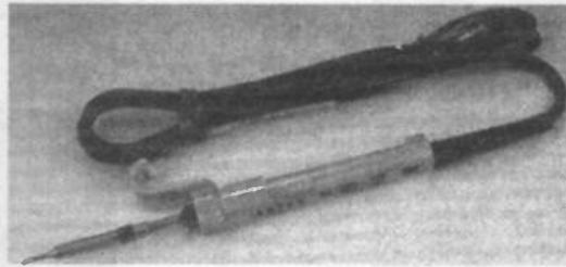
Model XS is a 25 Watt soldering iron which contains all the best constructional features incorporated during many years of soldering iron manufacturing, such as putting the element inside a stainless steel shaft and then using a slide on bit to cover both the shaft and the element for maximum efficiency.
