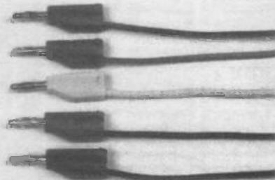
Five coloured coded test leads fitted with 4mm stackable banana plugs on both ends. Capable of carrying max current of 0.5A, 1 Metre long.
