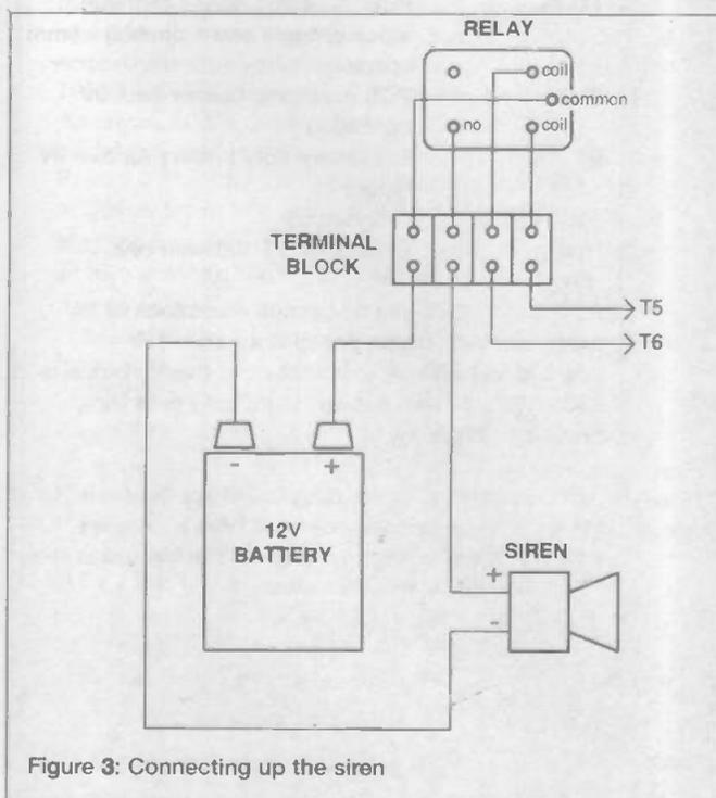
Figure 3: Connecting up the siren
