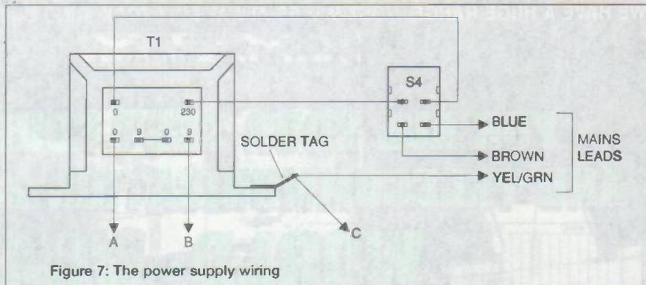
Figure 7: The power supply wiring
