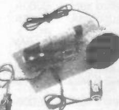
Based on the popular ZN414, a miniature pocket radio kit that includes all components including tuning capacitor, headphone socket and crystal headphone. Excludes PP3 battery. Small enough to fit into your pocket but sensitive enough to pick up distant radio stations.
