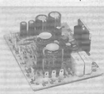
A compact stereo amplifier that will operate from a wide range of supply voltages. It can deliver 2x10W or 1x20W depending on connection.
