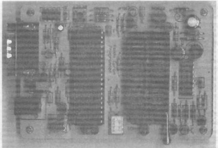
Programs all types of 28 pin EPROMs. Fully microprocessor-controlled and comes complete with a professional ZIF socket. Includes on-board power supply to provide the correct programming voltages, especially the 6V Vcc supply that ensures long term reliability (a feature that is missing on many other units). Also features Eprom read, which gives an output file for our Disassemblers.
