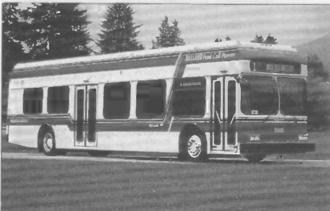
Figure 6: Current design of the second generation Ballard Bus, with a 275 HP Ballard Fuel Cell engine. (Courtesy Ballard Power Systems Inc)
