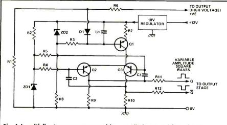
Fig. 4 A multivibrator arrangement with controlled output drive voltage.
