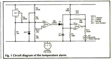
The LM334Z is a current source IC which has a linear variation in output with temperature. This feature can be a nuisance if you actually want to use it as a current source, but is very useful for making thermometers and suchlike. The current from the LM334 develops a voltage across R1 which is compared with a reference voltage set by RV1.
