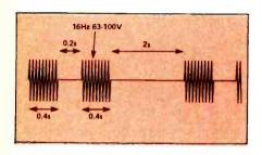
This device answers your telephone after a few seconds delay and then hangs up on the caller. The circuit requires no external power but operates on the AC ringing signal which is transmitted by the exchange to your phone. This is usually a 16Hz voltage with an amplitude in the range 63 to 100V with cadences as shown in the first figure.
