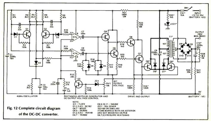
lower the DC resistance, and a secondary of 42T also of 1mm wire insulated from the primary by a layer of PVC tape.
