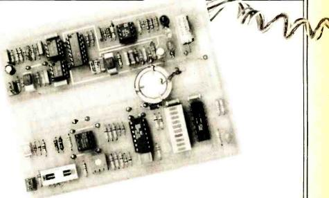
inputs are low the oscillator is inhibited. The frequency of the oscillator thus indicates the input logic levels. Low for logic low, high for logic high, off for indeterminate and a pipsqueak for pulses and transitions! A piezo sounder is used as the transducer.
