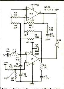
Fig. 2. Circuit diagram of the bridge amplifier.
