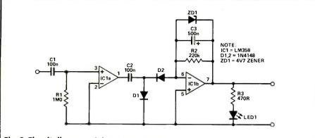
Fig. 2 Circuit diagram of the touch switch.
