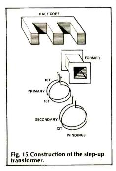
are given in Fig. 15, and the wire used should be 1mm enamelled copper. Most of the transformer kits available are supplied with a coil former which already has a 120/240V mains winding. This must be discarded and a new former made up from stiff cardboard. The E and I laminations are then fitted into the former and the completed core secured as recommended by the kit supplier, usually by means of end-cheeks which are bolted together through the laminations.
