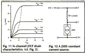
Because of the wide spreads in  $V_{gs}$  (off) and  $I_{dss}$  for different FETs, a variable resistor is used to set the current. This is not very satisfactory as it adds extra time and costs in manufacturing. An alternative is to manufacture FETs with built in resistors to give a fixed current from a two terminal device (Fig. 12). These can be obtained from Siliconix for currents from 200mA to 5mA. Tolerances vary from 10% for the CR022-CR470 devices down to 30% for the J553-J557 devices.
