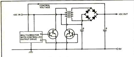
Fig. 2 A DC-DC converter with push-pull drive.
