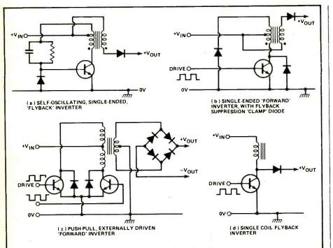
Fig. 1 Various circuit arrangements for an inverter.
