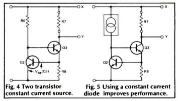
stabilises Q3's base more effectively. The dynamic impedance of the two transistor circuit is 20 times the impedance of its equivalent resistor compared with about four times for the single transistor circuit. Further tests showed that with resistor R6 in circuit the impedance was constant up to 100kHz. If R6 was replaced by aJ503 constant current diode the impedance decreased with increasing frequency (Table 3).
