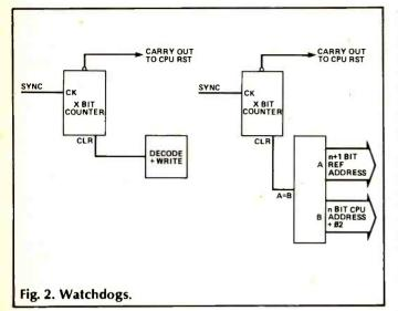
look for addresses which should not be generated, and allow N of them to cause a system reset. This second approach is definitely the more flexible and is totally transparent to software. If you are really crafty, for a small penalty in terms of reliability, you could use write protected registers to hold the comparator settings so that individual applications packages could set the watchdog to suit themselves.
