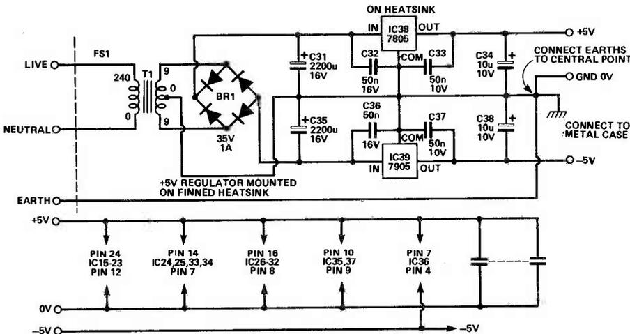
Fig. 7 Circuit diagram of the power supply.
