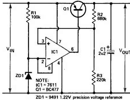
reference which gives a very stable 1.22V and can operate from a current as low as 50µA. This reference voltage is fed to the inverting input of a CMOS op-amp where it is compared with a fraction of the output voltage. The output of the op-amp drives the base of the BC477 and this transistor increases the output current of the amplifier.
