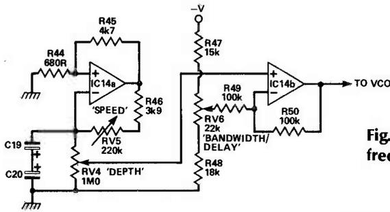
Fig. 6. Circuit diagram of the low frequency oscillator.
