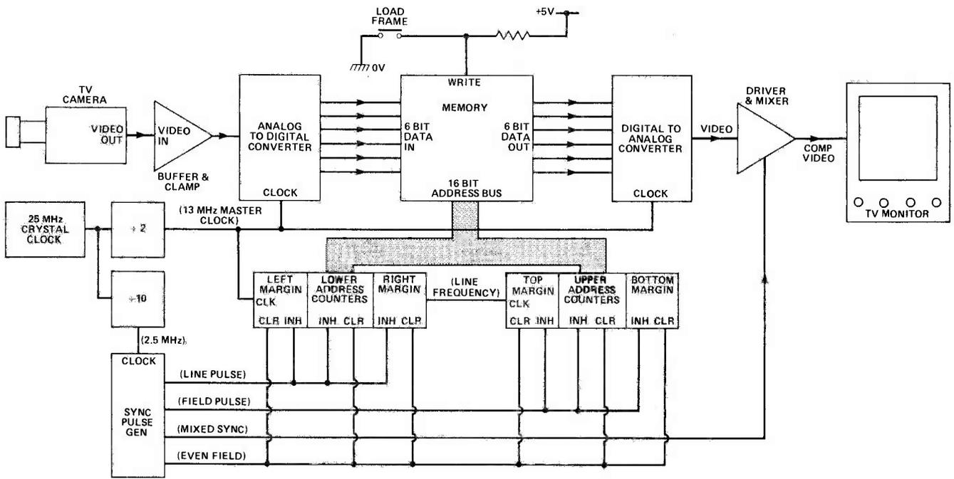
end of a frame the address counters are reset by the sync pulse generator and the process continues again.
