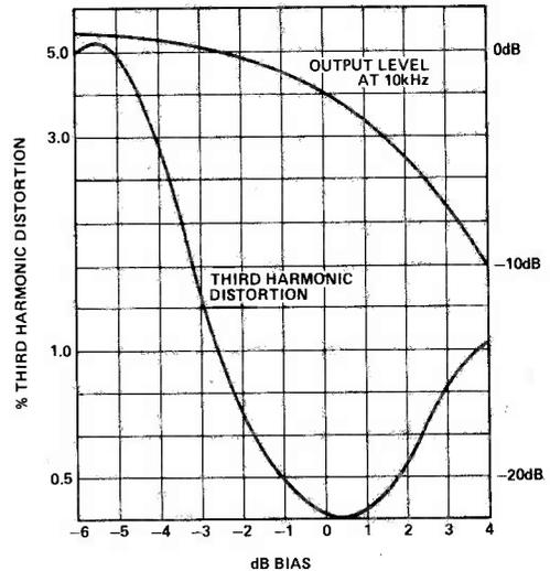
Fig. 7 Relationship between distortion and frequency response with a change of bias level. Optimum point for minimum distortion also produces a drop of 3 dB in the 10 kHz signal level (for one brand of C120; tapes vary in amount of distortion and HF loss).
