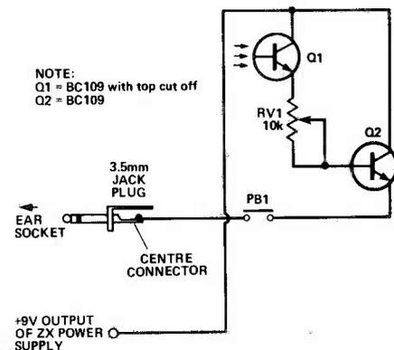
amount of light required for switch-on can be adjusted by RV1 to suit different colours on the screen.
