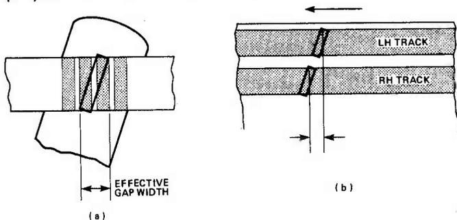
Fig. 9 When azimuth is not vertical, gap bridges across short wavelength zones, increasing its effective width and thus losing the high frequencies, (a). With a stereo head, (b), incorrect azimuth produces a delay between channels which can impair stereo image by upsetting the phase relationships. Azimuth errors shown here are exaggerated for the purpose of illustration.
