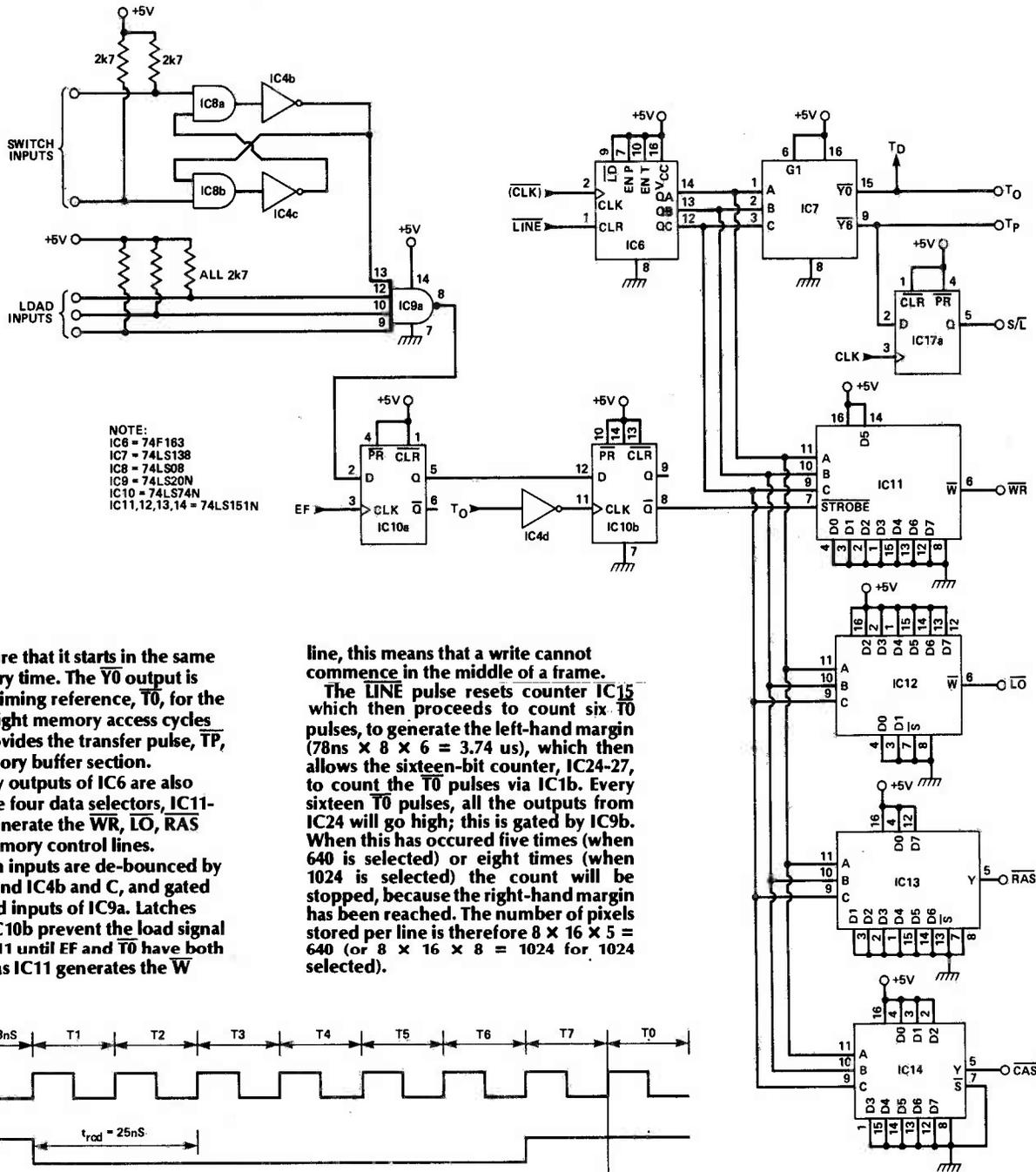
**LINE** to ensure that it starts in the same position every time. The **Y0** output is used as the timing reference, **T0**, for the first of the eight memory access cycles while **Y6** provides the transfer pulse, **TP**, for the memory buffer section.
