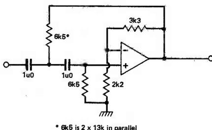
Fig. 4 Circuit for a second-order filter.
