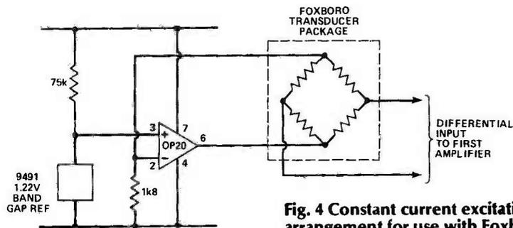
Fig. 4 Constant current excitation arrangement for use with Foxboro transducer.
