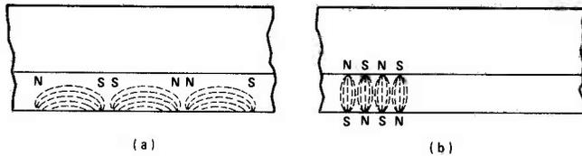
**Fig. 4** Conventional recording heads produce longitudinal magnetic zones in the tape coating, with NS, SN, NS polarity, (a). Perpendicular recording in which the tape passes between the recording poles gives a greater packing density, and N, S, N, S adjacent pole polarity.
