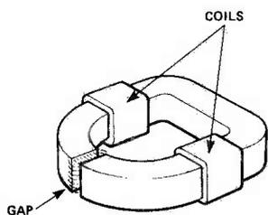
**Fig. 1** Magnetic recording head showing core, gap and coils.
