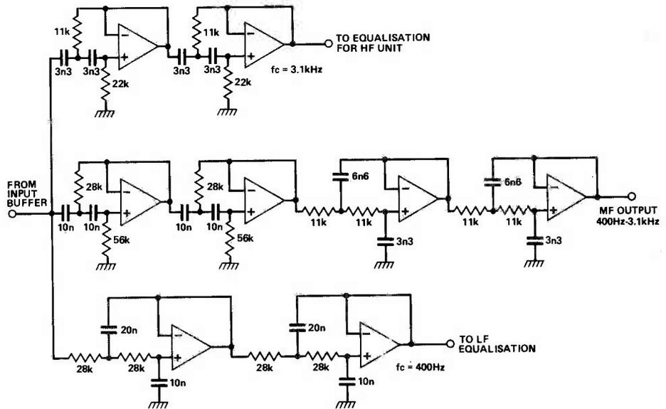
Fig. 2 Basic circuit diagram for a three-way cross-over. You'll have to work out the details (and the PCB) yourself.
