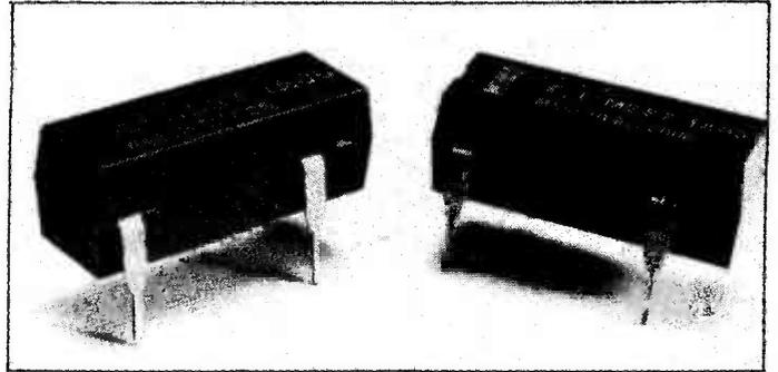
optional modification, the addition of a transient suppression diode to the coil, is available on both types.
