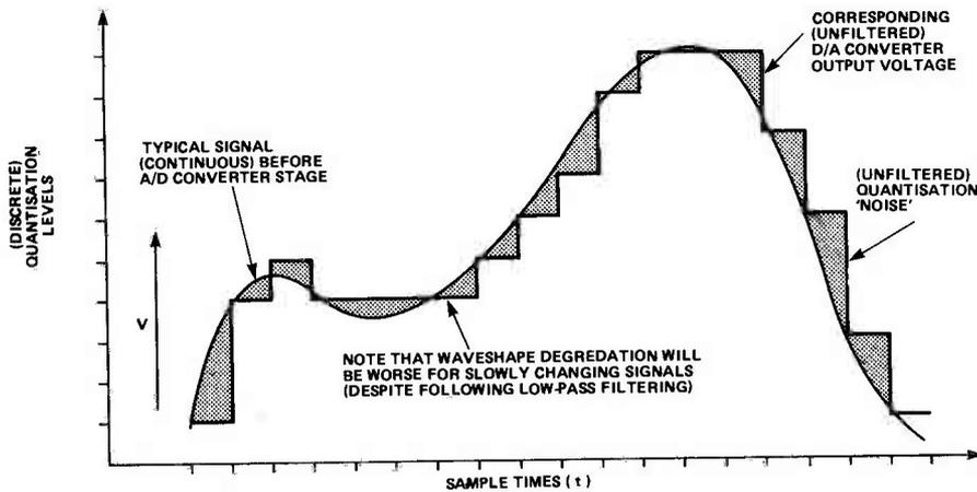
Fig. 1 The generation of quantisation noise during A-D conversion.
