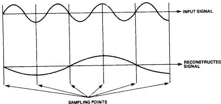
Fig. 2 How the use of too low a sampling rate leads to the reconstruction of a different 'alias' frequency.
