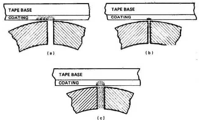
**Fig. 3** A wide gap in a recording head can record short wavelength signals by overlapping and partially erasing the previous half-cycles. External gap from the field is roughly hemicylindrical (semi-circular when viewed from the top) and the depth of the field in the tape is roughly half the gap width (the gap is the diameter of the circle and the depth the radius). A narrower gap (b) leads to a smaller depth than a wider gap (c).
