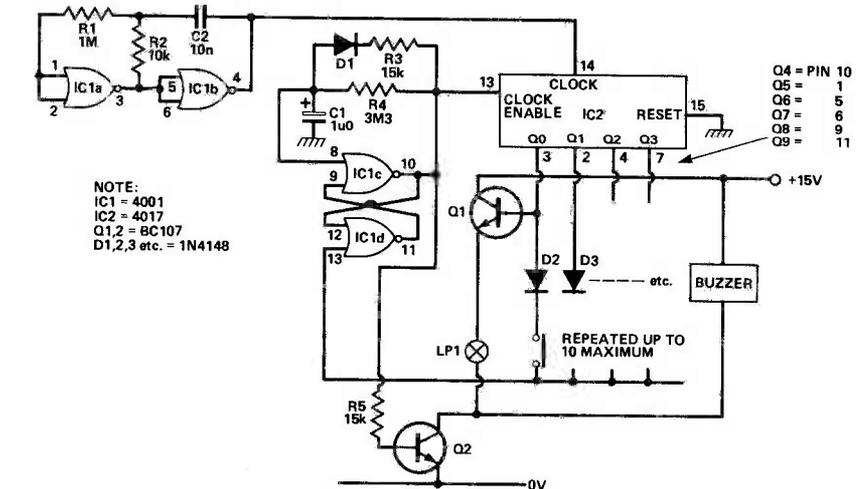
indicating that PB1 has been pressed. LP1 remains lit for a time period set by C1, R4 (approx. 3 seconds) after which the bistable is set via pin 8. Lamp LP1 is then extinguished and the circuit is ready for another round.
