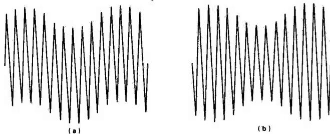
Fig. 6 The difference between a superimposed signal (a) and a modulated one (b). With the superimposed signal, the amplitude of the high-frequency component remains unaffected, hence it is not modulated.
