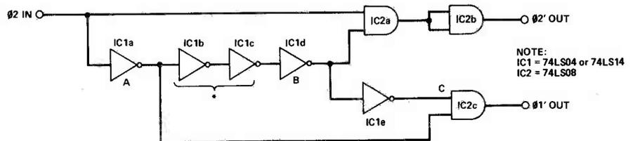
\*OMIT OR REPLACE WITH 1 SECTION OF 'LS08 FOR SHORTER  $\phi_1$  DELAY. INSERT SPARE SECTION OF 'LS08 BETWEEN INVERTERS FOR LONGER DELAY
