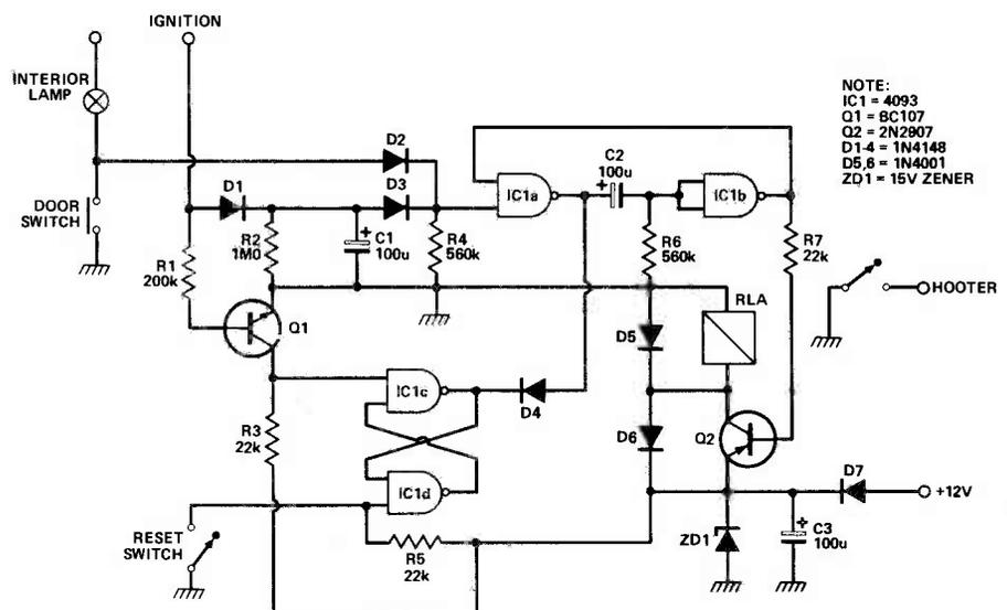
magnetic switch was used in the prototype). This causes the NAND latch around IC1c and IC1d to set, putting an earth on D4 which will reset the monostable. The car can now be entered without fear of sett-
