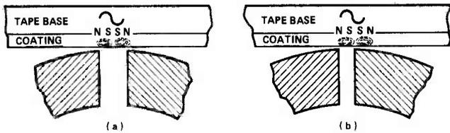
**Fig. 2** When the playback gap is equal to a whole recorded wavelength, the fields of opposite half-cycles cancel and produce zero output (a). When the gap is equal to half a wavelength (b), output is at maximum.
