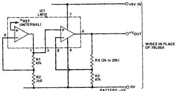
Fig. 2 Adjustable regulator arrangements to replace the 78L05A.
