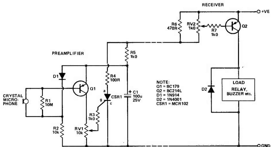
delay to prevent CSR1 triggering at switch-on.
