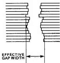
**Fig. 8 Laminated stack with imperfect alignment. Effective gap width is increased. With widths of little more than one micron, small irregularities matter.**
