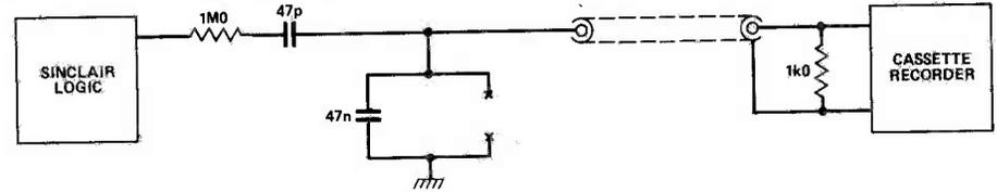
much smaller than the 5V logic level, the input signal-to-hum ratio becomes very large and reliable data transfer is much more likely.
