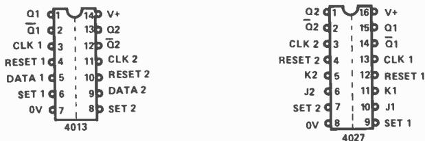
Fig. 1. Outlines and pin notations of the 4013 dual D and the 4027 dual J-K CMOS flip-flops.
