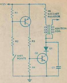
Transistor assisted ignition
