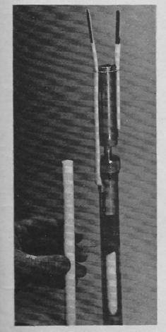
Fig. 12. Actual cell of ECRC Na-S cell showing the Beta-alumina tube used as a solid electrolyte.
