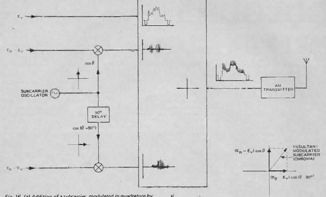
Fig. 16. (a) Addition of a subcarrier, modulated in quadrature by both colour difference signals to the luminance signal Ey. (b) Vector representation of subcarrier.
