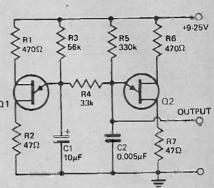
This circuit was evolved to provide a highly stable and ripple-free voltage to act as the reference for the stabilised power-supplies of an electronic music synthesiser; the stability of its voltage-controlled oscillators depended directly on the constancy of supplyrail voltages.
