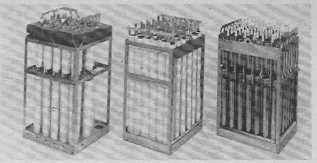
Fig. 13. Three stages of development increased packing density of the ECRC cells into the battery module. They must be electrically insulated from each other at an operating temperature of around  $350^{\circ}$ C.
