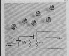
The new Plessey PPC 522 low-cost broadband ceramic pyroelectric infra-red detector which comprises a detector element and J.F.E.T. preamplifier encapsulated in a TO5 transistor can, with a suitable cell window according to the required application. These devices are specifically designed for intruder detection, fire alarm and pollution monitoring applications.
