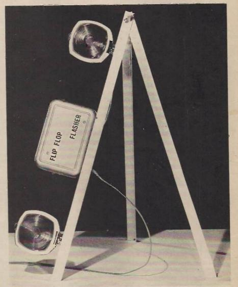
legs can separate by an angle of only about 32 degrees. The third leg is attached to a small bracket made from the same aluminium angle, and shown in Fig 10. The bracket is attached to the front legs by the bolt and wing nut which holds them together. The rear view arrangement is shown in Fig 11, and from this it can be seen how the rear leg is kept central.
