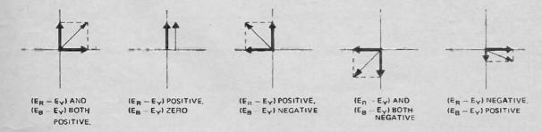
Fig. 18. Typical chroma vectors (thin arrow) produced by various values of  $(E_R - E_y)$  and  $(E_q - E_y)$  modulated as in Fig. 16.
