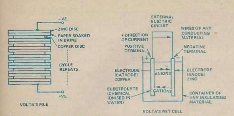
Fig.2. Cross sectional diagrams of the first electrochemical cells - VOLTA'S pile and wet cell.
