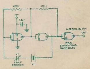
Fig.4. Reliable TTL crystal oscillator.
