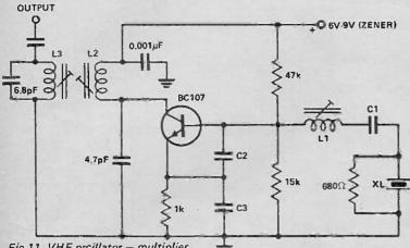
65 MHz Xtal 130 MHz OUTPUT L1 = NEOSID AZ ASSEMBLY (4mm FORMER & F29 SLUG) WOUND WITH 12 TURNS OF 4.55 mm ENAMEL WIRE, CLOSEWOUND
