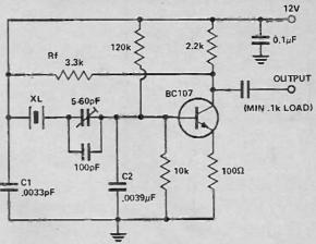
Fig.6, Parallel mode LF oscillator.
