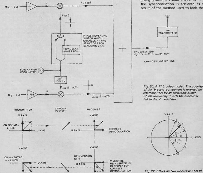
Fig. 21. Inversion of V signal on alternate lines in the PAL system.
