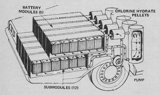
Fig.9. Layout of chlorine-zinc battery installation in a vehicle.
