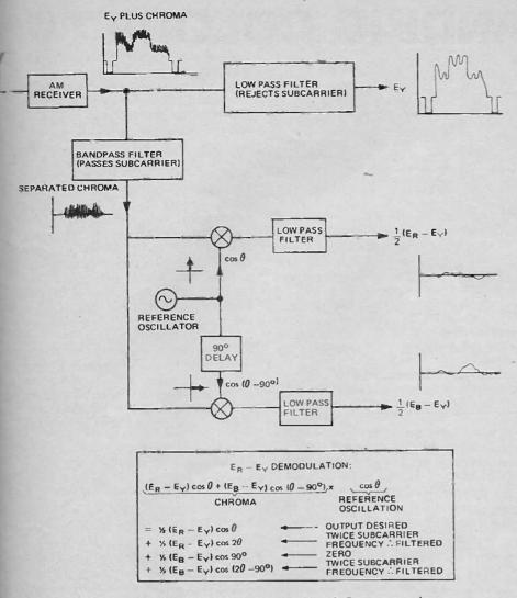
Fig. 17. A suitable receiver for the signal produced by Fig. 16. For correct colour demodulation the reference oscillator must be precisely phase-locked to the transmitter. The insert shows a full description of the  $(E_R - E_Y)$  demodulator; the  $(E_B - E_Y)$  demodulator works similarly.
