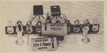
Fig. 8. Actual tag strip for negative earth version. Note the wire joining the two tags above the mounting feet, and also the use made of the lower holes in the tags.
