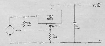
Fig 3: A circuit for use in a car or where the supply voltage is 9 to 18V.
