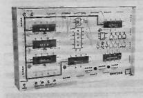
This advanced logic trainer has been designed for teaching the principles of binary arithmetic and four-bit data word manipulation.
