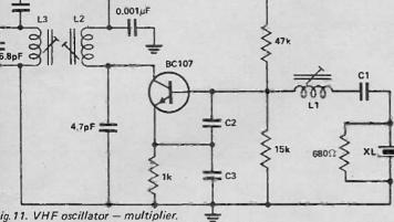
Fig. 11. VHF oscillator - multiplier.
