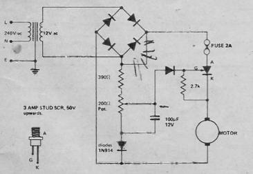
The following is a low voltage adaptation of the type of speed control popularly used to regulate power drills. It gives very good starting torque and excellent speed regulation of the model. A reversing switch may be incorporated in the leads to the motor.
