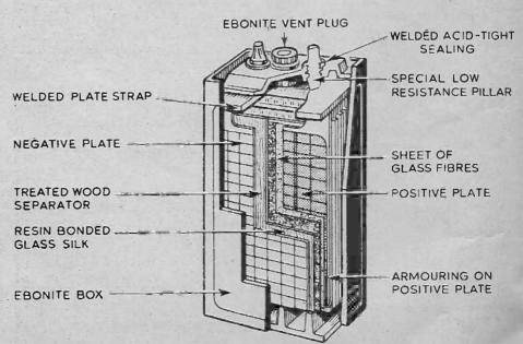
Fig.7. Interior of lead-acid storage cell. Electricity is stored by virtue of chemical reactions induced by charging the cell with electricity.
