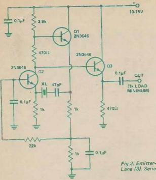
Fig.2. Emitter-coupled oscillator – after Lane (3). Series mode.
