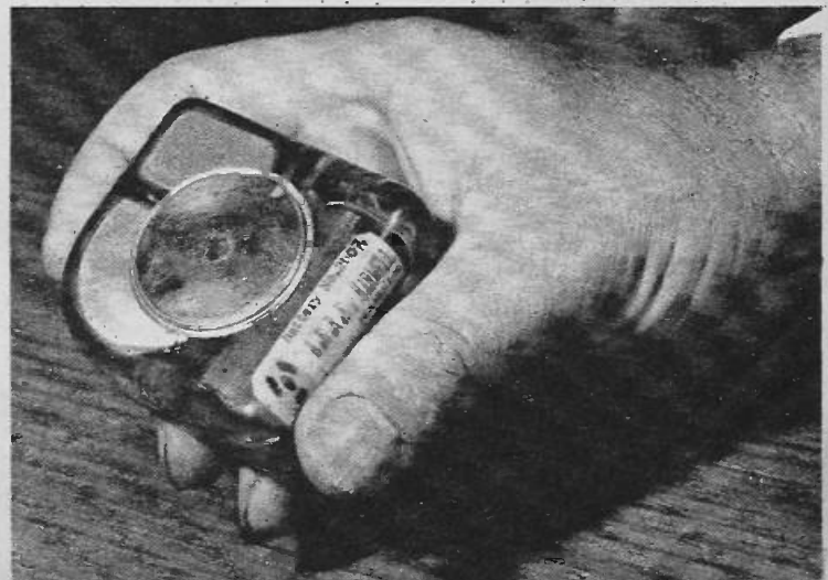
This isotope battery powered heart pacemaker was successfully implanted in a patient on July 15, 1970. The unit is expected to operate for at least ten years.
