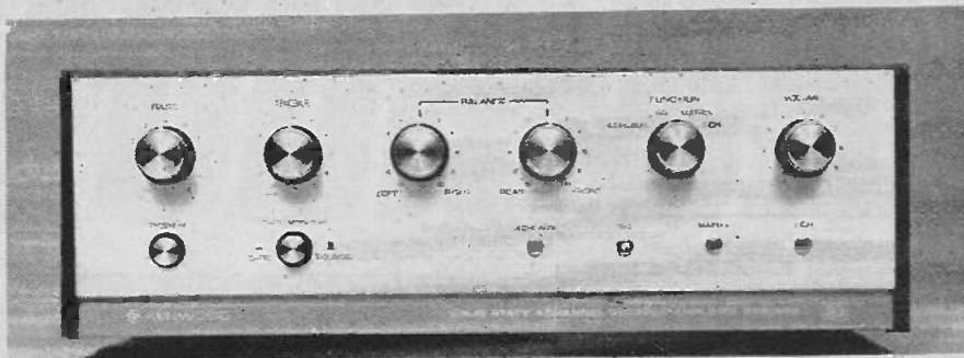
Four-channel amplifier and decoder from Kenwood has decoding circuitry for both SQ and non-SQ matrix systems.
