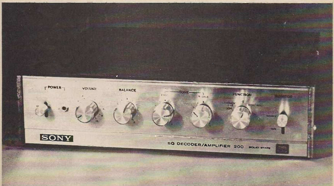
This unit has an amplifier and decoder combined.
