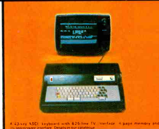
A 43-key ASCII keyboard with 625-line TV interface. 4 page memory and microprocessor interface. Details in our catalogue
