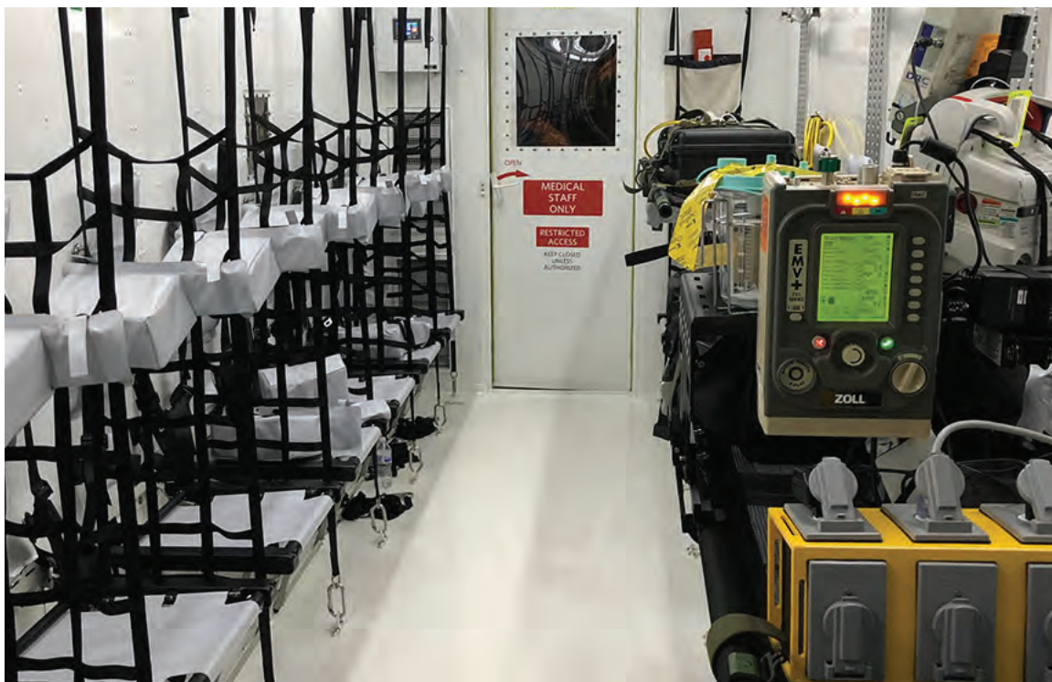
The inside of the NPC-Lite includes ambulatory patient seating (left) and litters with medical equipment (right)
