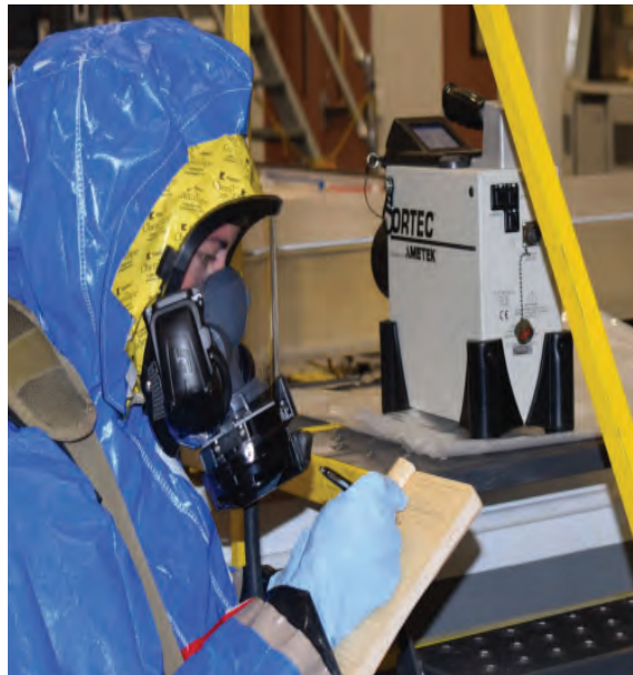
Picture 4. Characterization of Reactor Pool with Ortec Detective-DX 100T,
