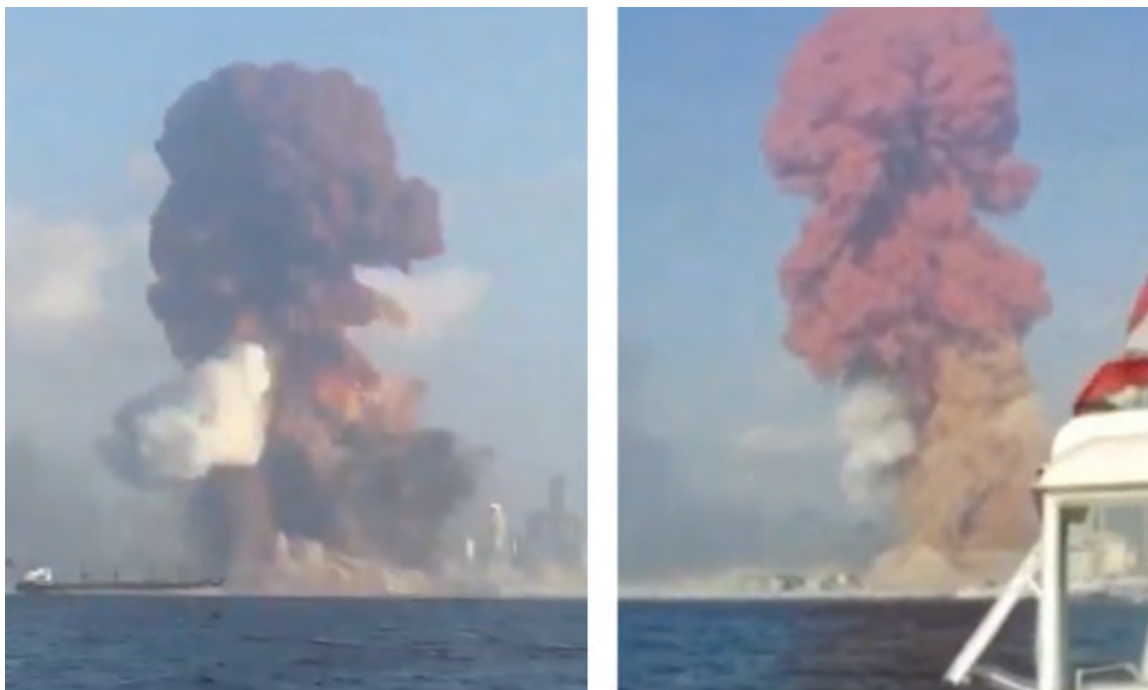
Figure 6. Late-time cell phone images of August 4th, 2020 Beirut explosion debris cloud. Note the maximum cloud height is about 7 or 8 times the maximum height of the buildings on the skyline in the images on the left. (Instagram, August 4th, 2020, YouTube, August 11th, 2020).
