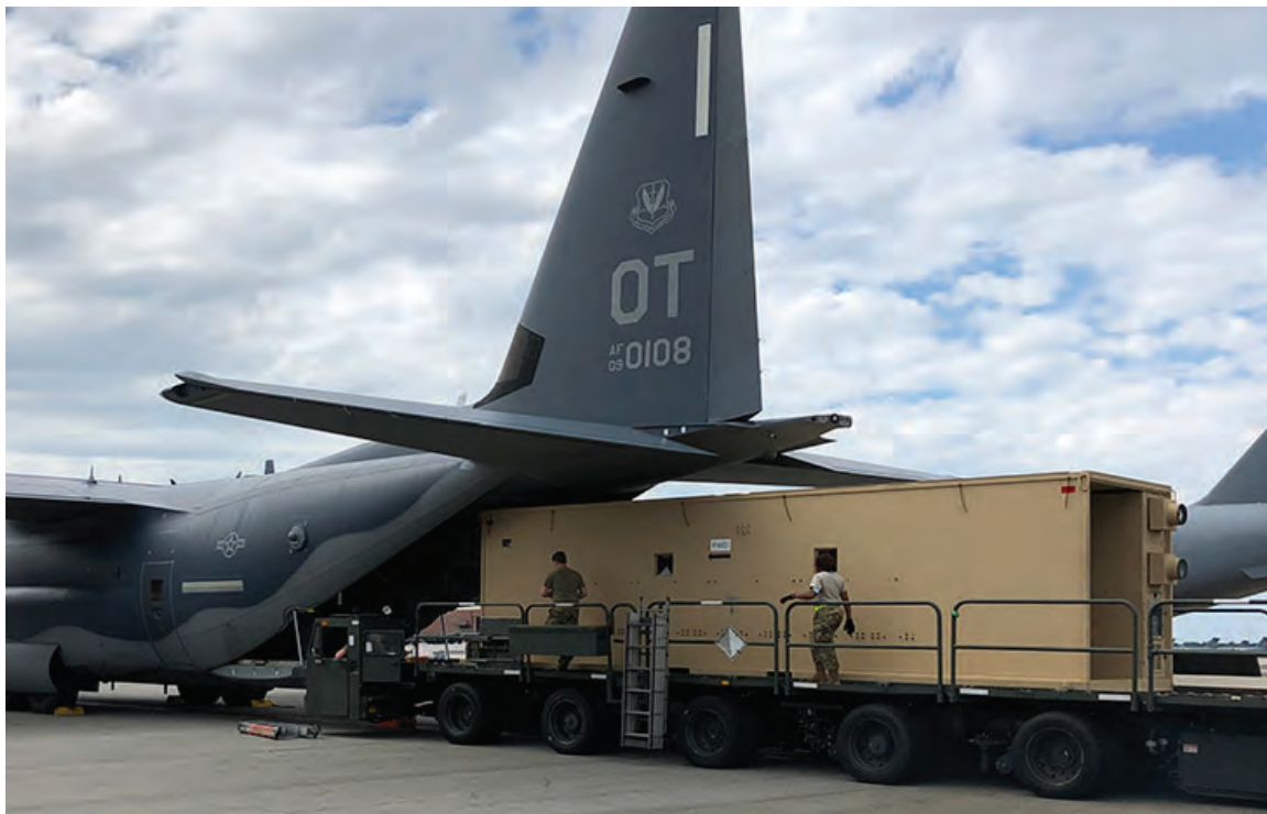
The Negatively Pressurized CONEX Lite system is placed inside an Air Force C-130 Hercules. The system is designed for transporting COVID-19 diagnosed and symptomatic warfighters out of forward installations and on to medical facilities. Picture by DEVCOM CBC
