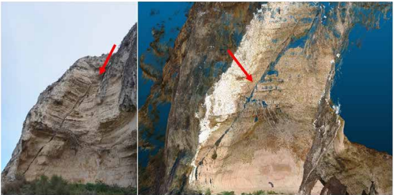
Fig. 1: Image of the fracture, on the left side; detail of the point cloud of the fracture on the right side.
