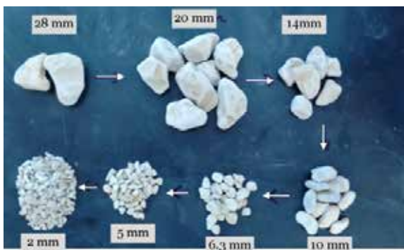
Fig. 1: Fragments of FR siltstone sample retained in the drum after five cycles in SDT [3].
