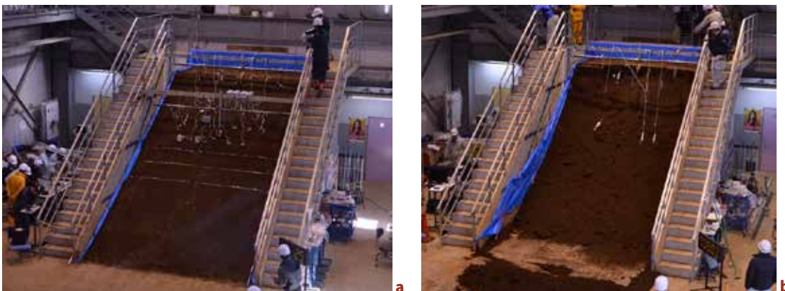
Fig. 1: Full-scale slope model test. a) initial time, b) The third collapse
