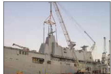
Synchronous hoisting and load positioning
