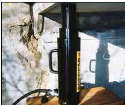
◀ The portable lock nut cylinder RACL-1506 used for extended load supports during epoxy injection for bridge reinforcement.
