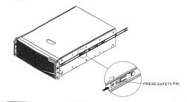
Press the safety locking pin to release the inner member from the chassis.
