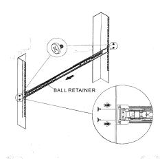
Align brackets to the desired vertical position on the rack and insert the fasteners.
