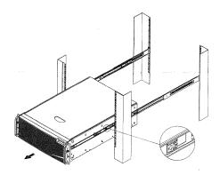
Fully extend the slides until it is in the locked position; pull the release button to release the lock and disconnect the inner member from the slides.
