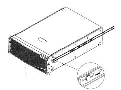
Align inner member key holes to standoffs on chassis; move the inner member in the direction shown here.
