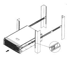
Pull the release button in the inner member to release the lock and allow the chassis to close.
