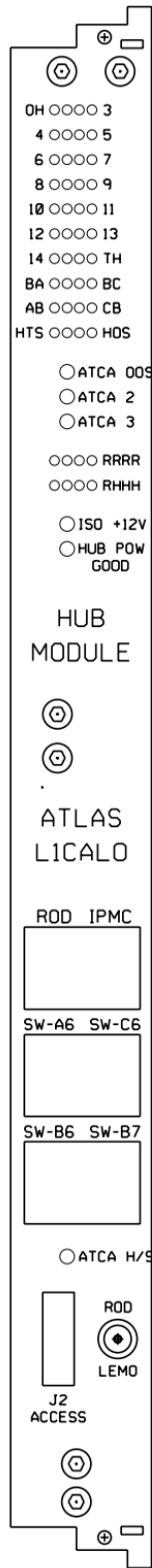
Figure 14: Hub prototype front panel silk screen.
