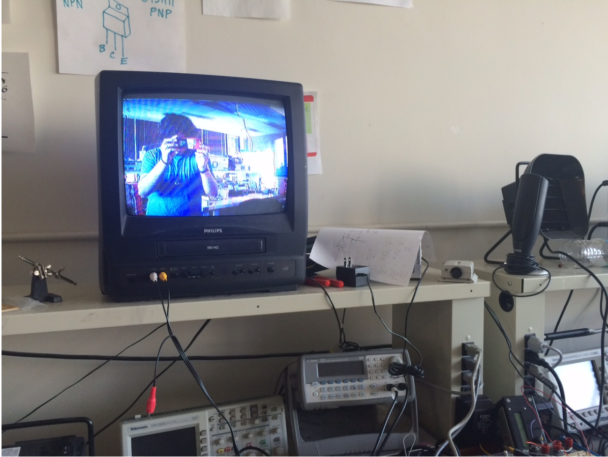
Figure 48: NTSC video signal output to the television after fiber optic transmission.
