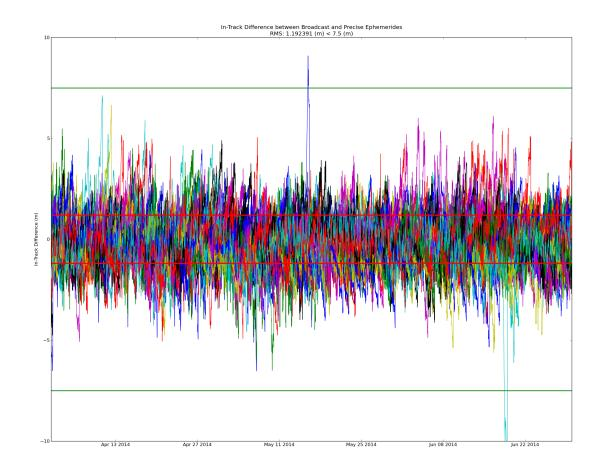
Figure 6.2: In-track ephemeris deltas between NGS precise orbits and broadcast ephemeris
