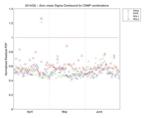
Figure 3.5: Daily GPS CNMP aggregate zero-centered sigma overbound values with glitch
