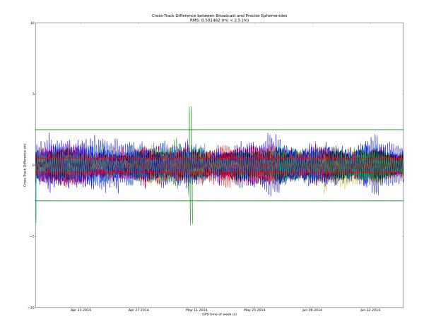
Figure 6.1: Cross-track ephemeris deltas between NGS precise orbits and broadcast ephemeris
