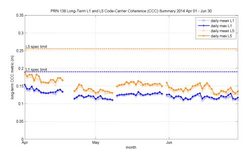
Figure 7.7: Long-term code-carrier coherence (CCC) for PRN 138
