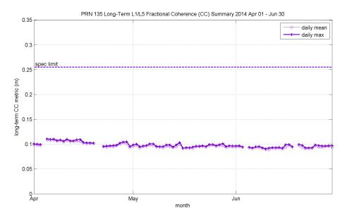
Figure 7.1: Long-term fractional coherence (CC) for PRN 135
