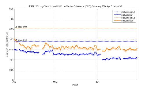
Figure 7.5: Long-term code-carrier coherence (CCC) for PRN 135
