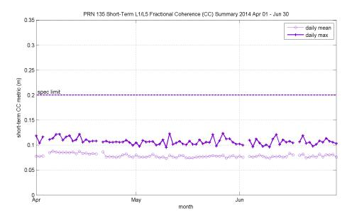
Figure 7.6: Short-term fractional coherence (CC) for PRN 135
