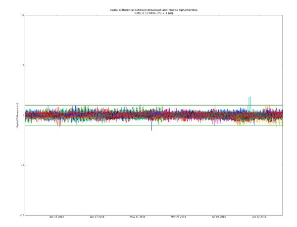
Figure 6.3: Radial ephemeris deltas between NGS precise orbits and broadcast ephemeris
