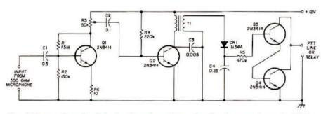
Flg. 1. The vox-box circuit is simple and requires only a few inexpensive parts. Wiring is non-critical. T1 is a small transistor interstage transformer, 1000-ohm primary, with a secondary of either 1000 or 2000 ohms, center tapped.
