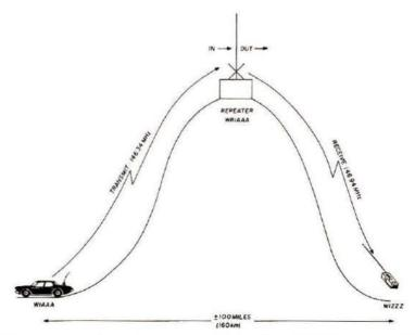
Fig. 1. The principle of repeater operation. A signal from W1AAA is received by the repeater on its input frequency, amplified, and retransmitted by the repeater on its output frequency where it is received by W1ZZZ. Since the input and output frequencies are different, no interference is caused at the repeater, and simultaneous reception and transmission can take place; since the mobile and hand-held are transmitting and receiving on different frequencies, they do not interfere with each other.
