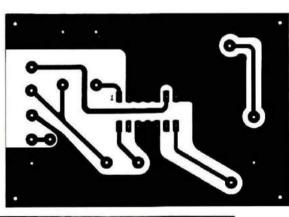
Fig. 2. Full-size printed circuit board layout pattern for the audio amplifier. A foilside view of the board is depicted above. An X-ray view from the component side is shown below.
