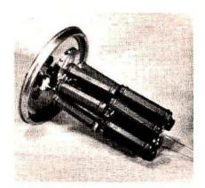
The completed resistor stack is shown attached to the connector and lid of the paint can, before it is inserted into the can and final soldering completed.
