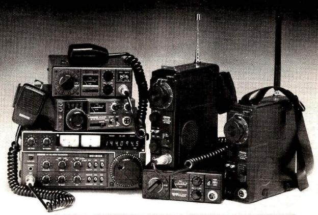
Clockwise from lower left: IC-211 4MHz, 2 meter, All Mode Transceiver; IC-245 Mobile 2 meter Transceiver; IC-225 Mobile VHF FM Transceiver; IC-502 Portable 50 MHz SSB Transceiver; IC-215 Portable 2 meter FM Transceiver; IC-30A Mobile UHF FM Transceiver.
