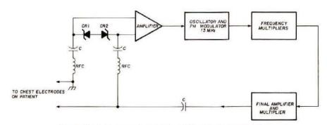
Fig. 4. Block diagram of a popular vhf telemetry transmitter.
