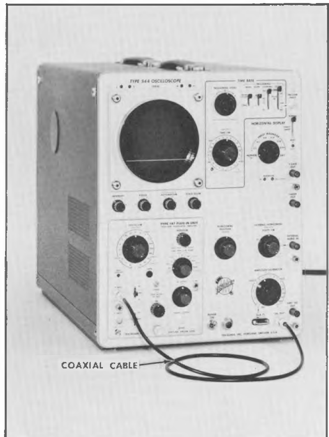
Fig. 2-2. Setup at completion of step 8 in the First-Time Operation procedure.
