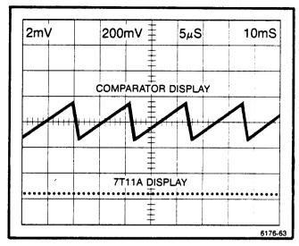
Figure 5-8. Typical display for adjusting Slewing Ramp (A2R310) and Servo Zero (A1R588).
