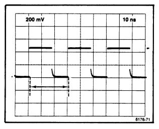
Figure 5-16. Trigger holdoff measurement.
