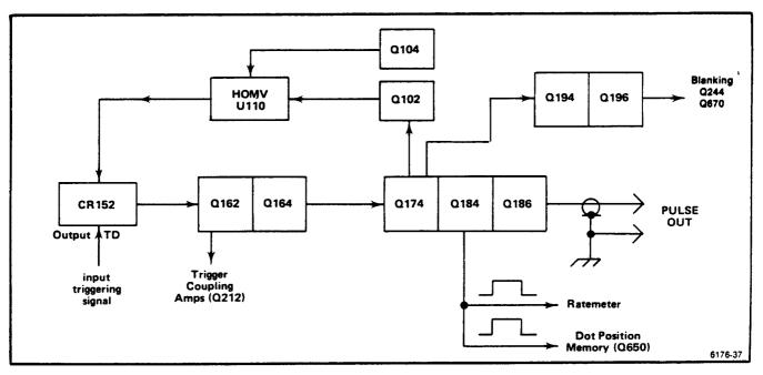
Figure 3-27. Trigger Output Circuits.
