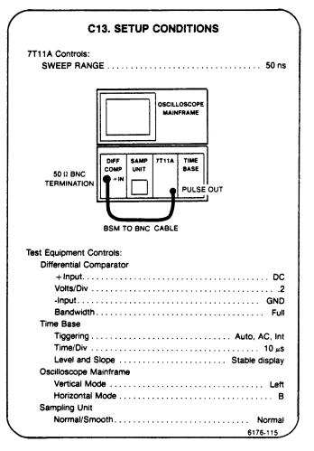
a. **EXAMINE**—the oscilloscope display to determine the trigger holdoff time. Use the settings and holdoff values given in Table 5-13 (see Figure 5-16 for a holdoff measurement example).
