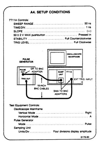
a. Set 7T11A TIME POSITION and TRIG LEVEL (if necessary) to view the pulse leading edge on the oscilloscope.
