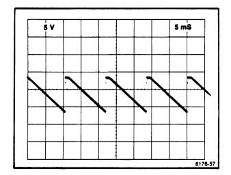
Figure 5-2. Sweep Out waveform to check Repetitive Scan rate.
