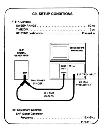
a. Set the Generator Amplitude and Sampling Unit Units/Div controls to provide at least 200 mV of trigger signal to the 7T11A and display a steep enough waveform slope to accurately measure jitter.
