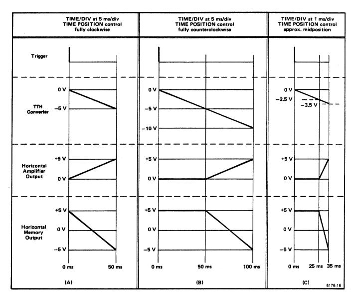
Figure 3-6. Effect of TIME POSITION and TIME/DIV controls. SWEEP RANGE set at 5 ms/div to 10 µs/div position.
