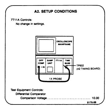
a. Set the Differential Comparator - Input to the Comparison Voltage (Vc).
