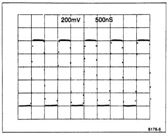
Figure 2-4. Sequential equivalent-time sampling display of 1  $\mu$ s, 1 V square-wave output of pulse generator.
