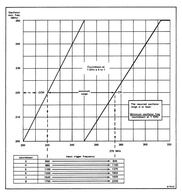
Figure 4-7. Minimum range required for the 200 MHz oscillator.
