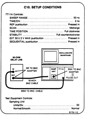
a. Obtain a free-running sweep by setting 7T11A STA-BILITY full clockwise and TRIG LEVEL to approximately midrange.
