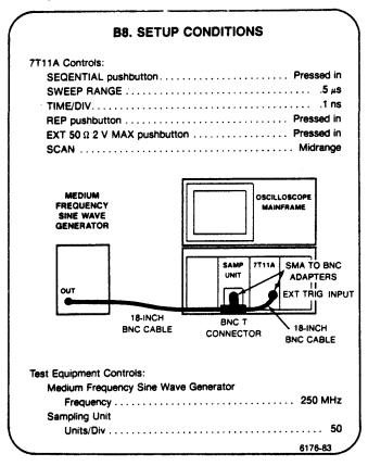
a. CHECK—the oscilloscope display for jitter using the settings and requirements given in Table 5-7(A). Carefully adjust 7T11A STABILITY and TRIG LEVEL for minimum jitter before a measurement is made. Press the 7T11A REP pushbutton in when checking Sequential mode operation and the MAN pushbutton in when checking Random mode.
