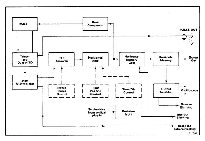
Figure 3-2. 7T11A complete block diagram for Real-time sampling.
