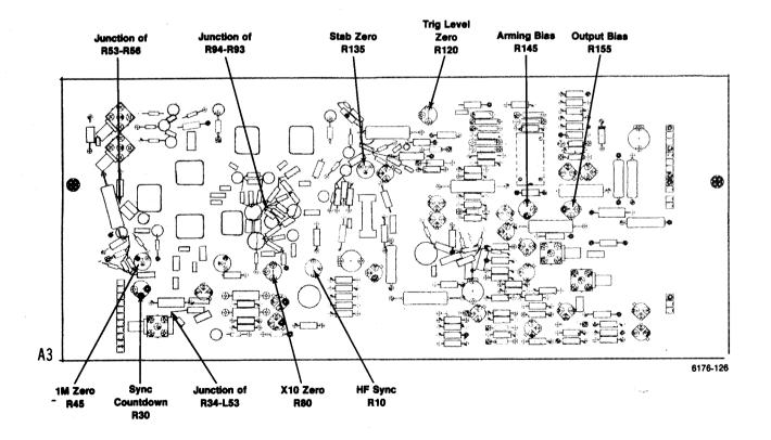
Figure 8-9. Location of Trigger adjustments.
