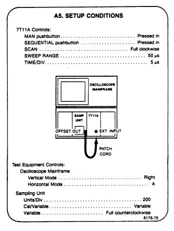
a. CHECK—for a dot on the display, positioned near the right graticule edge.
