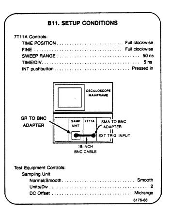
a. Install a Sampling Head having less than 2 mV of display noise in the Sampling Unit. Connect the Sampling Head input to the 7T11A EXT TRIG INPUT.
