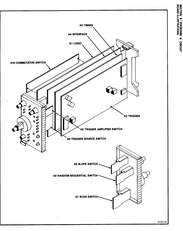
Figure 8-2. Location of circuit boards in the 7T11A.
