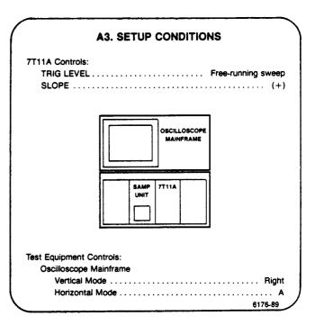
a. Set 7T11A STABILITY as far counterclockwise as possible while still maintaining a free-running sweep. Note the position of the TRIG LEVEL control.
