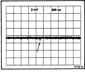
Figure 5-15. Typical display of trigger kickout.
