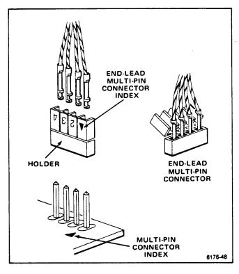
Figure 4-3. Orientation of multi-pin connectors.
