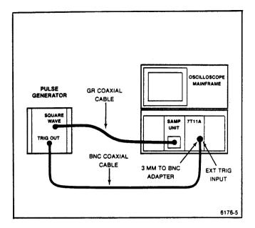
Figure 2-3. Equipment setup for Operators Checkout Procedure.
