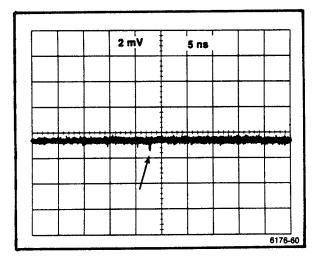
Figure 5-5. Typical display of trigger kickout.
