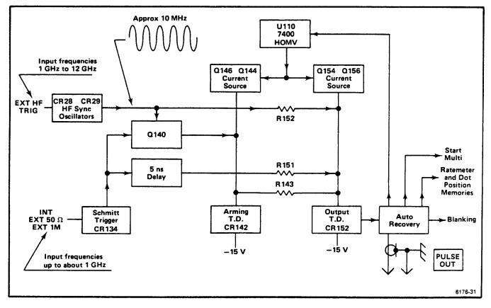
Figure 3-21. Relationship of the Output Tunnel Diode to other 7T11A circuits.
