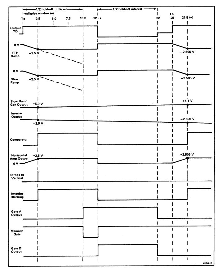
Figure 3-9. Ideal waveform relationships during sequential equivalent-time sampling.
