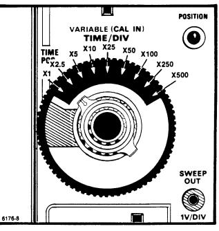
Figure 2-6. Position of selected TIME/DIV setting within control window and corresponding magnification rate.
