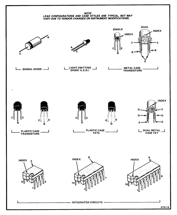
Figure 8-1. Semiconductor lead configurations.
