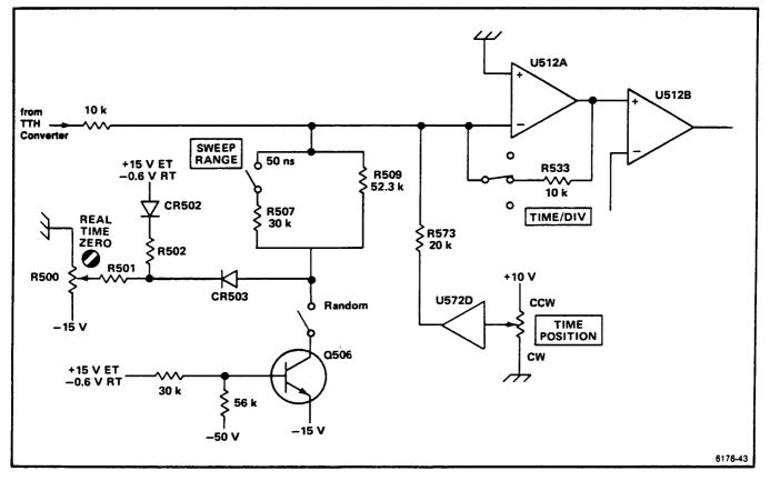
Figure 3-33. Simplified diagram showing sources of Horizontal Amplifier offset current.
