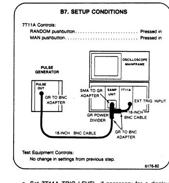
a. Set 7T11A TRIG LEVEL, if necessary for a display such as that shown in Figure 5-3A.
