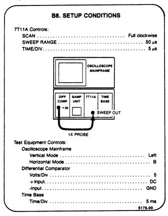
a. CHECK-the display for 25 ms or less per sawtooth (see Figure 5-11).
