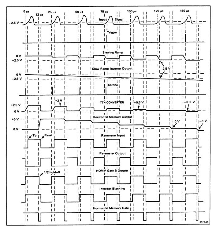
Figure 3-15. Ideal waveform relationships during Random equivalent-time sampling.
