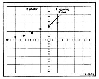
Figure 3-16. Display of samples taken in Figure 3-15.
