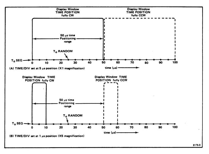
Figure 2-7. Effect of TIME POSITION control (SWEEP RANGE at 5 µs/div to 10 ns/div position).
