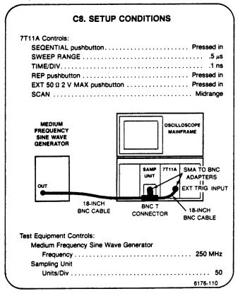
a. Set 7T11A TRIG LEVEL and STABILITY, Sampling Unit Offset, and signal generator Amplitude for an 8-division sine wave display.
