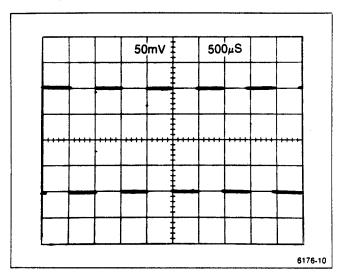
Figure 2-8. Real-time sampling display of the 0.2 V, 1 kHz output of a 7000-series oscilloscope calibrator.
