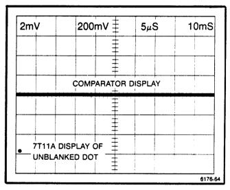
Figure 5-9. Typical display for adjusting Dot Position Memory (A1R645) and Servo Zero (A1R588).
