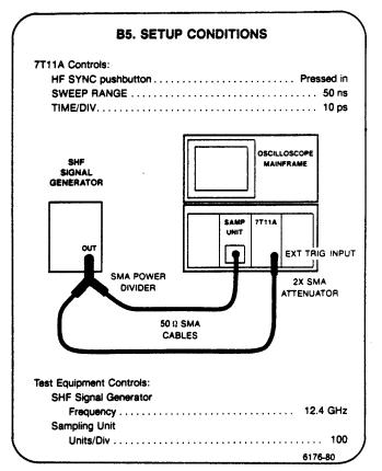
a. CHECK—that a stable, triggered waveform providing 200 mV of trigger signal to the 7T11A can be obtained on the oscilloscope with the 7T11A STABILITY and TRIG LEVEL controls along with the signal generator Amplitude control.
