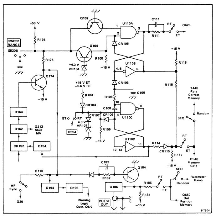
Figure 3-24. Outputs of the HOMV and associated circuits.
