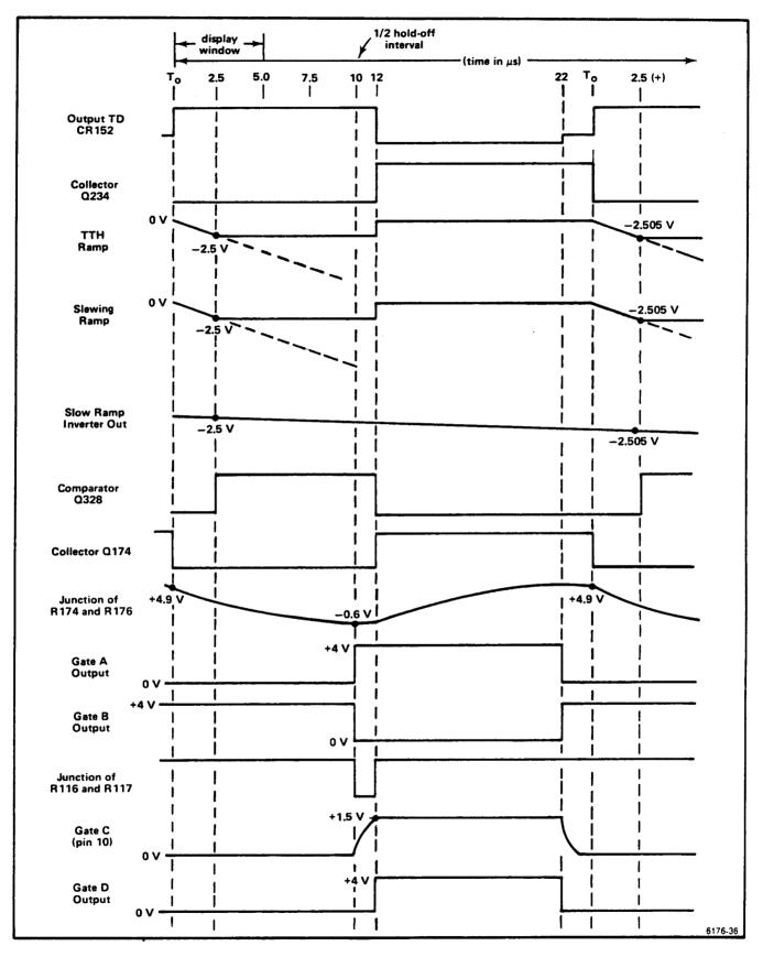
Figure 3-26. Typical waveform relationships during sequential equivalent-time sampling.
