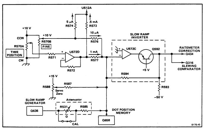
Figure 3-35. Inputs and outputs of the Slow Ramp Inverter.
