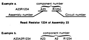
Read: Resistor 1234 of Subassembly 2 of Assembly 23
