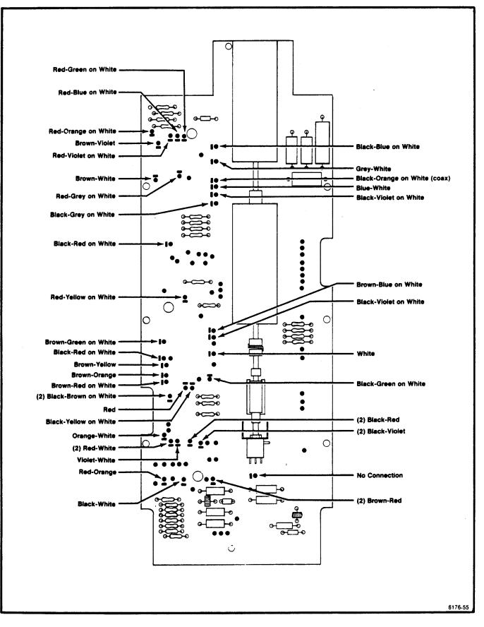
Figure 4-9. Connections to Interface assembly A4.
