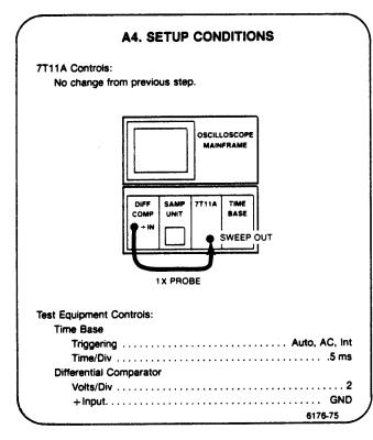
a. Use the Differential Comparator Position control to center the displayed sweep.
