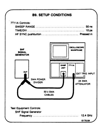
a. Set the signal generator Amplitude and Sampling Unit Units/Div controls to provide at least 200 mV of trigger signal to the 7T11A and display a steep enough waveform slope to accurately measure jitter.
