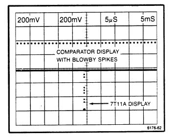
Figure 5-7. Typical display of Memory Gate blowby.
