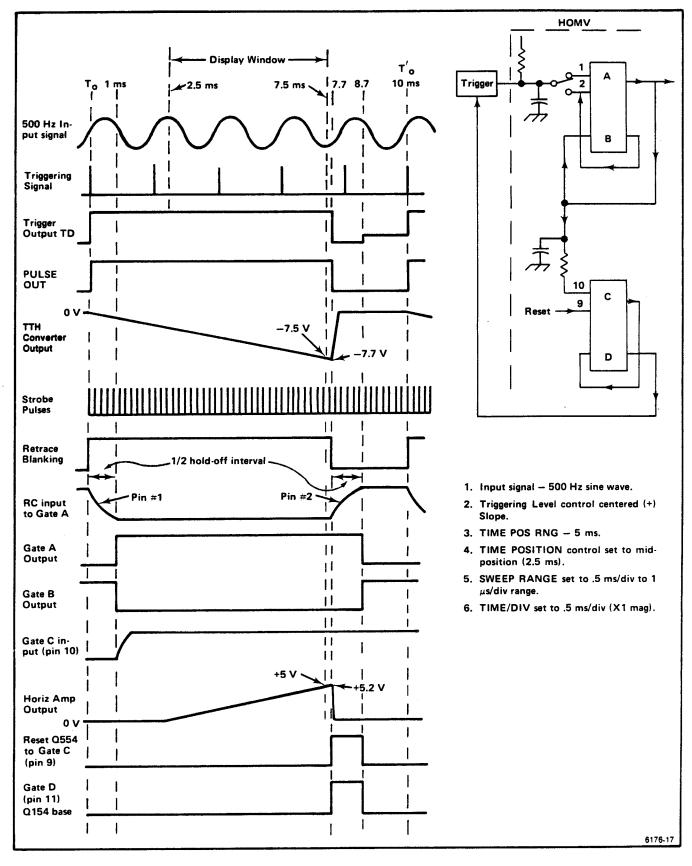
Figure 3-7. Ideal Trigger, Sweep, and HOMV waveform relationships during real-time sampling.
