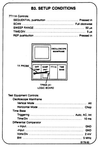
a. Set 7T11A TRIG LEVEL for a free running 7T11A sweep on the oscilloscope display
