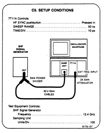
a. **CHECK**—that a stable, triggered waveform providing 200 mV of trigger signal to the 7T11A can be obtained on the oscilloscope display by using the 7T11A STABILITY and TRIG LEVEL controls along with the signal generator Amplitude control.
