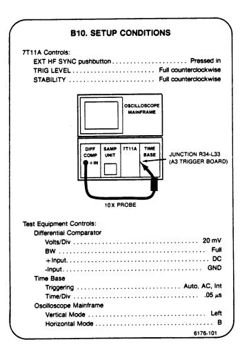
a. Set the Differential Comparator Position control and Time Base Position and Triggering controls for a stable display as shown in Figure 5-12A.
