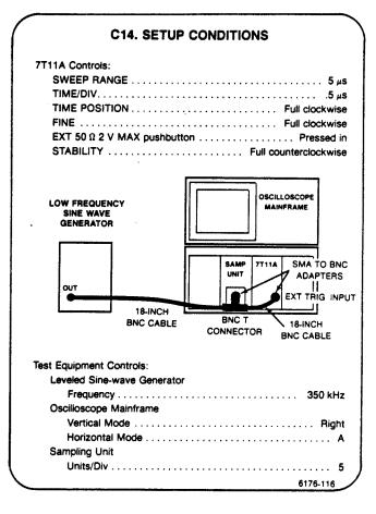
a. Set the Sine Wave Generator amplitude and 7T11A TRIG LEVEL for a stable display with 5 divisions of amplitude.
