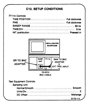
a. Install a Sampling Head having less than 2 mV of display noise in the Sampling Unit. Connect the Sampling Head input to the 7T11A EXT TRIG INPUT.
