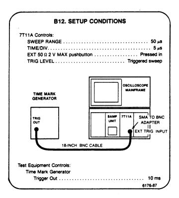
a. Set 7T11A TRIG LEVEL for a triggered sweep.
