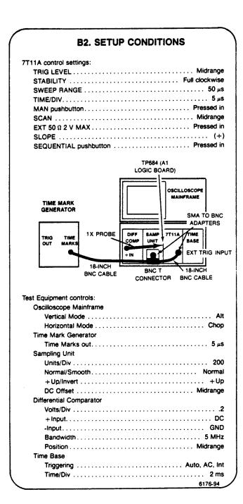
a. Set 7T11A SCAN to center the Differential Comparator trace on the oscilloscope display.
