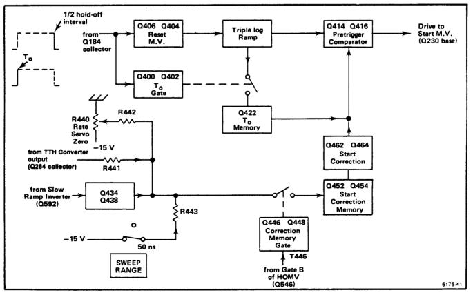
Figure 3-31. Simplified block diagram of Ratemeter circuit.
