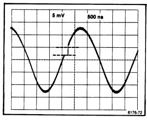
Figure 5-17. Typical display of strobe kickback.
