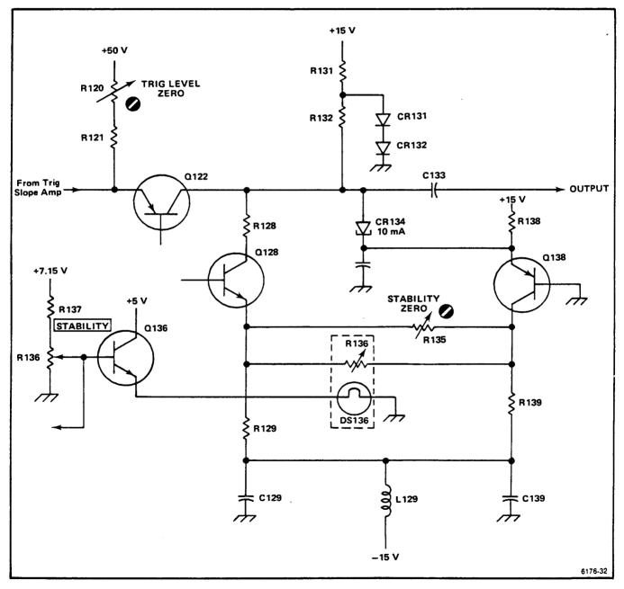
Figure 3-22. Simplified schematic of the Schmitt Trigger circuit.
