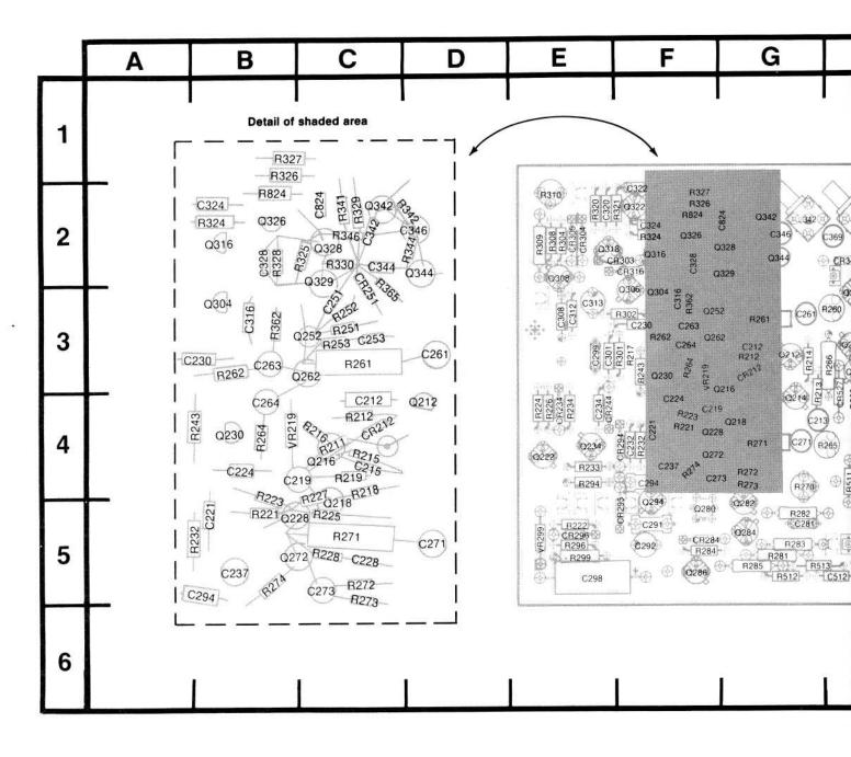
Figure 8-4. A2-Timing circuit boar
