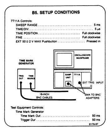
a. Set 7T11A TRIG LEVEL and STABILITY for a free running sweep.
