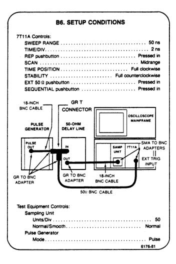
a. Set 7T11A TRIG LEVEL, if necessary for a display such as that shown in Figure 5-3A.
