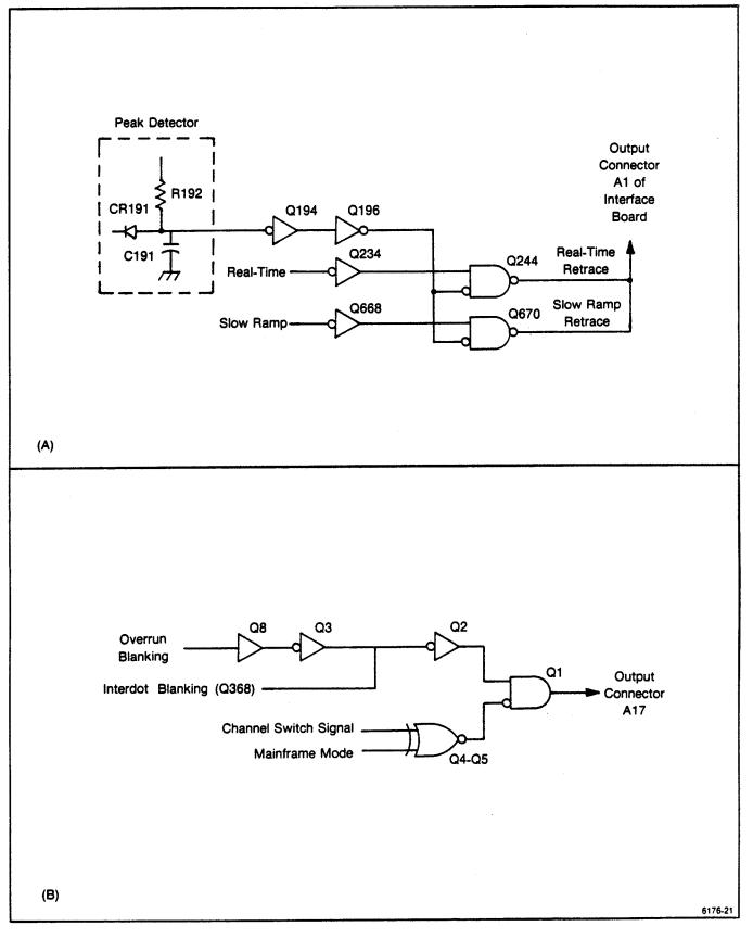
Figure 3-11. 7T11A Blanking Logic.
