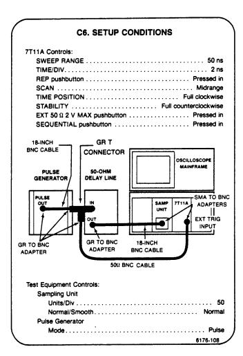
a. Set 7T11A TRIG LEVEL, if necessary, for a display such as that shown in Figure 5-13A.
