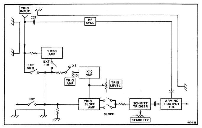
Figure 3-18. Block diagram of the 7T11A trigger circuit.
