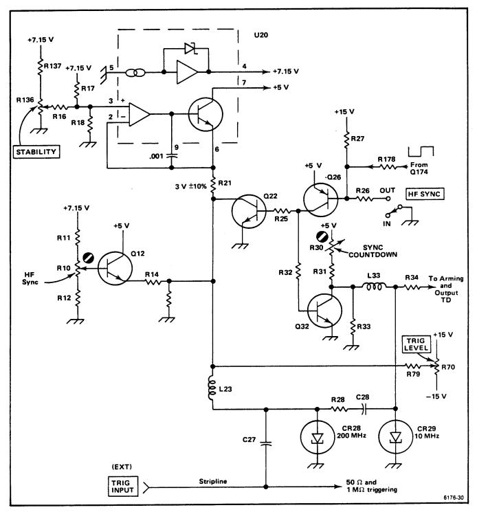
Figure 3-20. Simplified diagram of HF SYNC circuit.
