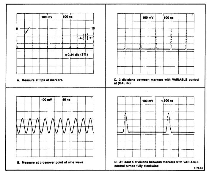
Figure 5-1. Typical displays for checking timing accuracy.
