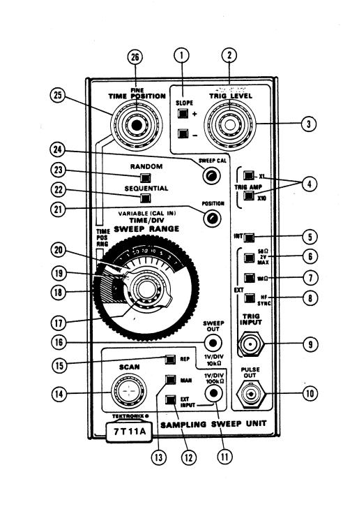
Figure 2-2. Front-panel controls, connectors and indicators.
