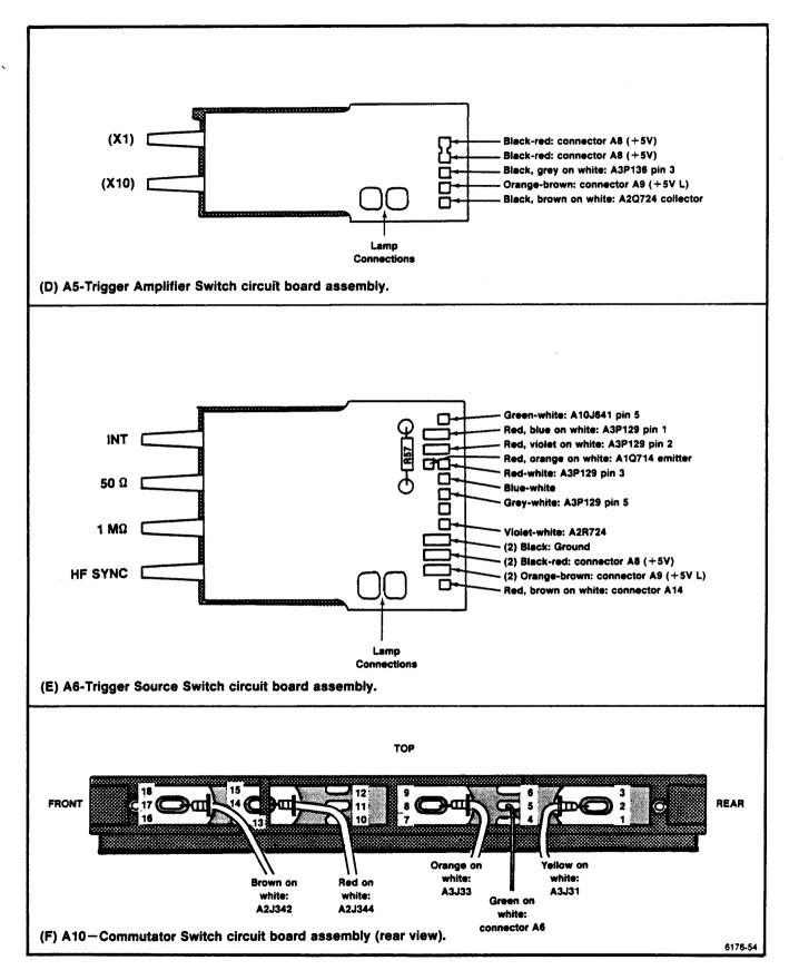
Figure 4-8. Connections to switch assemblies (cont.).
