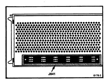
Figure 2-1. Connector J641 (fixed shoe), providing interconnection between 7T11A and 7S11 for strobe and trigger signals.
