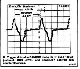
Figure 5-12. Typical display for HF Sync adjustments.
