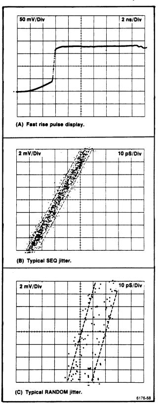
Figure 5-13. Determining display jitter.
