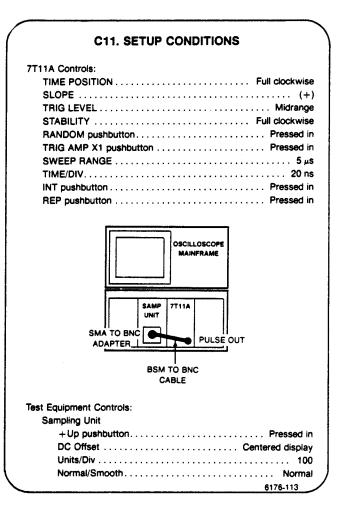
a. Rotate 7T11A TIME POSITION counterclockwise to display the rising portion of the pulse.
