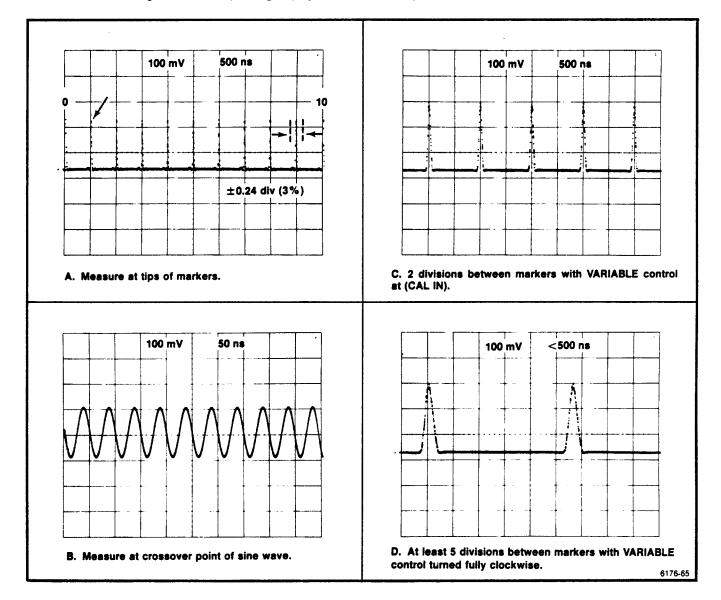
Figure 5-10. Typical displays for checking timing accuracy.
