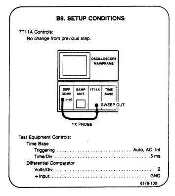
a. Use the Differential Comparator Position control to center the sweep on the display.
