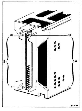
Figure 4-4. Pin numbering on interface connector.
