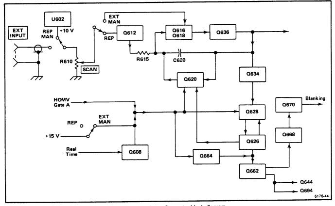
Figure 3-34. Slow Ramp Generator block diagram.
