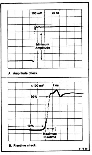
Figure 5-4. Typical display of the Pulse Out waveform.
