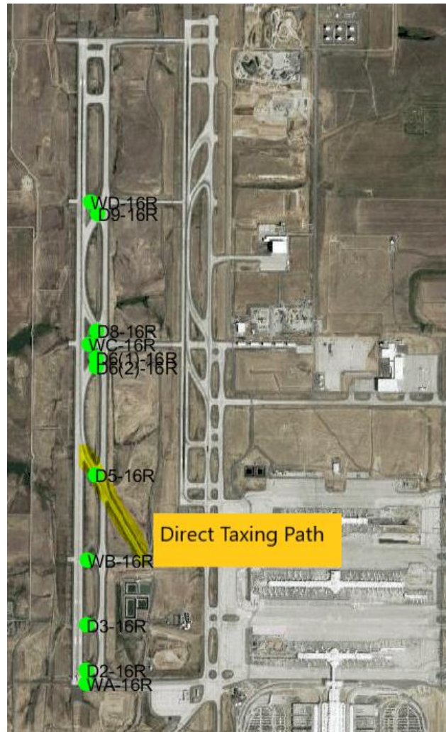
Figure 103. Taxiway D5 on Runway 16R at DEN, Which Leads Airplanes Easily Towards the Terminal Area.
