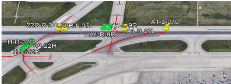
Figure 113. Sample Runway Exit Arcs and Other Information for Identifying Runway Exits.
