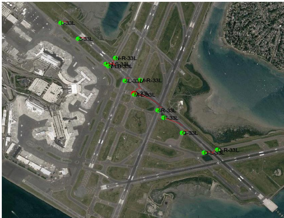
Figure 70. BOS Runway 33L Exit Configuration with Taxiway Q Shown as Closed.
