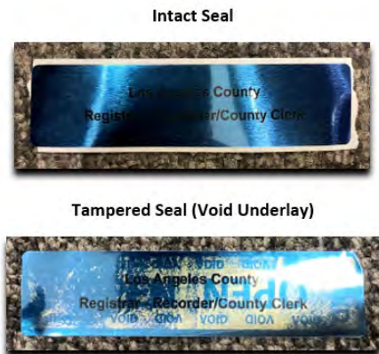
Tamper-evident seal placed over the seam of the Integrated Ballot Box
