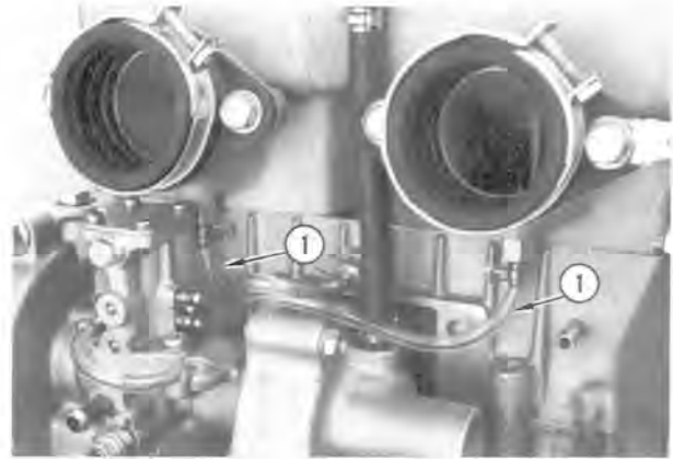
1. Oil Injection Tubes.
