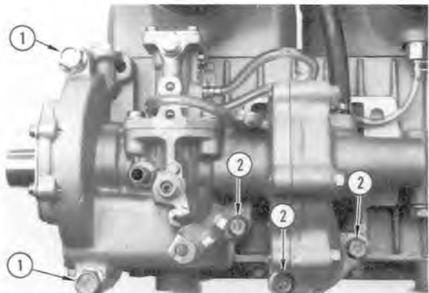
1. Torque to 144 in. lb (1.7 kg-m). 2. Torque to 60 in. lb (0.7 kg-m).
