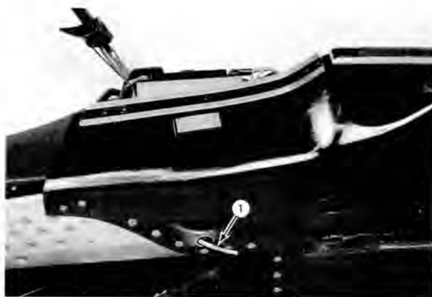
1. Battery Vent Tube
