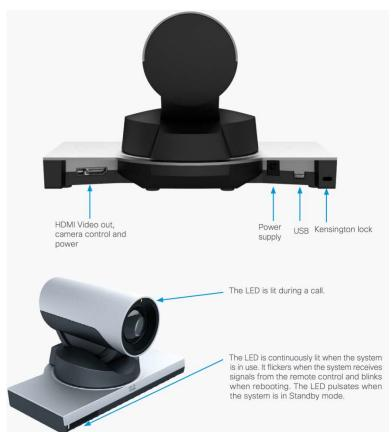
Description: The PrecisionHD 4x camera has had several different revisions. The latest model – the 4XS2 – ships with the SX20 and SX80, and is also integrated into the MX300 G2. The 4XS2 supports 4x
