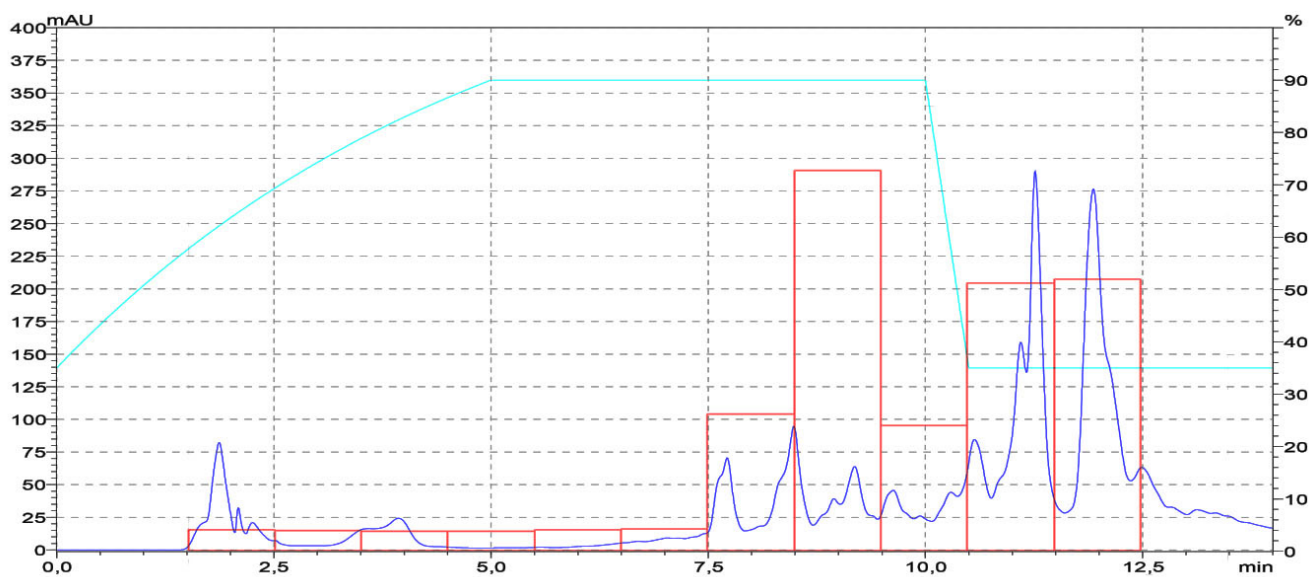
Fig. 5. HPLC separation of P. natans extract: chromatogram (UV 430 nm, blue line), luminescence of fractions (red line) and mobile phase composition (light blue line). All other conditions see Tables 2 and 3
