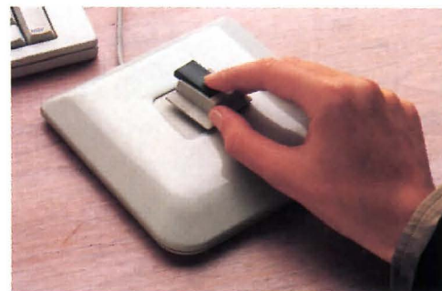
Felix (above) combines a handle like a joystick, a fixed position like a trackball, and an absolute mode like a digitizer.
