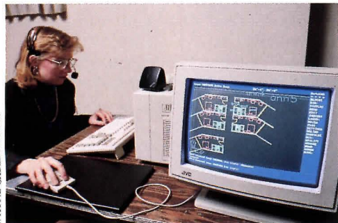
Mary S. Maudlin, AIA, enters Autocad commands by voice with the Bug by Command Corporation (above). With the headset, commands can be issued softly to avoid disruption.
