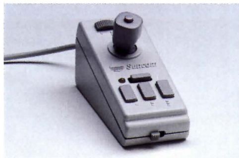
The tiny Icontroller (above) is a cross between a mouse and a joystick. It works well in tight spaces, but the handle takes practice.
