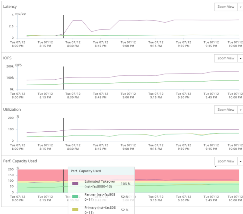
Figure 31) OnCommand Unified Manager failover planning graphs showing both nodes' performance capacity and estimated takeover performance capacity.
