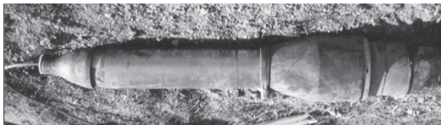
Figure 2 The Bursting Head of the Pneumatic System
