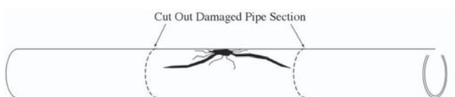
Figure 9 Cut out Damaged Section of Pipe
