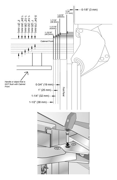
When installing hinge side next to an appliance or object that is within range of the door panel, limit the door opening angle to 90<sup>0</sup>. This is done by installing the banking pin as illustrated. Insert the banking pin through the holes and drive in with a hammer.
