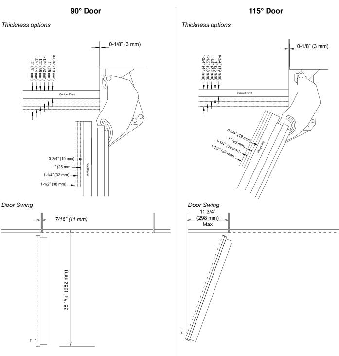
**NOTE**: Additional space needed depending on thickness of front panels and handle used
