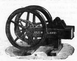
The office of this Machine is to break Ores and Minerals of every kind into small fragments, preparatory to their further comminution by other machinery. Also to break stone for McAdam roads, and Ballasting Railroads.
