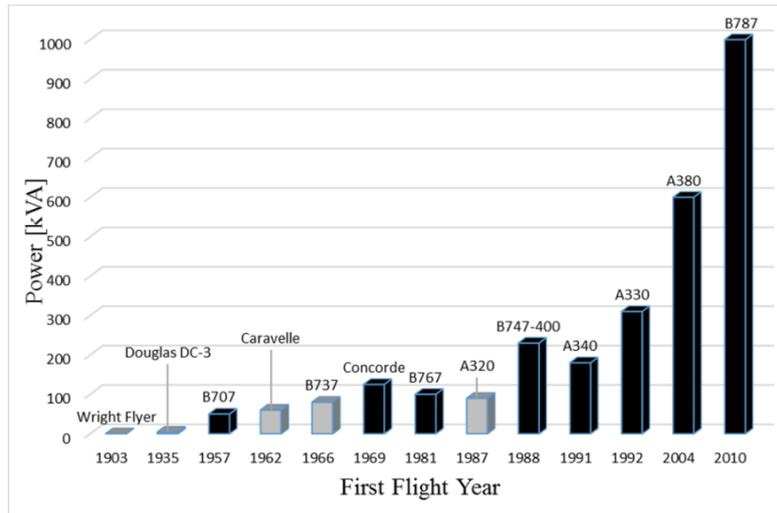
Figure 6 – Evolution of the first flights base on aircrafts models and power usage [28]
