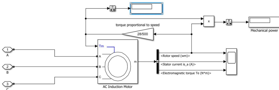
Figure 90 - Under the mask of the AC load: 12 kVA induction motor driving hydraulic pump
