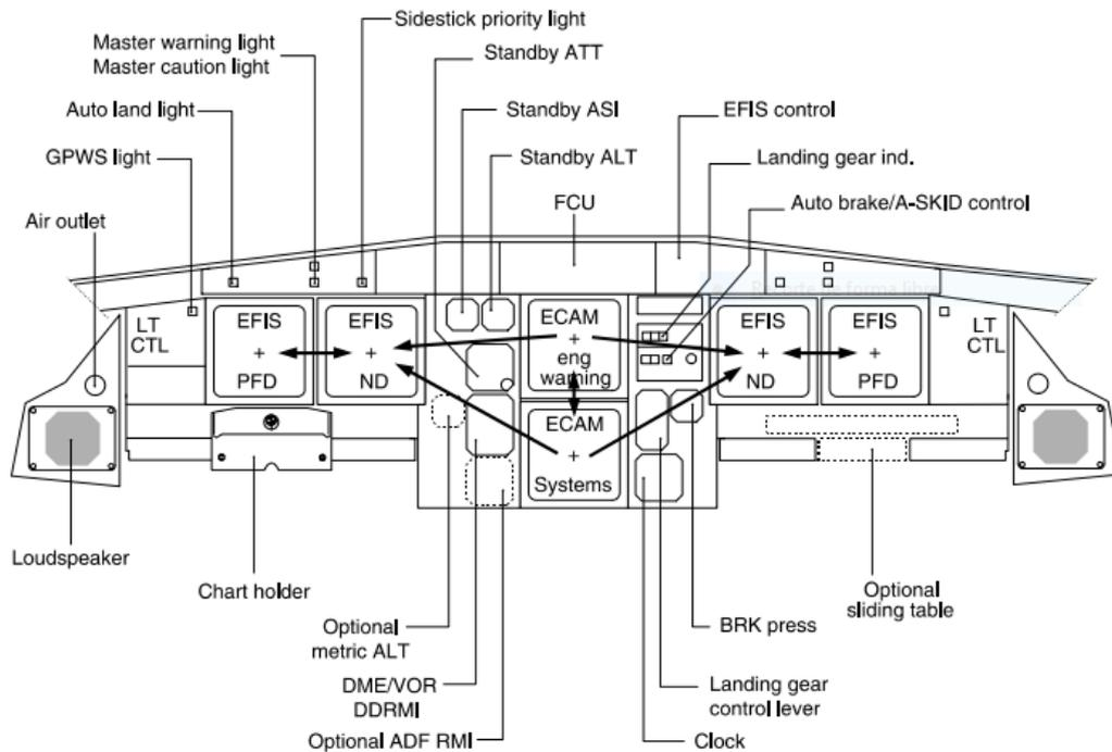
Figure 33 - Main instruments panels of an Airbus A320 [39]
