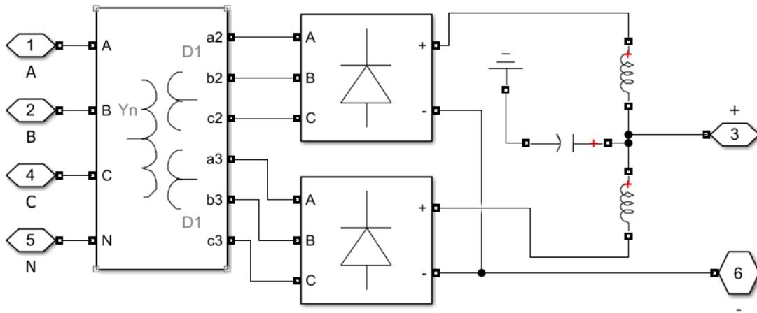
Figure 138 - Under the mask of the TRU block in MATLAB
