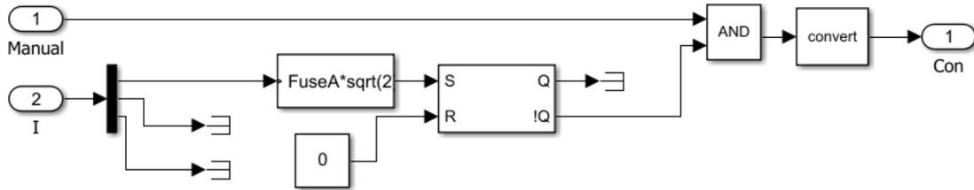
Figure 87 - Subsystem of the breaker trip block in MATLAB
