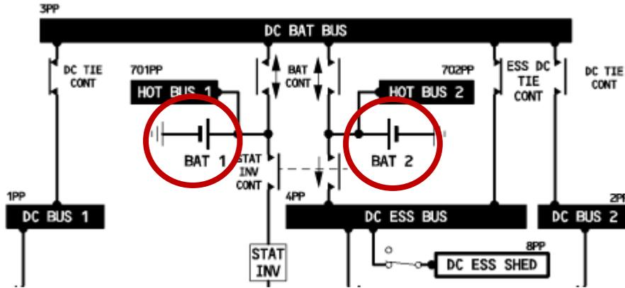
Figure 45 - Generating system of an Airbus A320 (BAT 1 & BAT2) [38]
