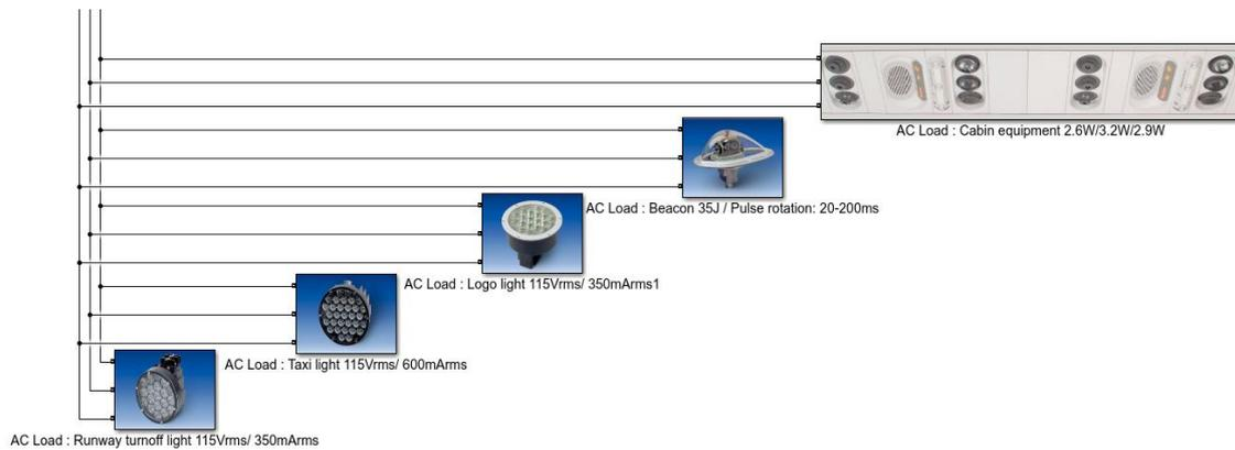
Figure 125 - AC loads: lights in MATLAB
