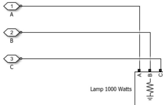
Figure 92 - Under the mask of the AC load: 1 kW lamp
