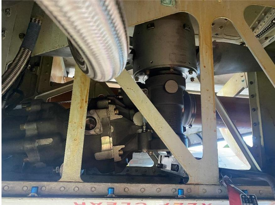
Figure 58 - Inside the RAT of an Airbus A320 (not deployed)
