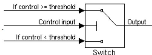
Figure 111 - Switch block in MATLAB
