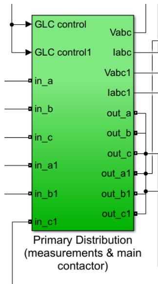
Figure 120 - Primary distribution block in MATLAB
