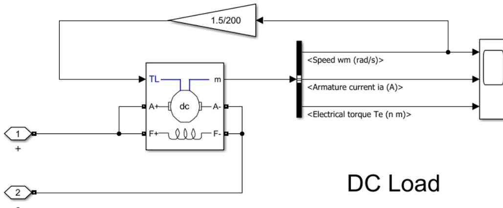
Figure 100 - Under the mask of the DC load: brush motor driving a fuel pump
