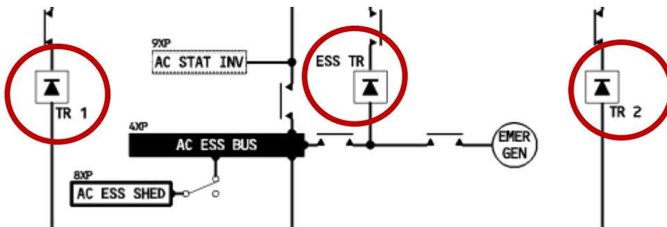
Figure 46 - Generating system of an Airbus A320 (TR1, TR2 & ESS TR) [38]
