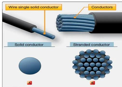
Figure 68 - Wiring types [27]
