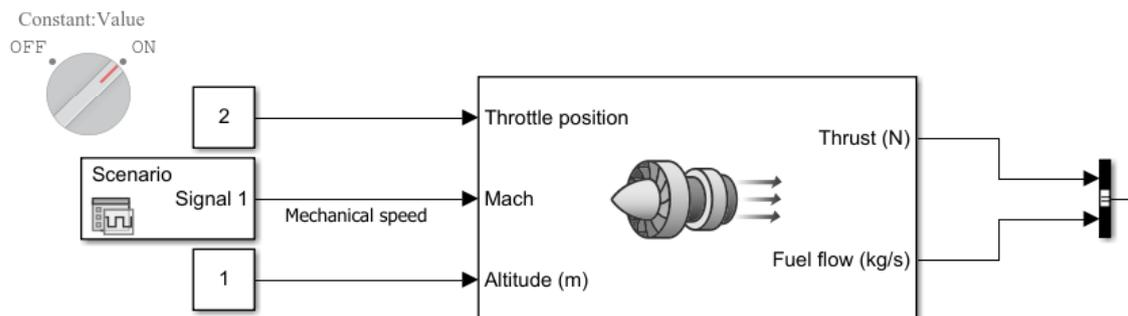
Figure 106 – Mechanical engine block in MATLAB
