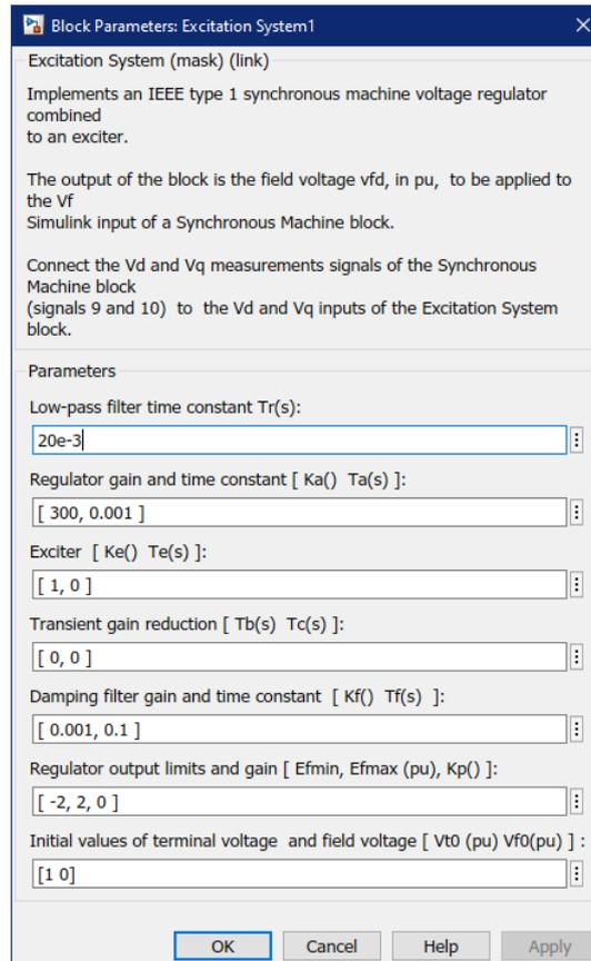
Figure 118 - Excitation system parameters in MATLAB
