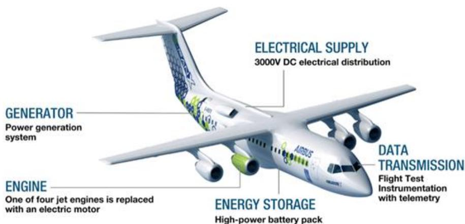
Figure 22 - Airbus electrical aircraft concept [34]
