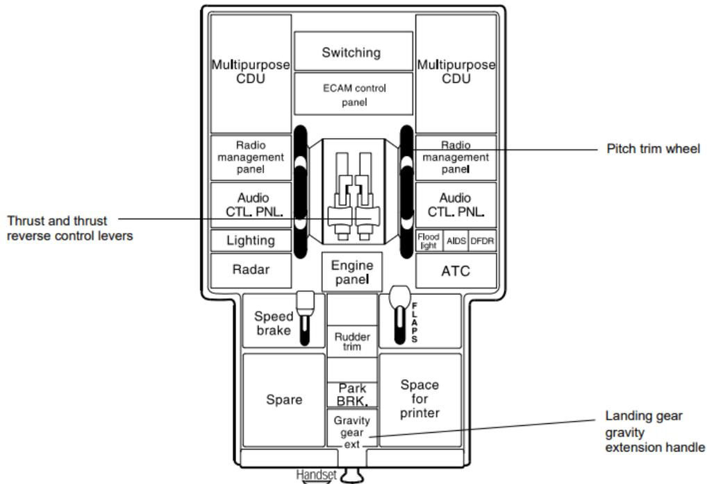
Figure 35 - Pedestal of an Airbus A320 [39]
