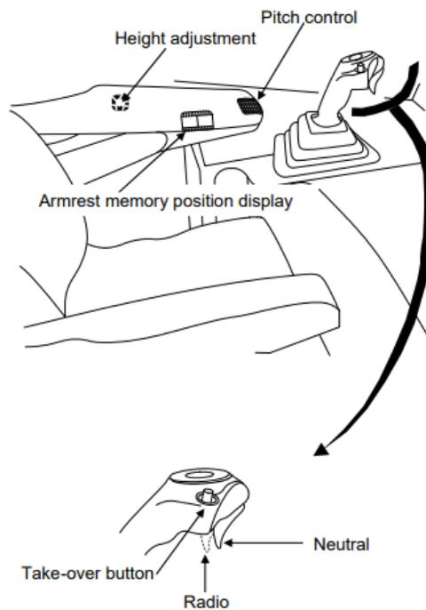
Figure 31 - Sidestick arrangement of an Airbus A320 [39]
