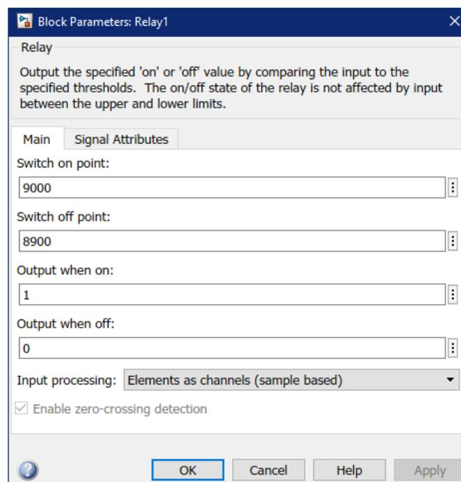
Figure 116 - Relay block values in MATLAB
