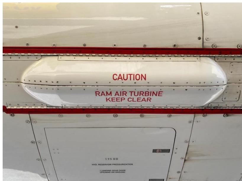
Figure 57 - Ram Air Turbine of an Airbus A320
