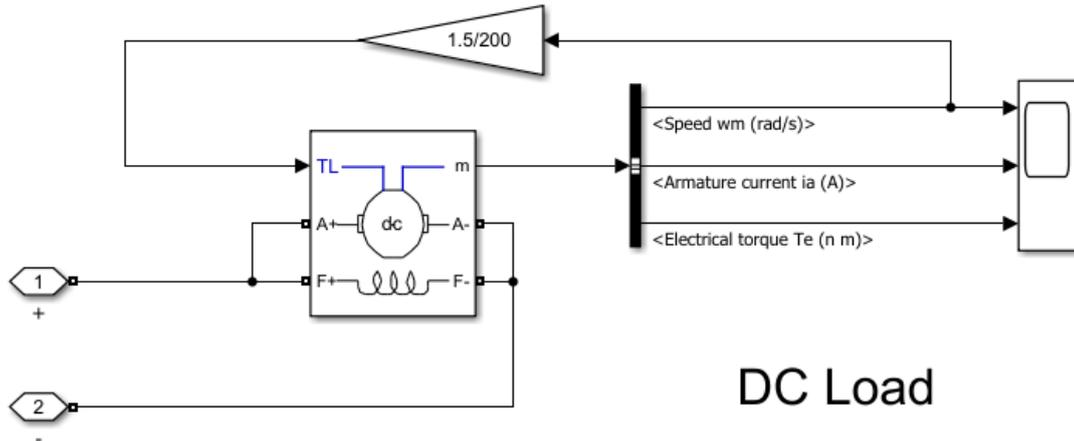
Figure 144 - Under the mask of the brush motor driving a fuel pump block in MATLAB
