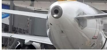
Figure 48 – APU (exterior) from an Airbus A320
