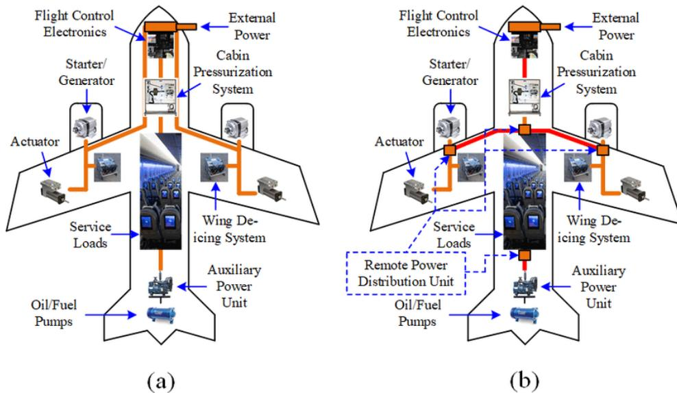
Figure 76 - Typical electrical power flow schematic
