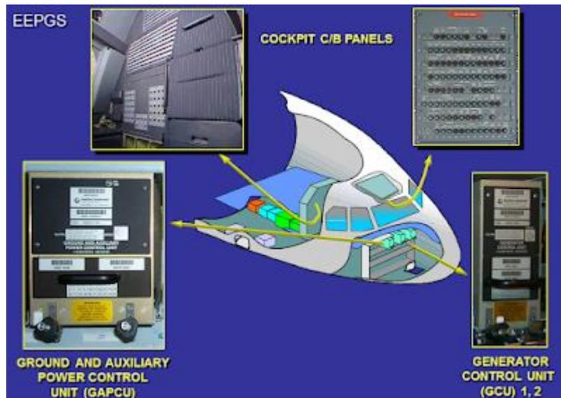
Figure 62 - Airbus A320 generation system distribution of the EEPGS [40]
