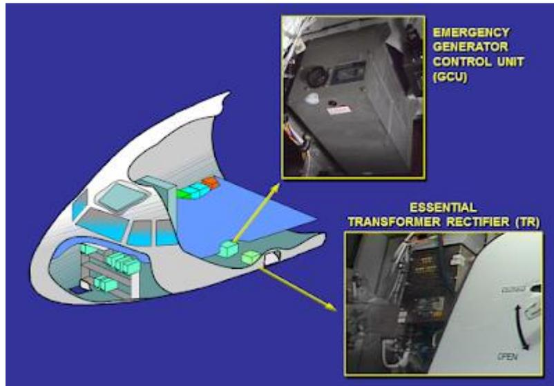
Figure 63 - Airbus A320 generation system of the EGPU [40]
