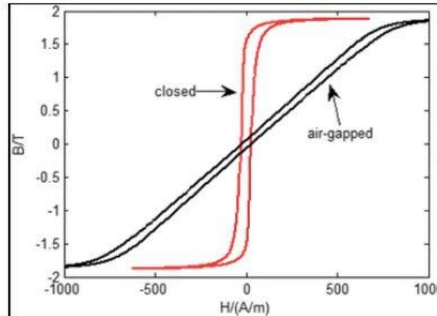
Figure 15 - Air gap curve on magnetics effect [23]
