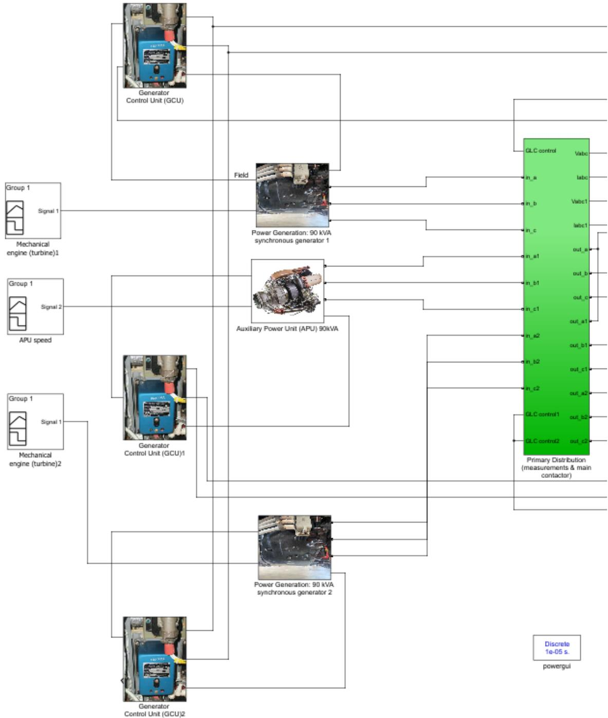
Figure 150 - Airbus A320 final schematic in MATLAB (1/4 parts)
