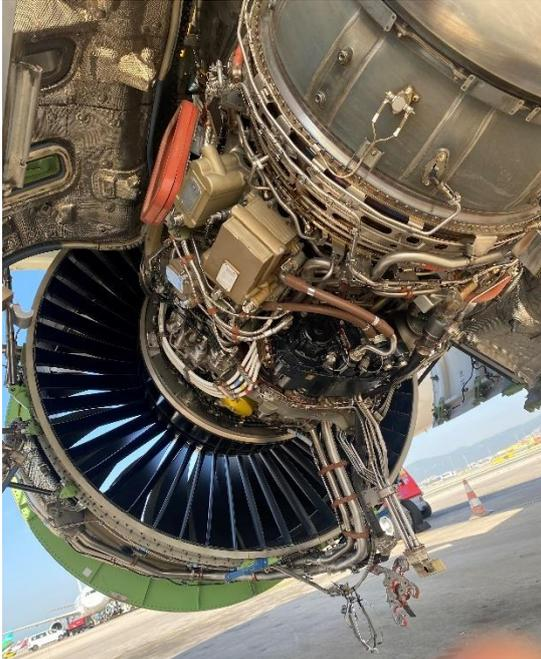
Figure 26 - Inside of the CFM56-5B engine (left side)
