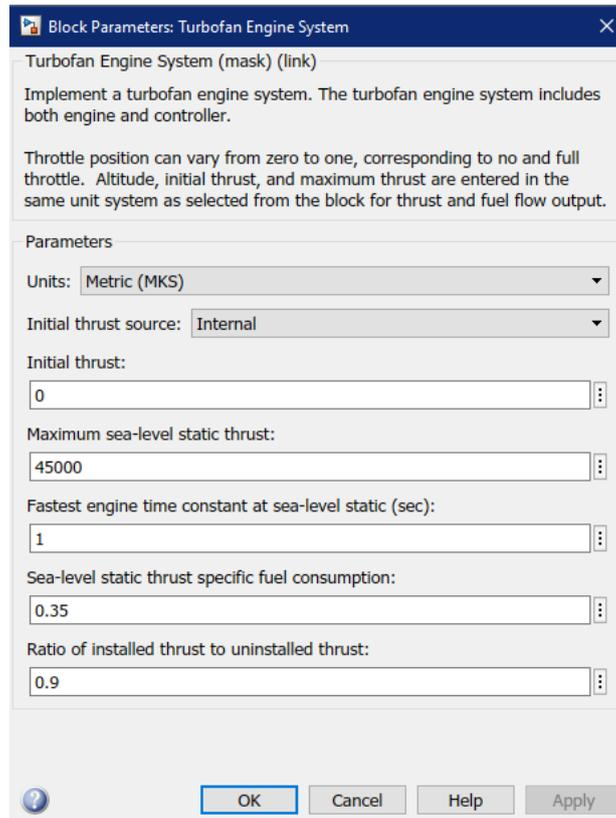
Figure 105 - Turbofan engine system parameters in MATLAB
