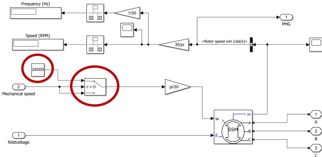
Figure 112 - Under the mask of the APU block in MATLAB
