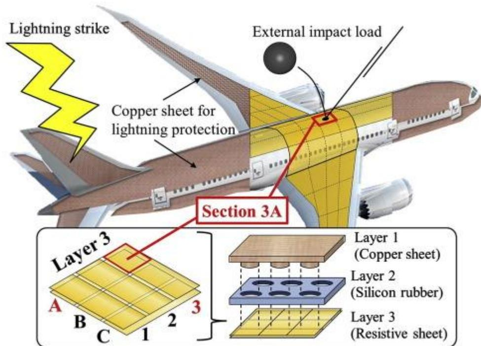
Figure 21 - Aircraft lightning strike sections [33]
