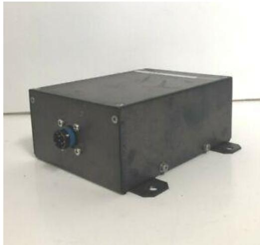
*Figure 18 - A320 static converter [33]*
