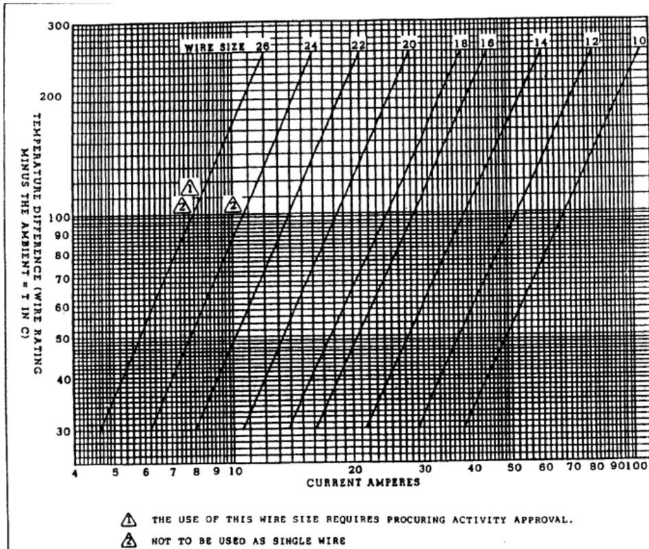
Figure 71 - Single copper wire on free air [3]
