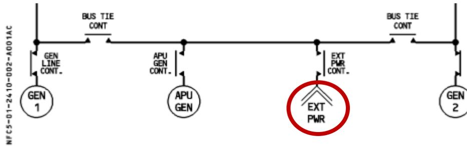
Figure 42 - Generating system of an Airbus A320 (EXT PWR) [38]
