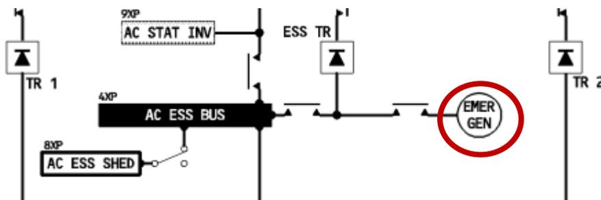
Figure 43 - Generating system of an Airbus A320 (EMER GEN) [38]
