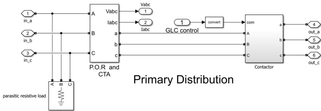
Figure 84 - Under the mask of the primary distribution
