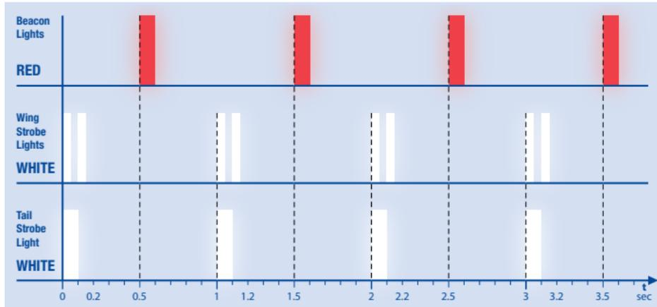
Figure 130 - Flashing sequences and synchronization
