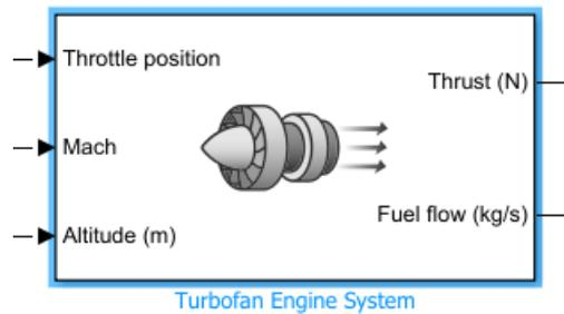
Figure 104 - Turbofan engine system block in MATLAB
