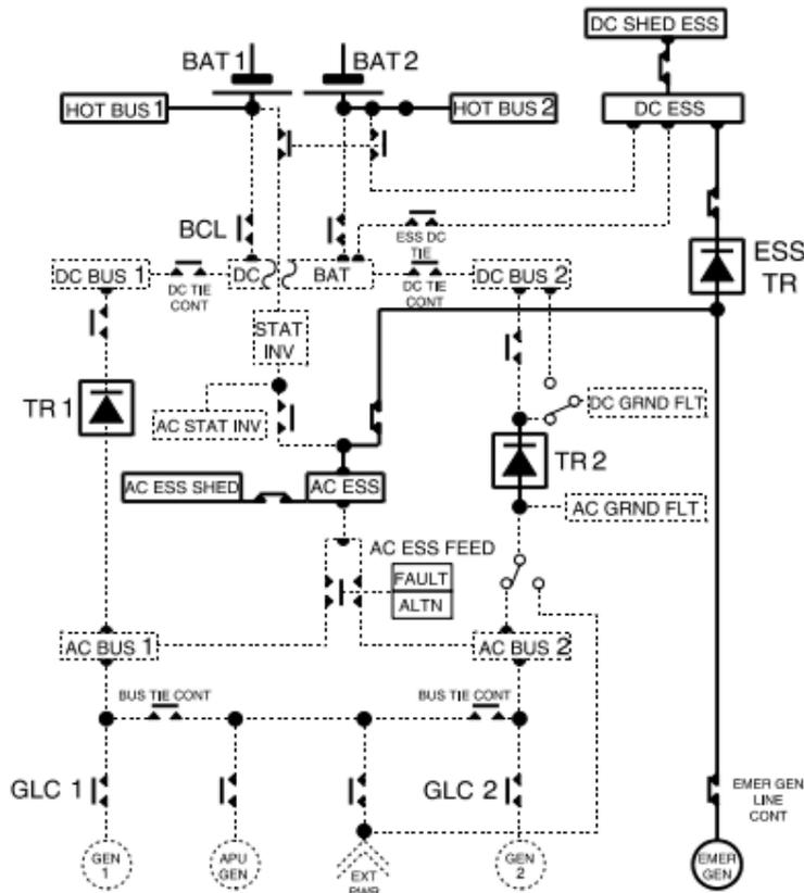
Figure 56 - Loss of main electrical generators scheme [38]
