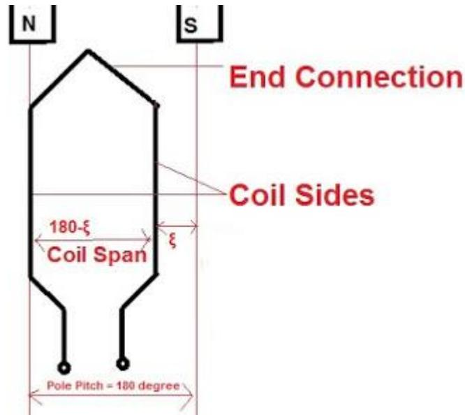
Figure 17 - Coil span factor [22]
