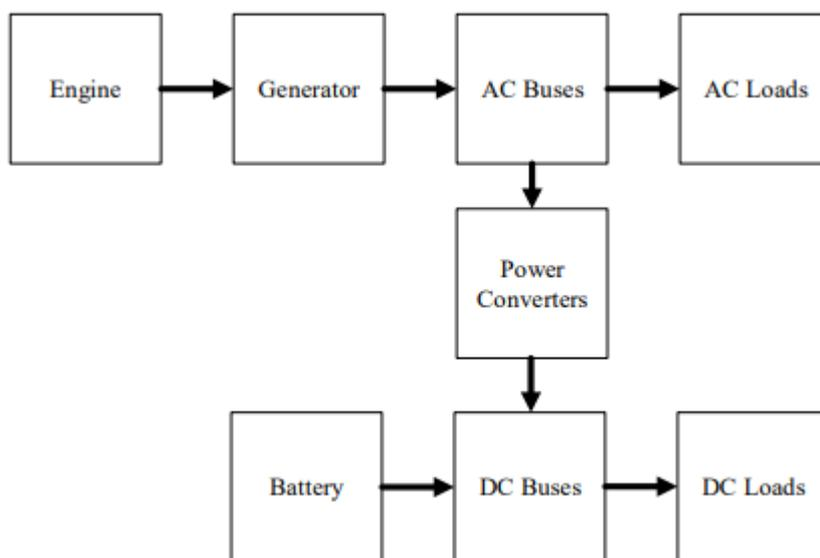
Figure 1- Typical electrical aircraft scheme [1]
