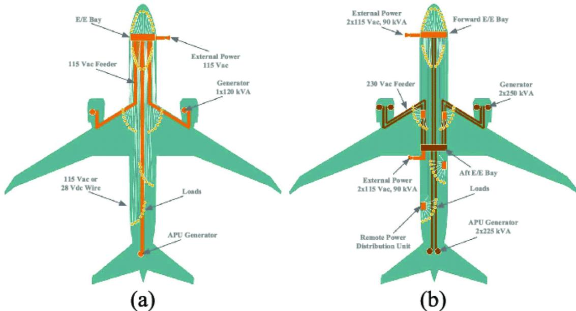
Figure 67 – Two types of distribution of an aircraft [41]
