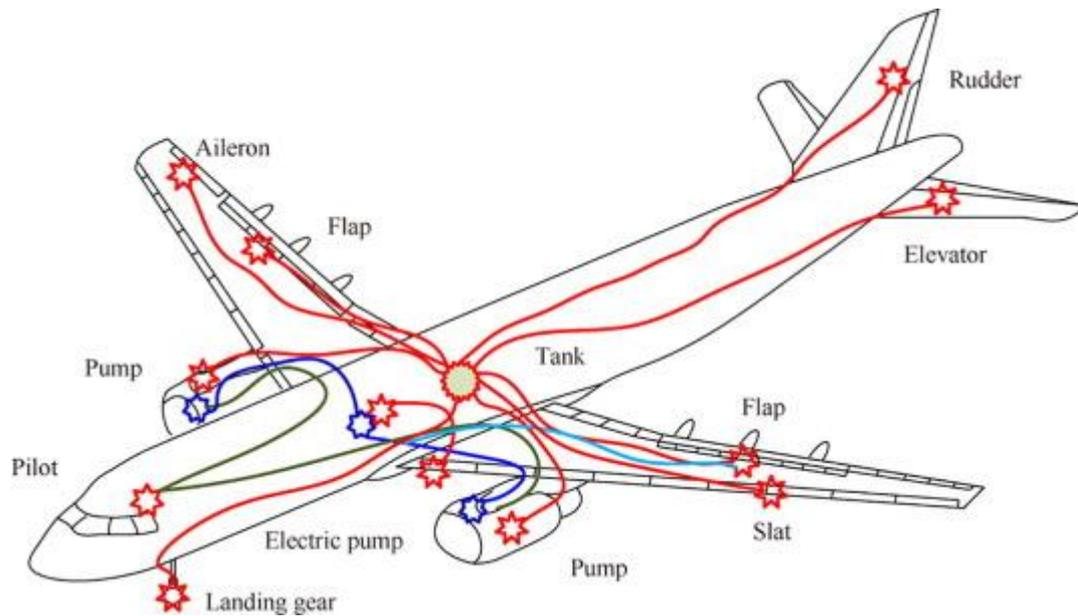
Figure 166 - Hydraulic aircrafts pipeline system [9]
