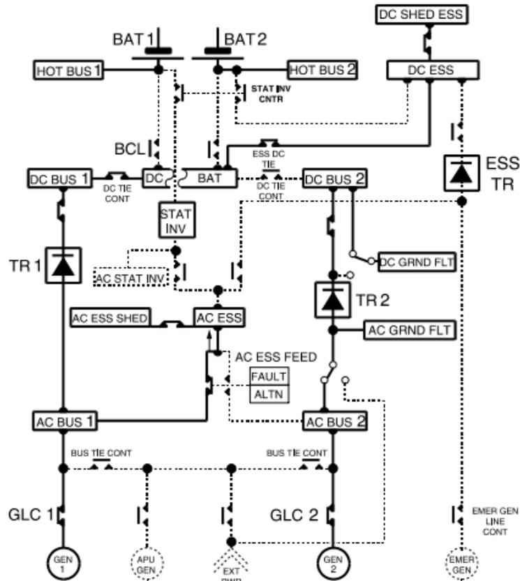
Figure 55 - Normal electrical flight configuration scheme [38]
