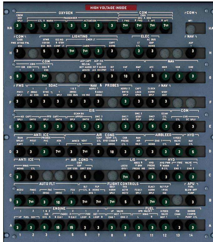
Figure 47 - Circuit breakers from an Airbus A320
