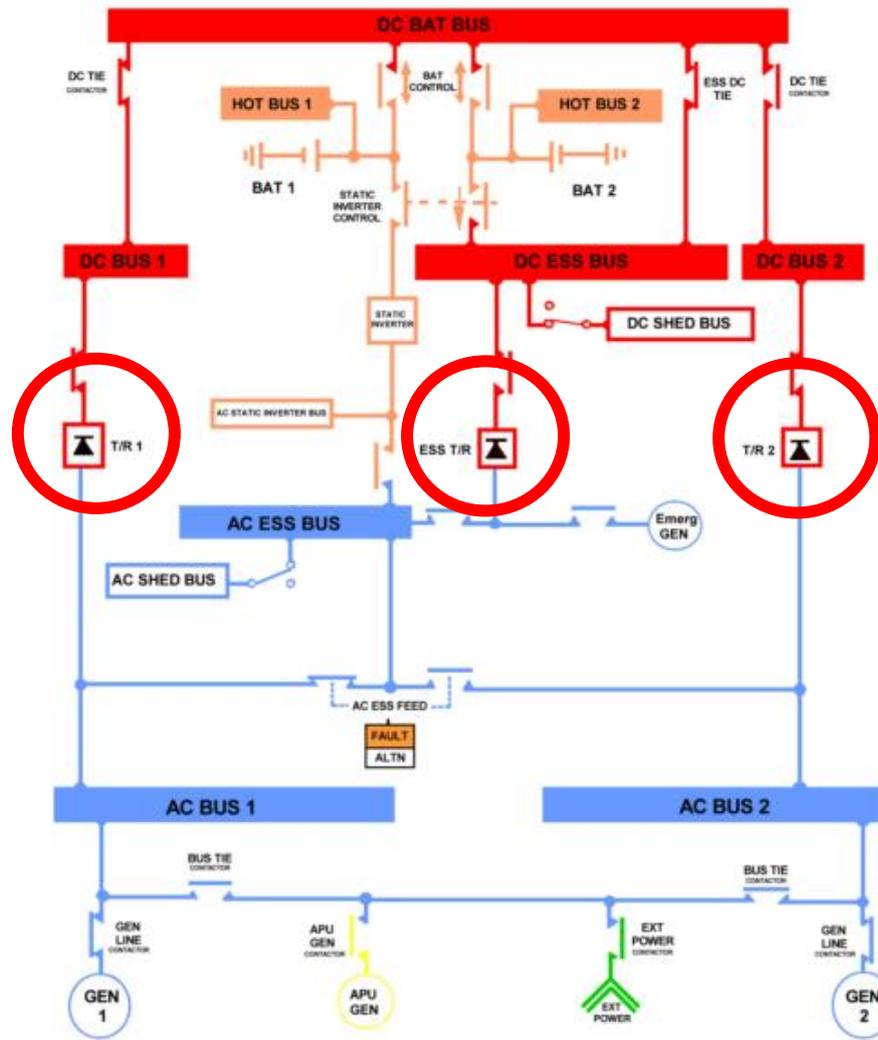
Figure 11 - Energy system detailed on an electrical system schematic [27]
