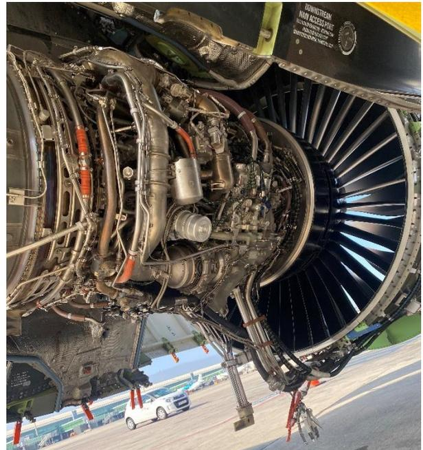
Figure 25 - Inside of the CFM56-5B engine (right side)
