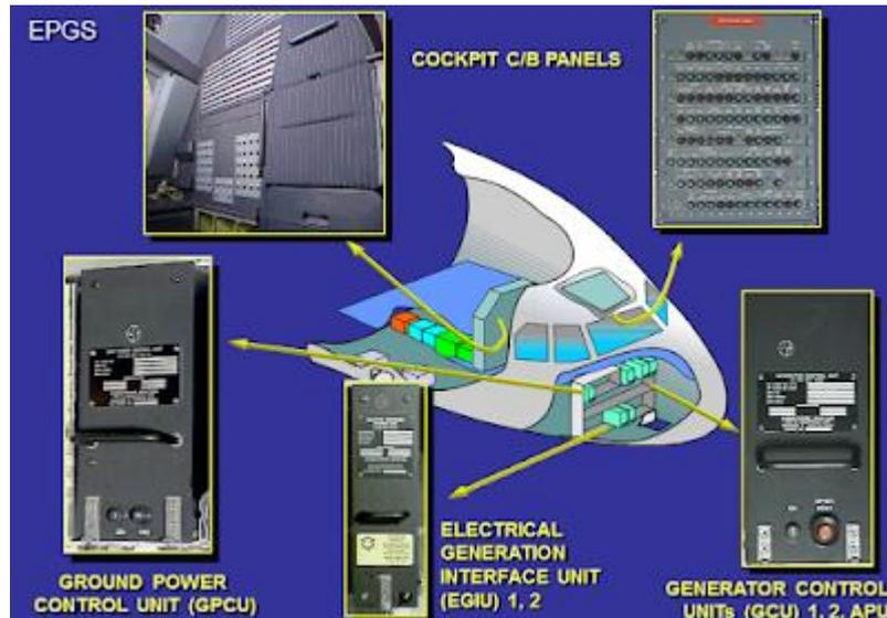
Figure 61 - Airbus A320 generation system distribution EPGS [40]
