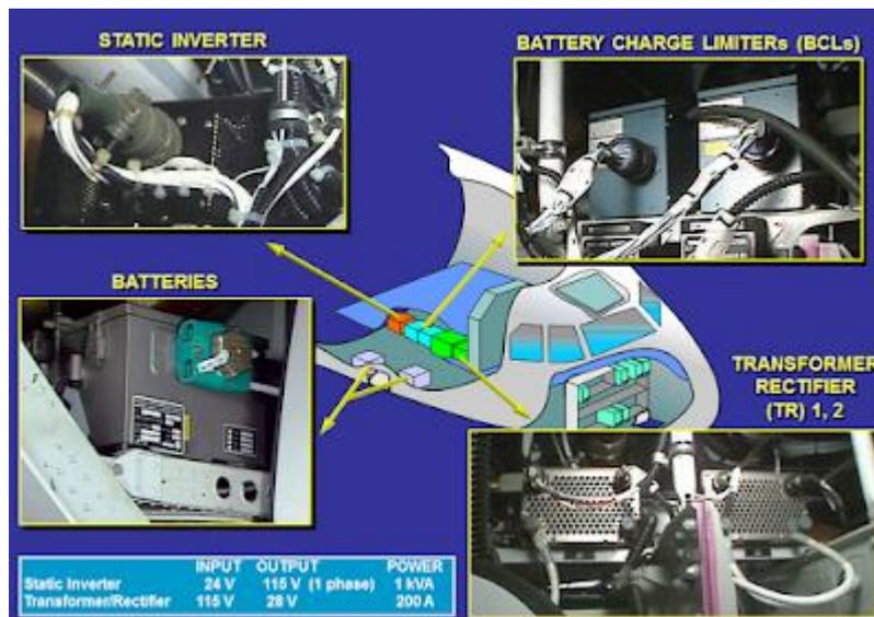
Figure 60 - Airbus A320 generation system distribution next to flightdeck [40]
