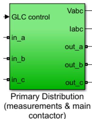
Figure 83 - Primary distribution block in MATLAB
