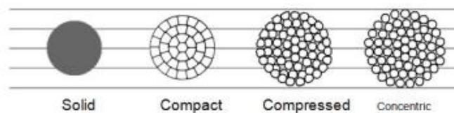
Figure 69 - Types of conductor construction [27]
