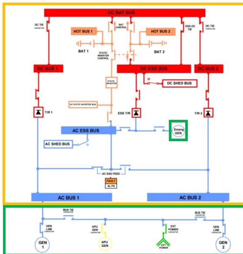
Figure 64 - Electrical system schematic divided in two parts [27]
