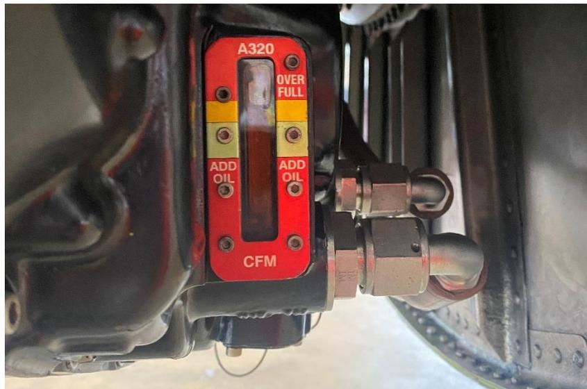
Figure 41 - Oil indicator for the IDG in the Airbus A320
