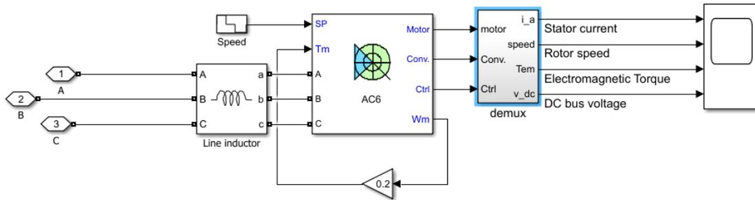
Figure 94 - Under the mask of the AC load: 2kW brushless motor driving a ball screw actuator
