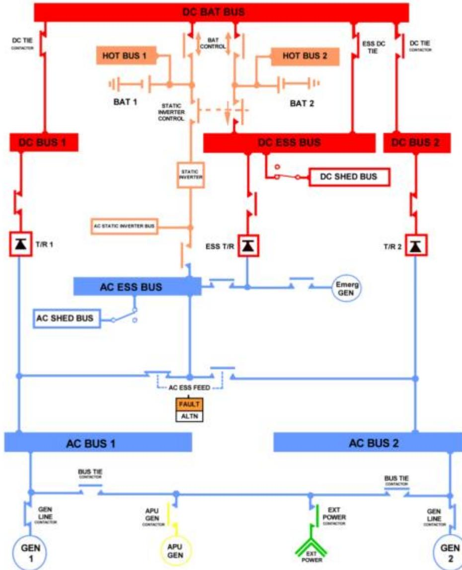
Figure 9 - Electric system schematic [27]
