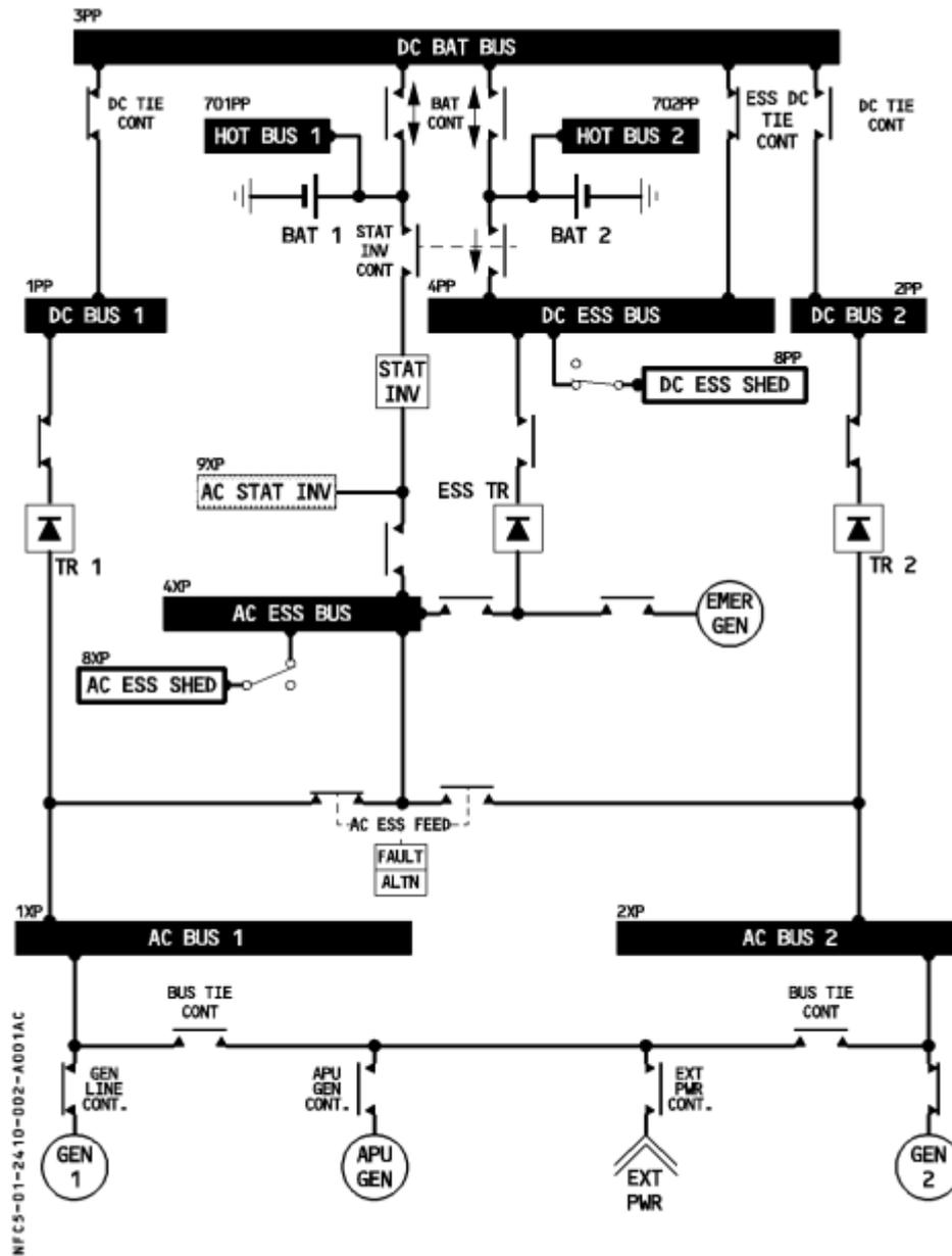
Figure 27 - Airbus A320 electrical system scheme [38]
