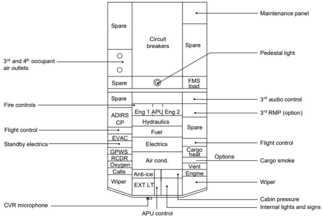
Figure 36 - Overhead panel of an Airbus A320 [39]
