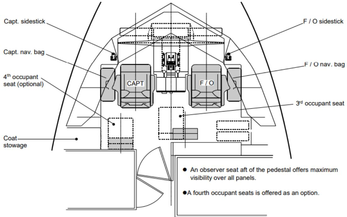
Figure 28 - Flight deck layout Airbus A320 [39]
