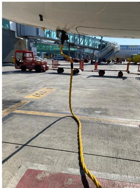
Figure 52 - Cable connection to the aircraft GPU
