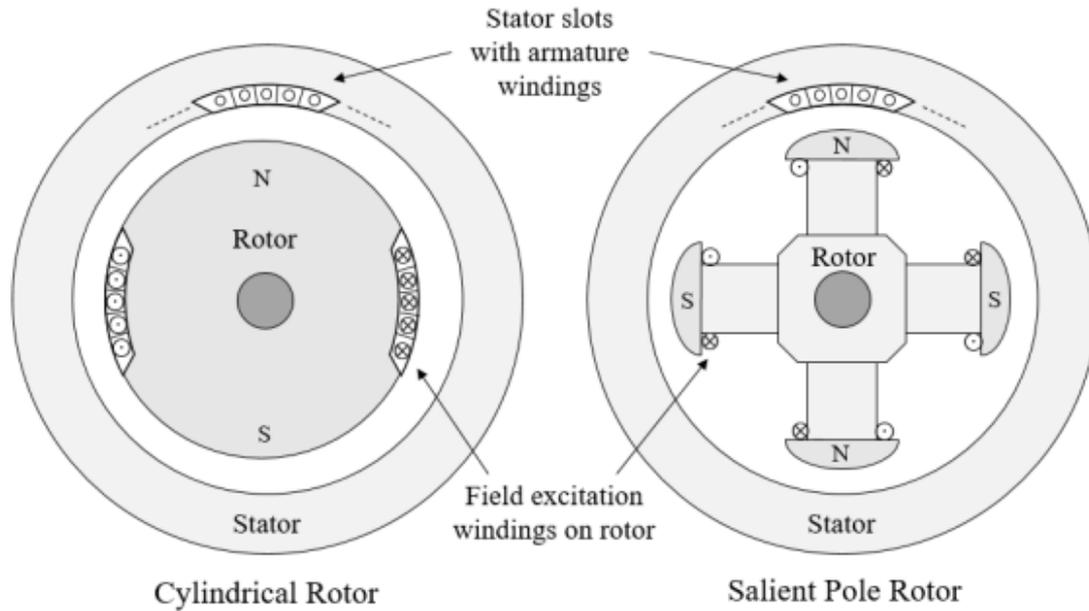
Figure 16 - Comparison between cylindrical and salient pole rotor [32]
