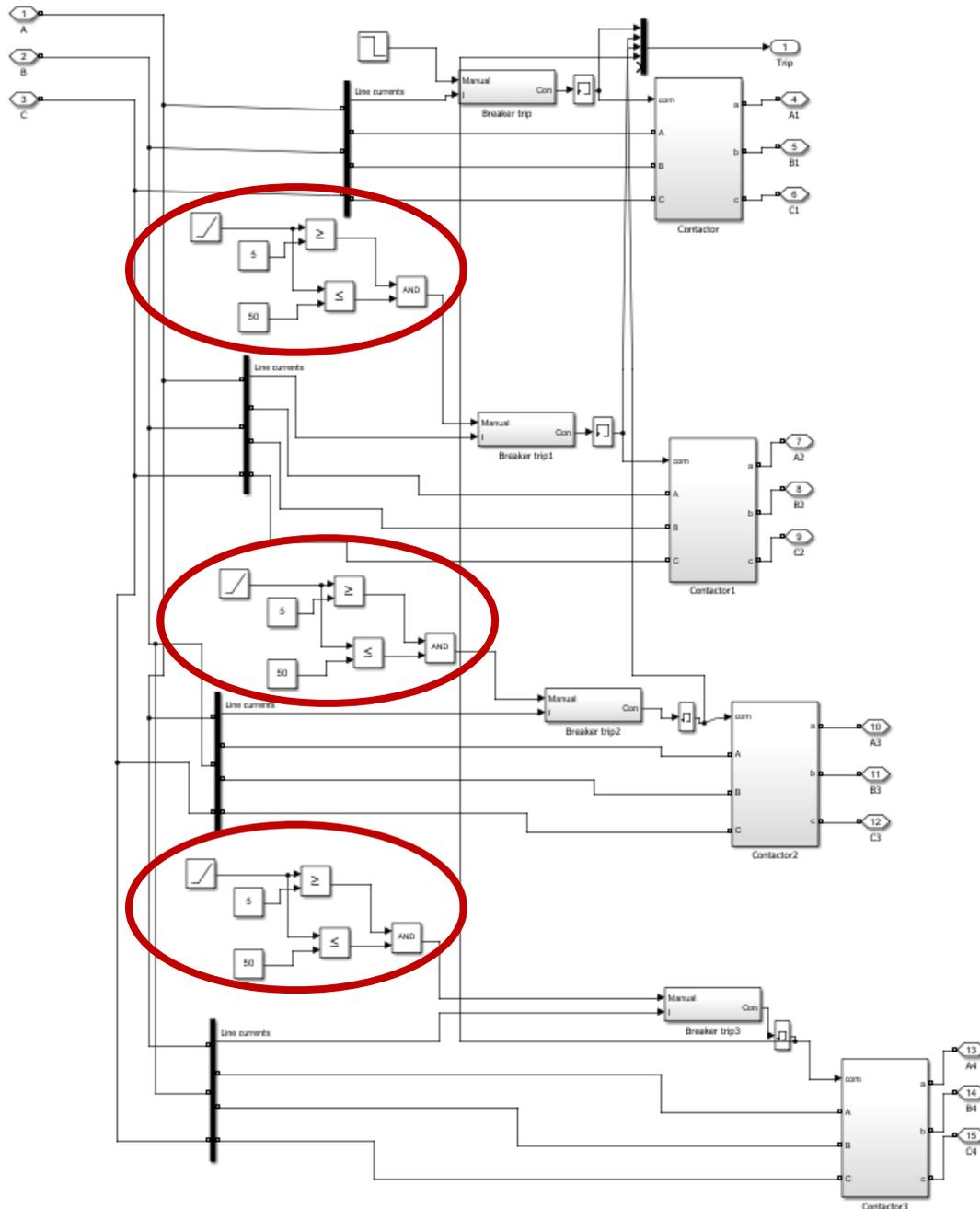
Figure 124 - Under the mask of the secondary distribution block in MATLAB
