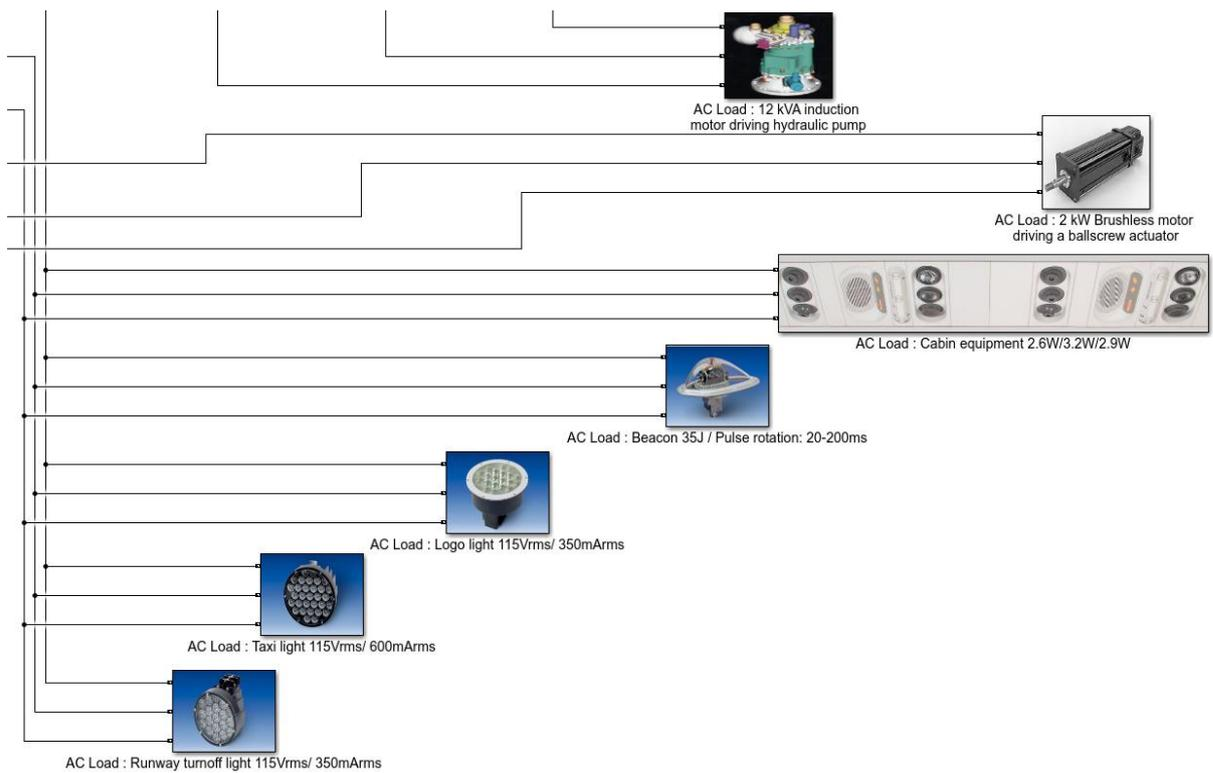
Figure 153 - Airbus A320 final schematic in MATLAB (4/4 parts)
