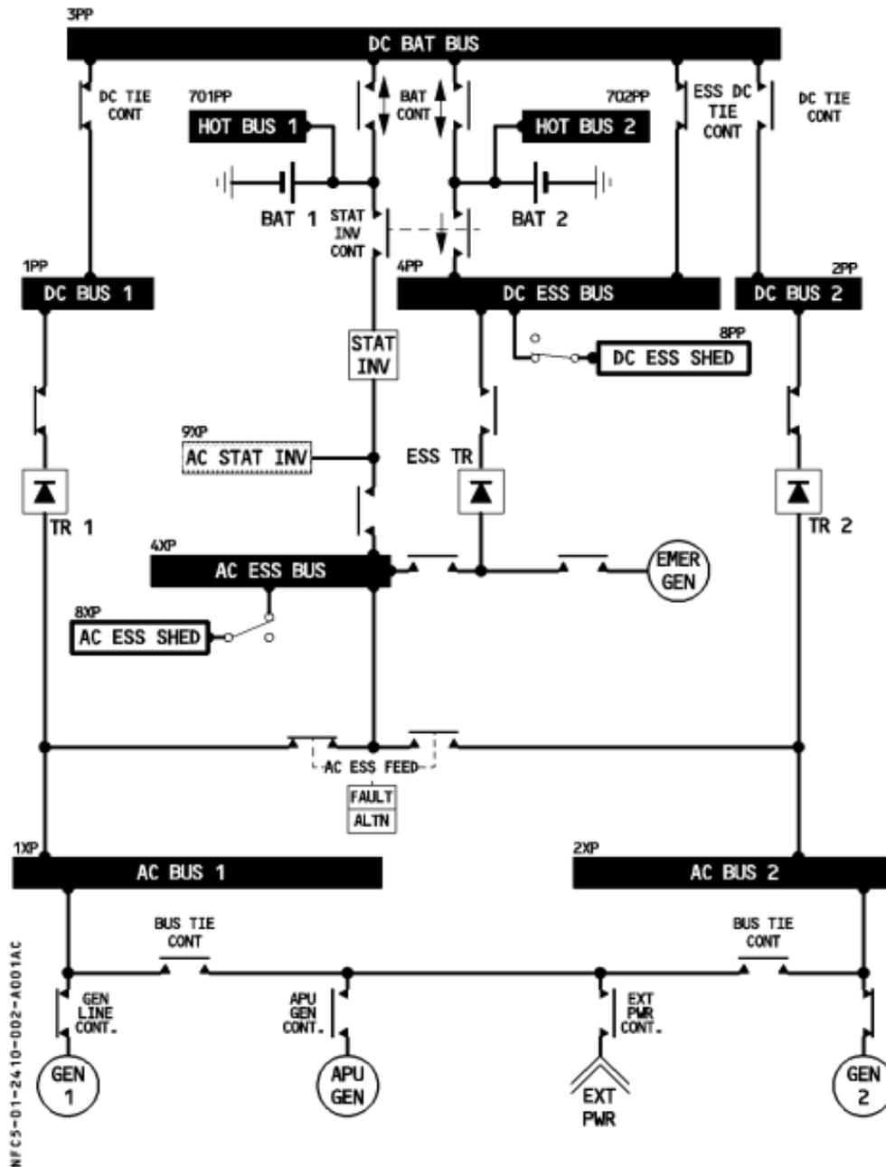
Figure 148 - Airbus A320 electrical system schematic
