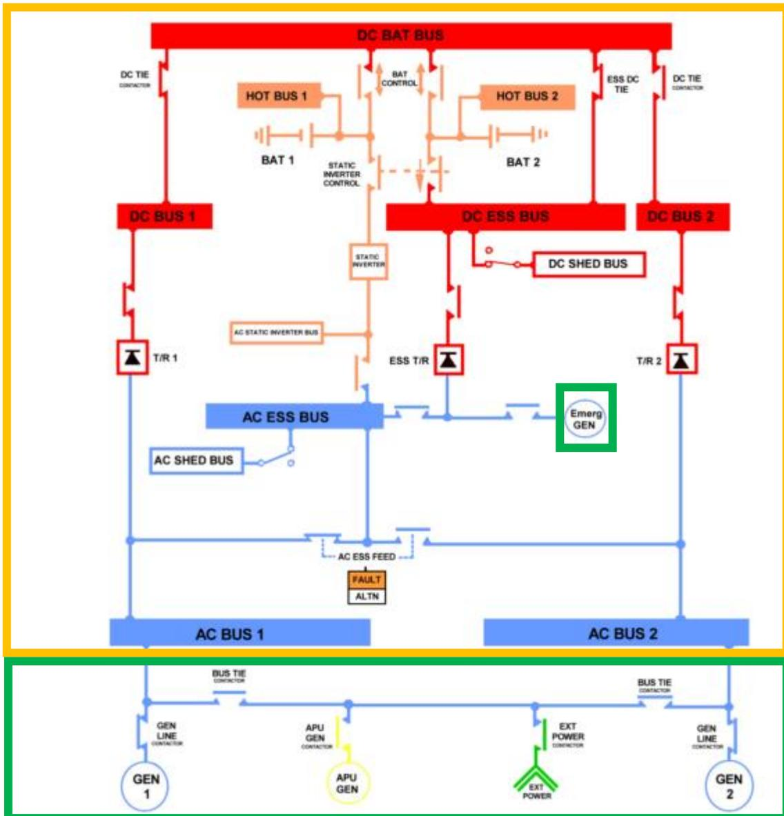
Figure 13 - Electrical system schematic divided in two parts [27]
