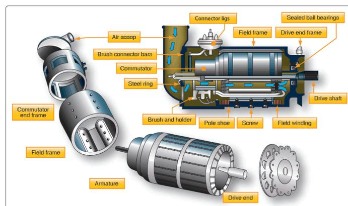
Figure 14 - Aircraft generator parts [23]
