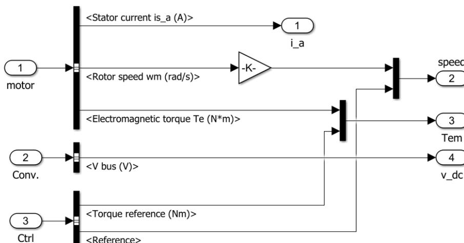
Figure 95 - Subsystem of the demux block parameter in MATLAB
