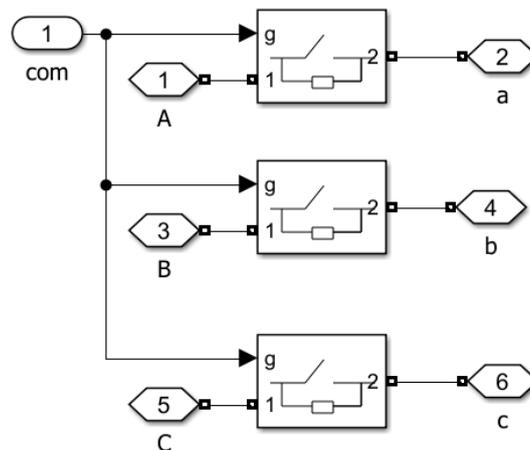
Figure 88 - Subsystem of the contactor block in MATLAB
