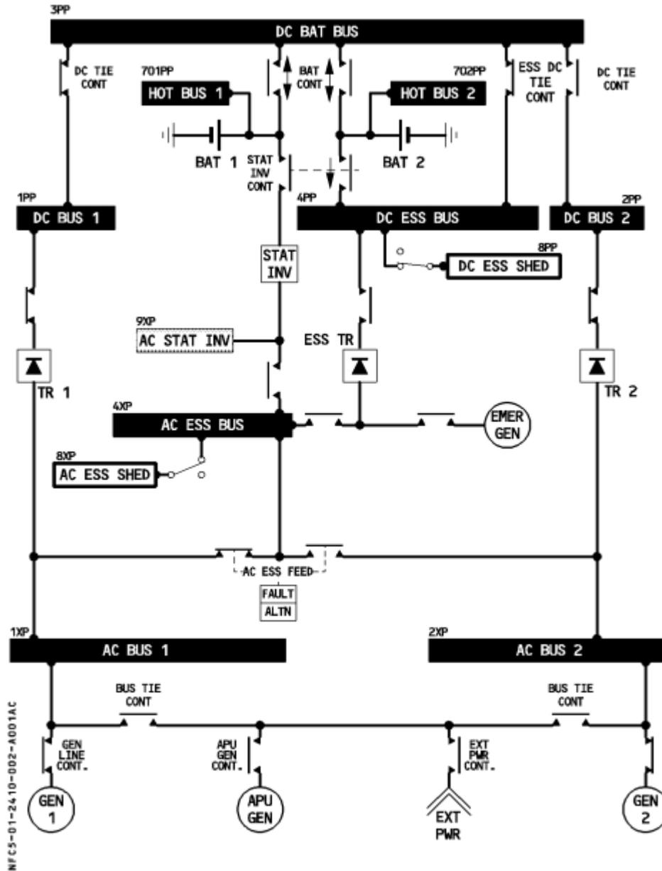
Figure 103 - Airbus A320 electrical system schematic
