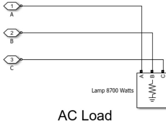
Figure 127 - Under the mask of the cabin equipment block in MATLAB
