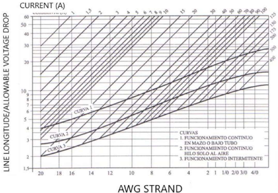
Figure 70 - Plot for the section calculation according to FAA [14]
