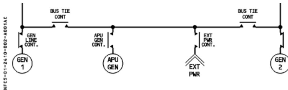
Figure 38 - Generating system of an Airbus A320 [38]
