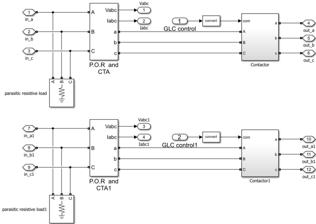
Figure 121 - Under the mask of the primary distribution in MATLAB
