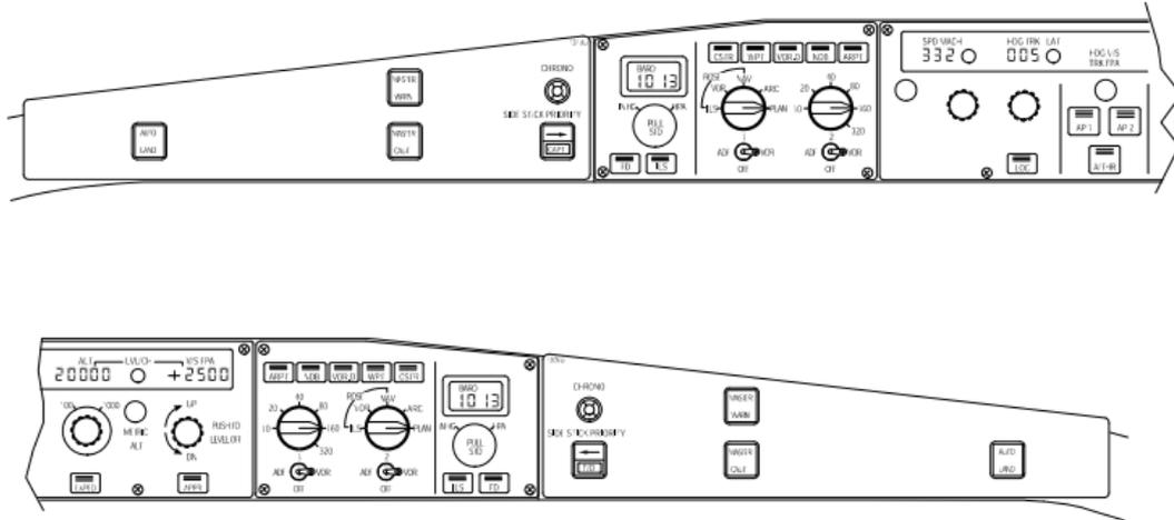
Figure 34 - Glareshield of an Airbus A320 [39]
