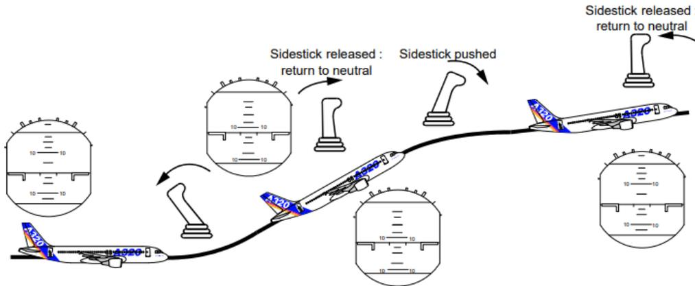
Figure 32 - Sidestick operation of an Airbus A320 [39]
