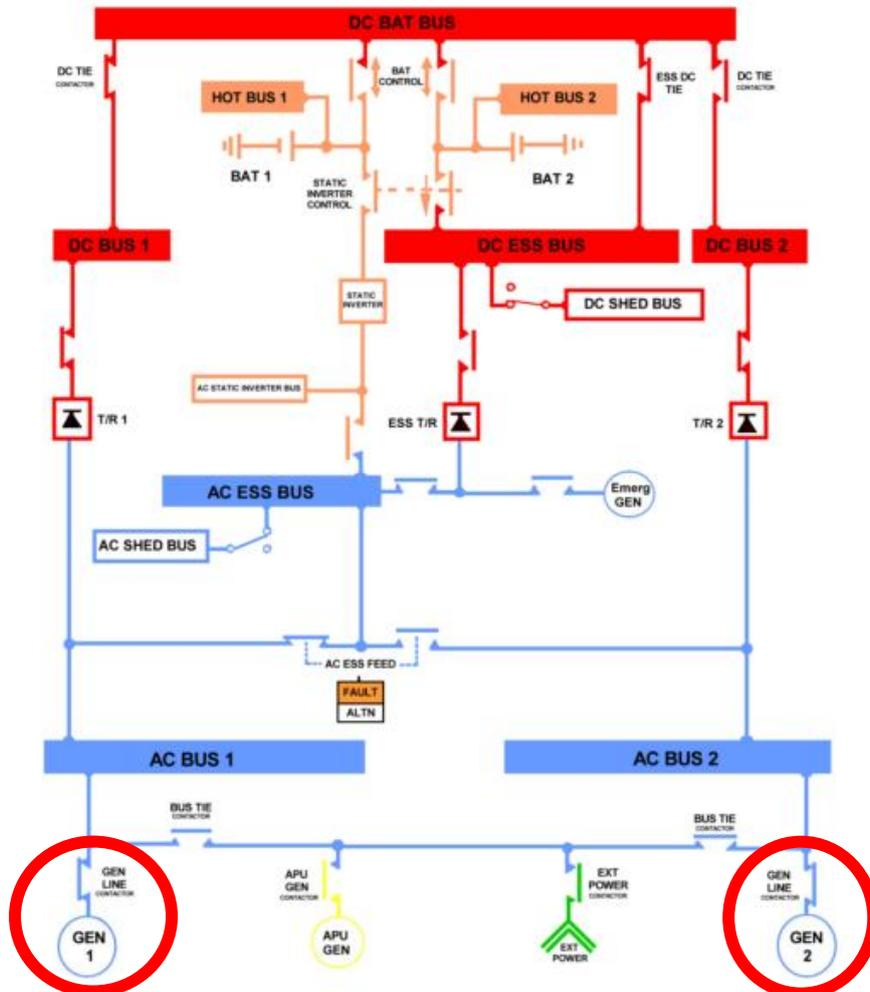
Figure 10- Generation system detailed on an electrical system schematic [27]
