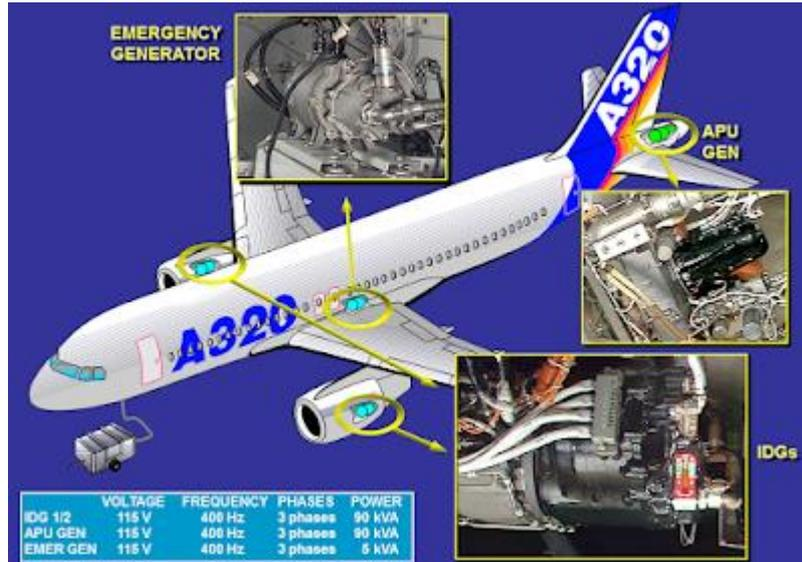
Figure 59 - Airbus A320 generation system distribution [40]
