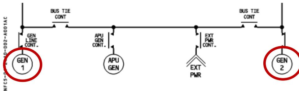
Figure 39 - Generating system of an Airbus A320 (GEN 1 & GEN2) [38]
