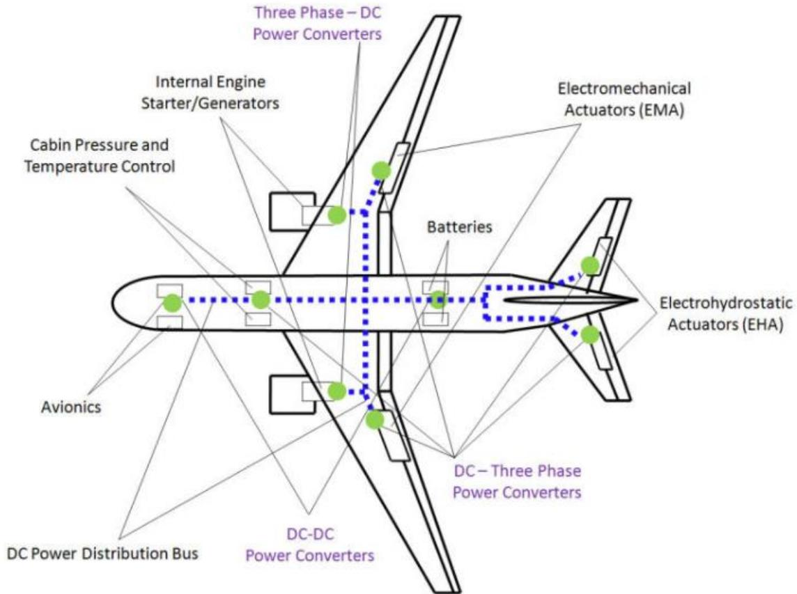
Figure 2- Power distribution system (PDS) of a commercial aircraft [31]
