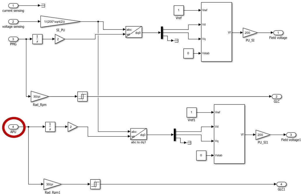
Figure 119 - Under the mask of the GCU block in MATLAB
