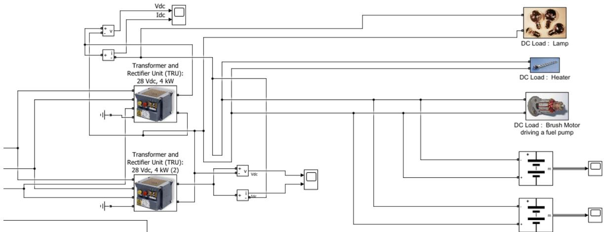
Figure 152 - Airbus A320 final schematic in MATLAB (3/4 parts)
