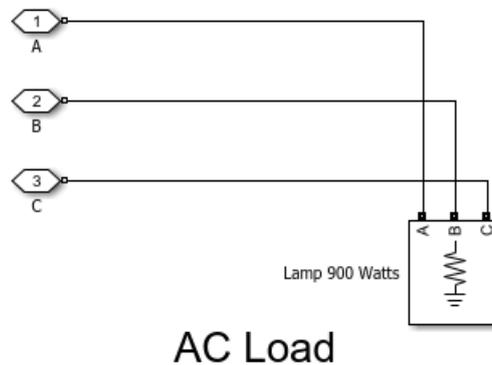
Figure 132 - Under the mask of the logo light in MATLAB
