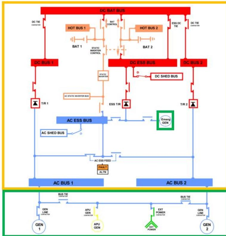
Figure 37 - Electrical system schematic divided in two parts [27]
