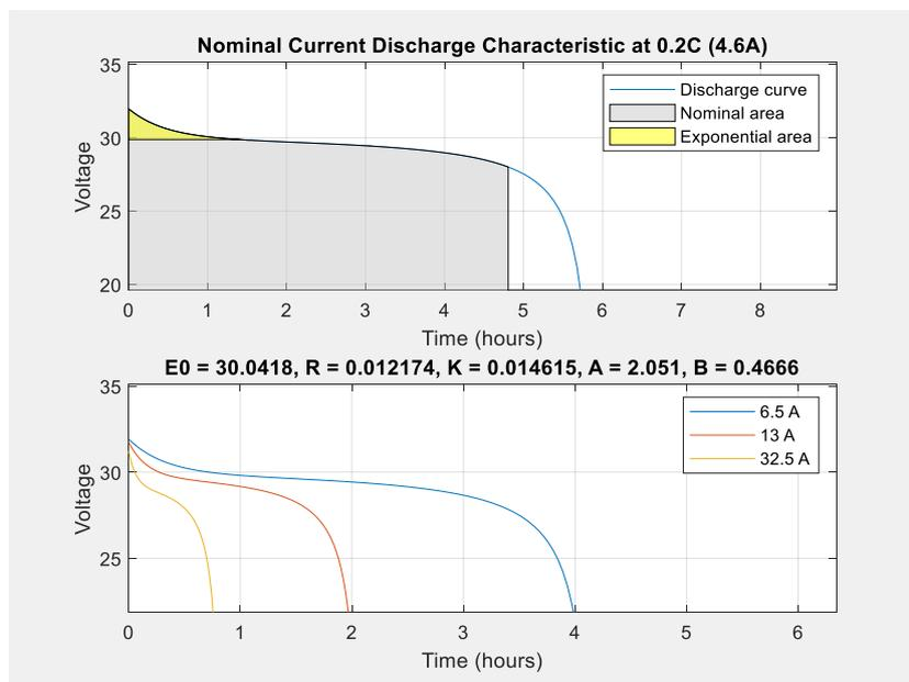
Figure 147 - Battery discharge characteristic
