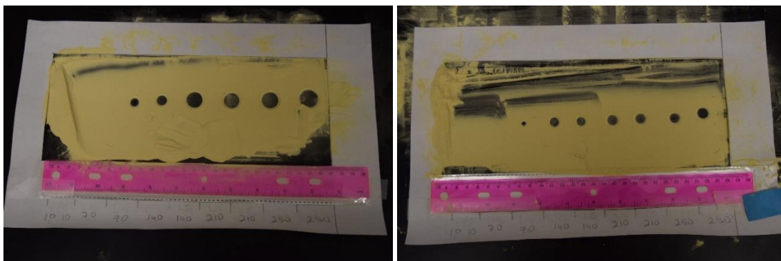
Fig. 3. Trial at 1.0 cm distance and with an air-flow duration of 0.9 s without (left) and with (right) the brass nozzle adapted on the exit-jet.
