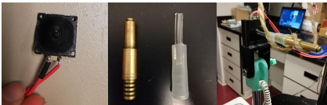
Fig. 1. Blower of the new aesthesiometer without the brass nozzle (left), brass nozzle and adaptor (centre) and brass nozzle adapted on the micro-blower (right).
