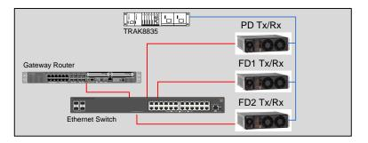
Figure 1-2: Basic Diagram of Ulster Analog Simulcast Remote Site with FD & PD Chanels
