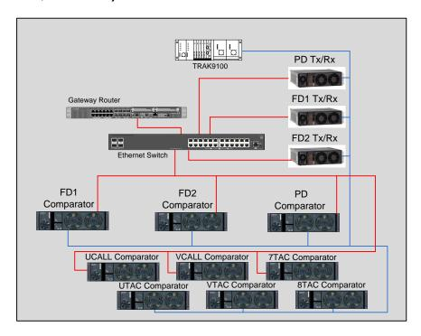
Figure 1-1: Basic Diagram of Ulster Analog Simulcast Prime Site
