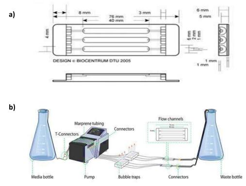
Figure 2-2 Flow cell model 2 from DTU.
