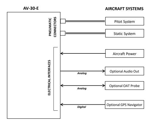
Figure 2 - AV-30-E Aircraft Systems Interfaces - AI Mode
