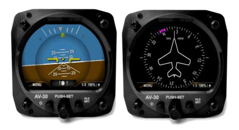
Figure 1 - AV-30-E Multi Mode Al/DG - Basic Display
