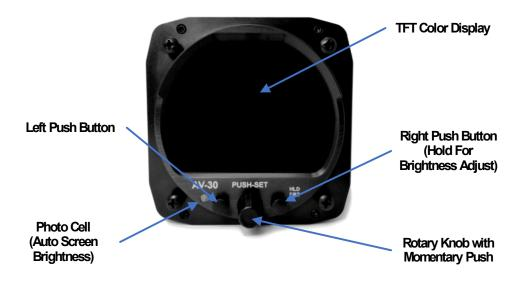
Figure 5 - Common User Interface Components
