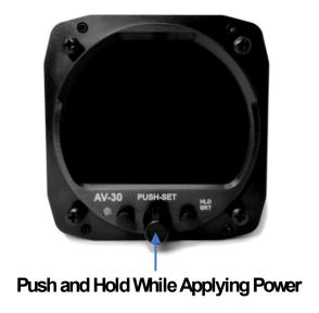
Figure 38 - Installation Menu Access
