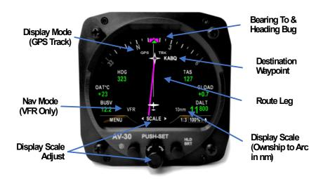
Figure 20 – GPS ARC Mode
