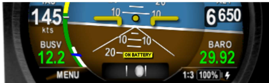
Figure 39 - On Battery Operation
