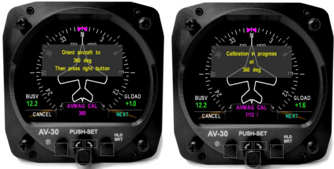
Figure 29 – AVMAG CAL In-Progress
