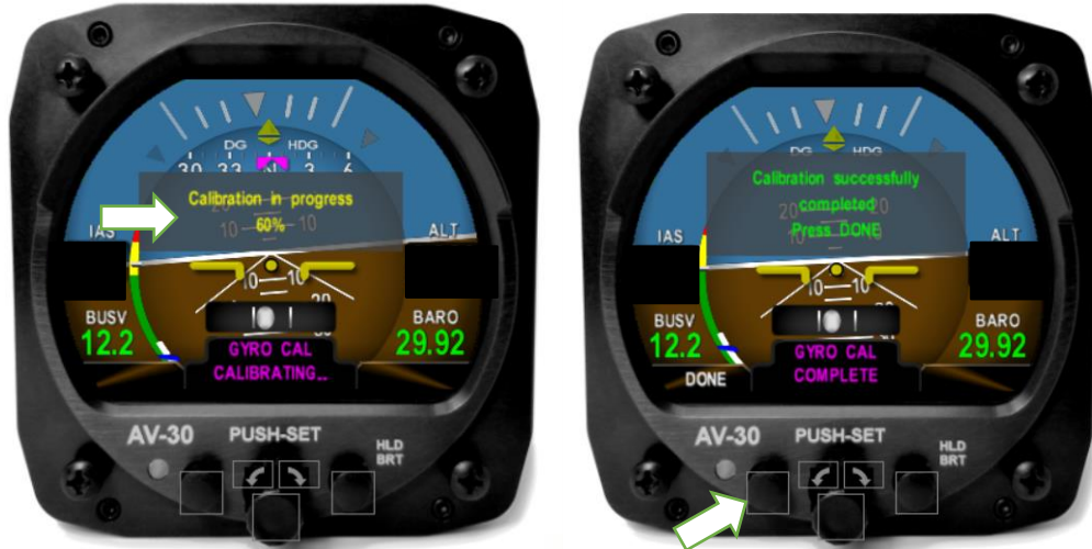
Figure 26 - Gyro Calibration Procedure
