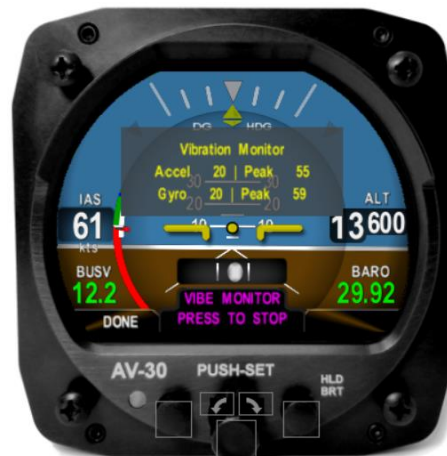
Figure 35 - Vibe Monitor Operation
