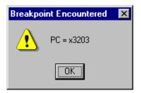
Click OK, and notice what has changed in your registers. The blue arrow and the PC both point to line x3203. R4 is unchanged – it contains x5. R5 has changed – it contains x2. R2 has changed – it contains x5. The condition codes have P=1. That tells you that when you continue to run the program, the branch will be taken.
