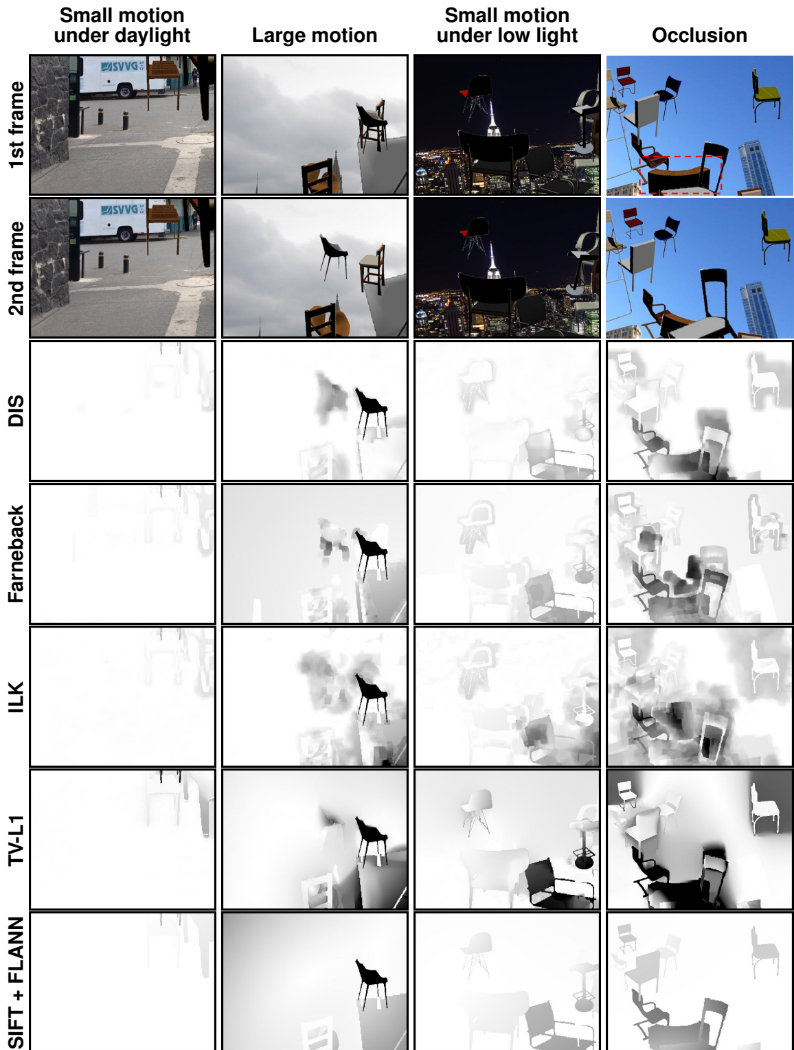
Figure 8.8. The results of the grayscale absolute error of optical flow estimated by conventional methods for four different scenarios: small motion under daylight conditions, large motion, small motion under low light conditions, and occlusion. White regions indicate where the motion is correctly estimated, while black regions refer to the motion is not correctly estimated. The grayscale images range between [0, 1] .
