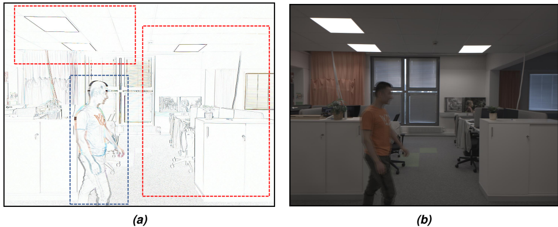
Figure 1.2. (a) Misalignment between two consecutive processed raw images due to global camera motion (the regions indicated by the red rectangles) and object movement (the region indicated by the blue rectangle) in the scene. (b) Ghosting artifacts due to the pixel shift.
