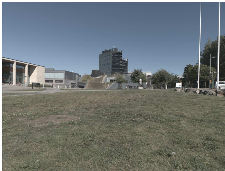
Figure 2.6. Image as in Fig. 2.3 but BLC, LSC, WB, and OETF applied.
