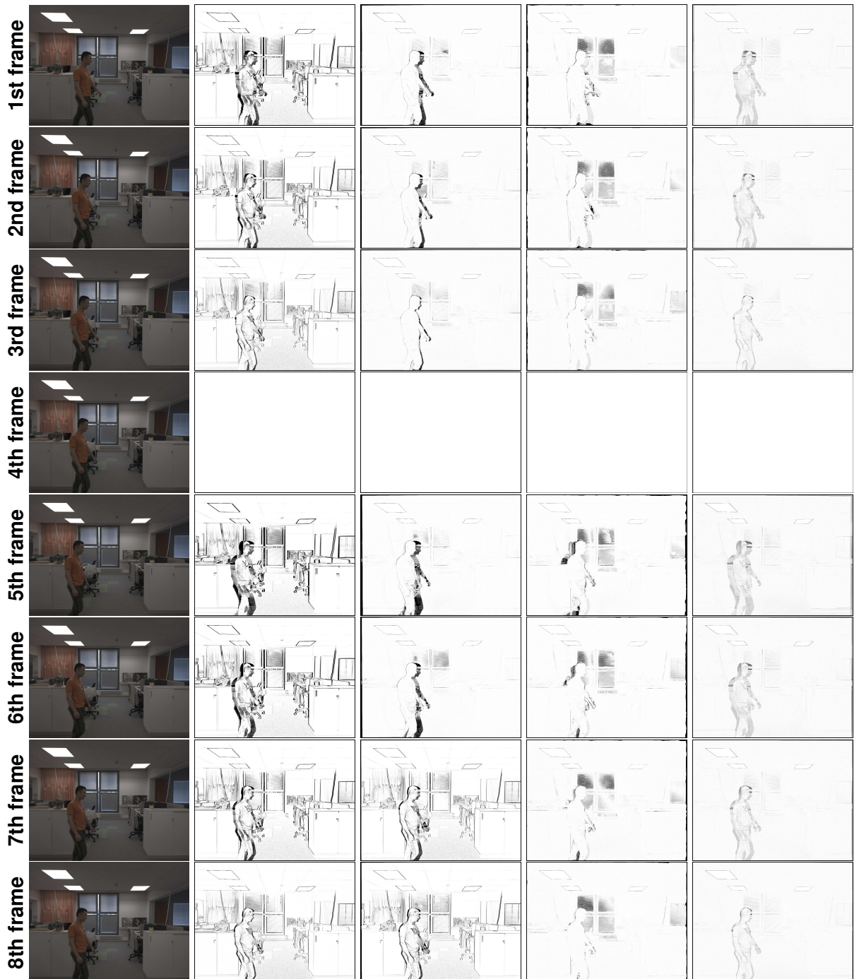
Figure 8.18. Processed raw image frames and delta images before and after alignment. From left-most to right-most, columns refer to multi frames, delta images before alignment, delta images after alignment, where pixel shifts are estimated by the CSFlow, DIS, and SIFT + FLANN methods, respectively.
