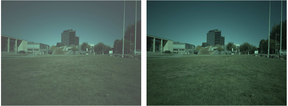
(a) Image as in Fig. 2.3 but Opto-Electronic Transfer Function (OETF) applied. (b) Image as in Fig. 2.3 but BLC and OETF applied.
