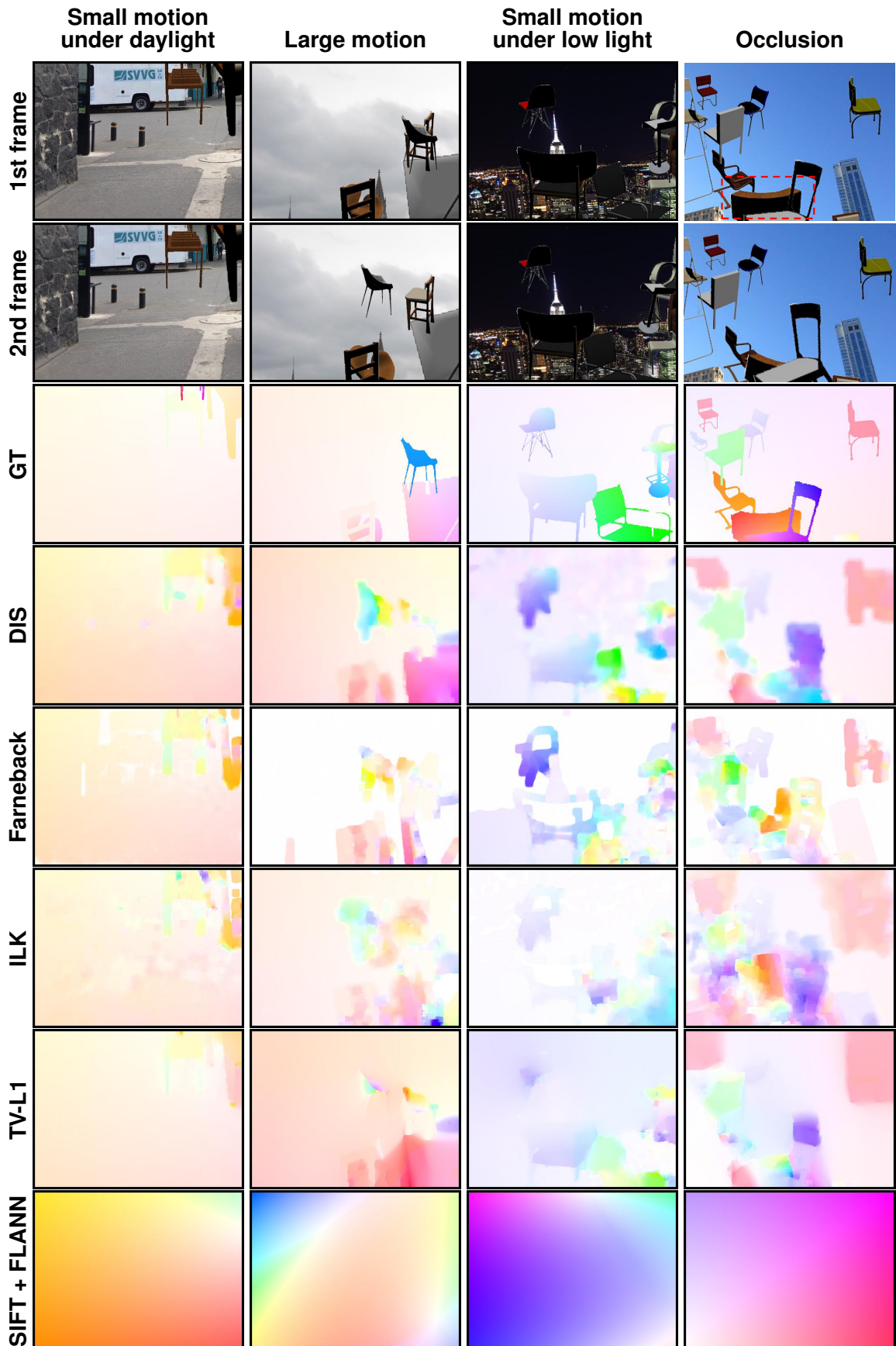
Figure 8.7. Color-coded results of optical flow estimated by conventional methods for four different scenarios: small motion under daylight conditions, large motion, small motion under low light conditions, and occlusion.
