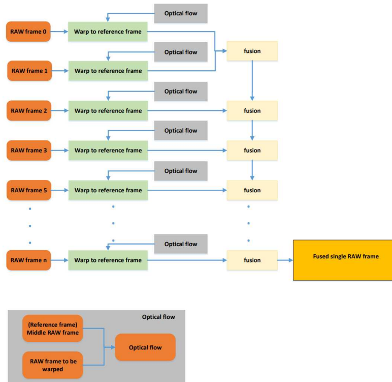
Figure 1.3. Raw bayer domain image alignment and fusion pipeline.
