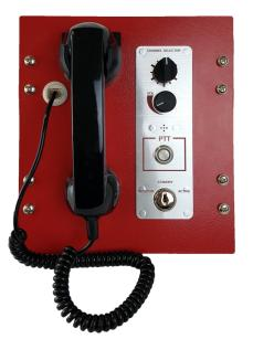
When building codes require isolated operations, literally isolating all communications to the incident building, a Channel Control Unit is required. By default, isolated radio enhancement systems are in a standby state and only activated during a incident.
