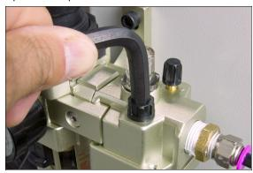
Figure 2-2: Fill port on an FRL.
