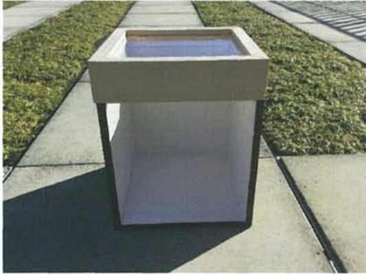
Figure 8-C-1. A Skylight without Glass Balls
