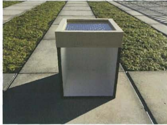
Figure 8-C-2. A Skylight with One Layer of Glass Balls
