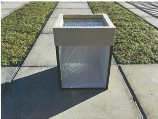
Figure 8-C-3. A Skylight with Two Layers of Glass Balls
