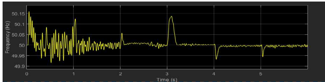
Fig 5: Frequency transients at 0.8 lagging power factor
