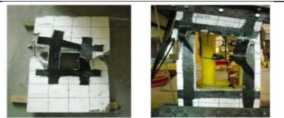
Figure 24: Crack patterns on the tension face after failure of the 40mm thick wall panels with openings strengthened with CFRP pattern 1. [23]
