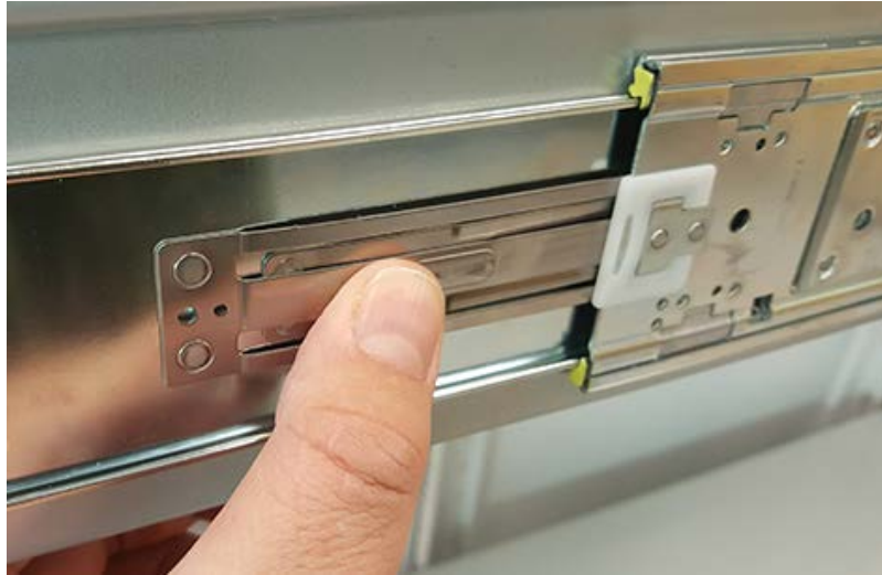
Figure 100: Safety Latch Release
