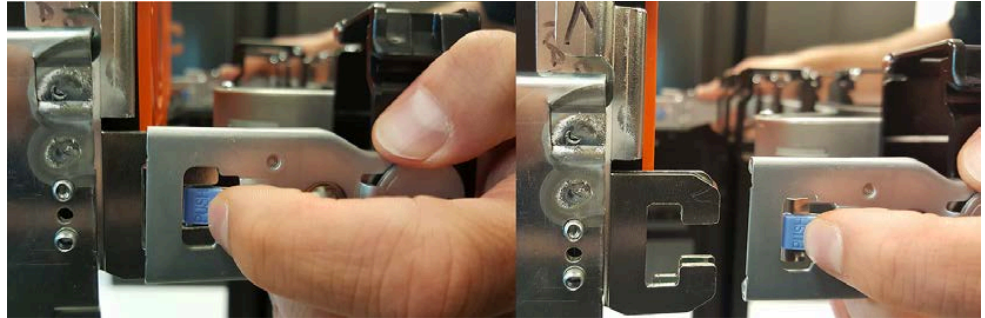
Figure 90: Unlatching a CMA Connector
