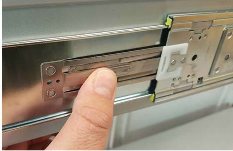
Figure 73: Safety Latch Release
