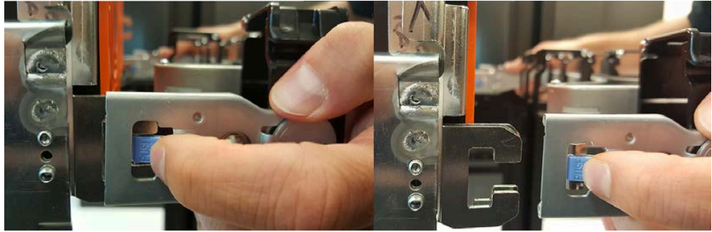
Figure 68: Unlatching a CMA Connector
