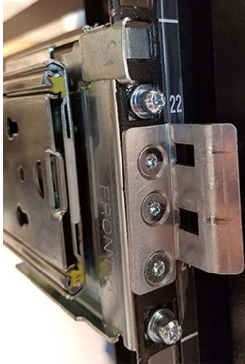
Figure 104: Rack Latch Bracket Installed
