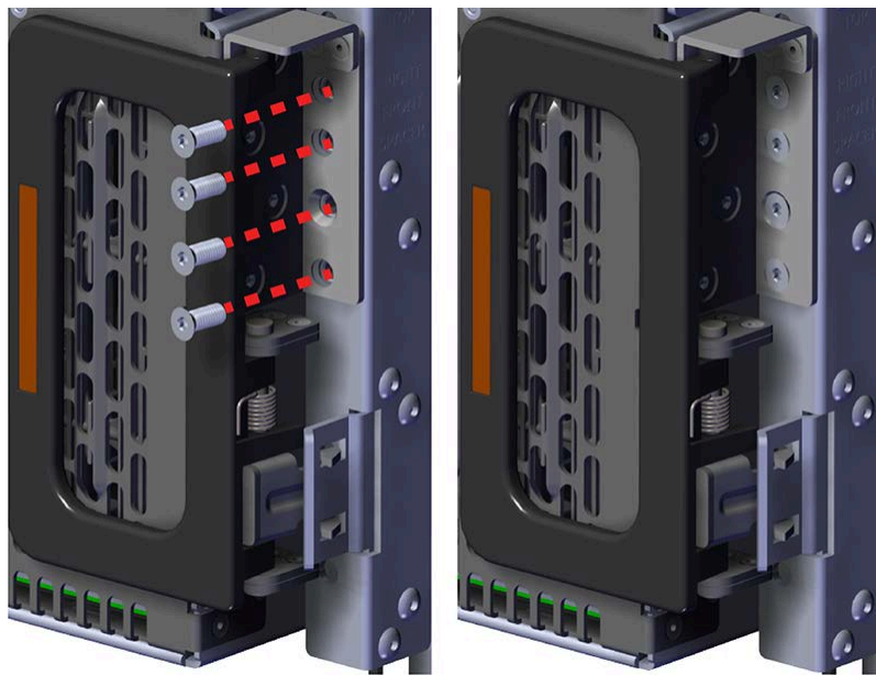
Figure 98: Shipping Bracket Screw Locations (CMA Lite)
