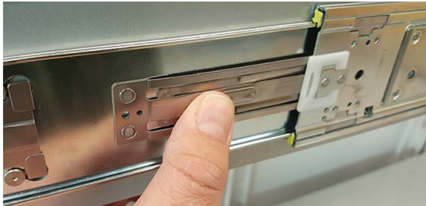
Figure 159: Inner Rail Safety Latch Release
