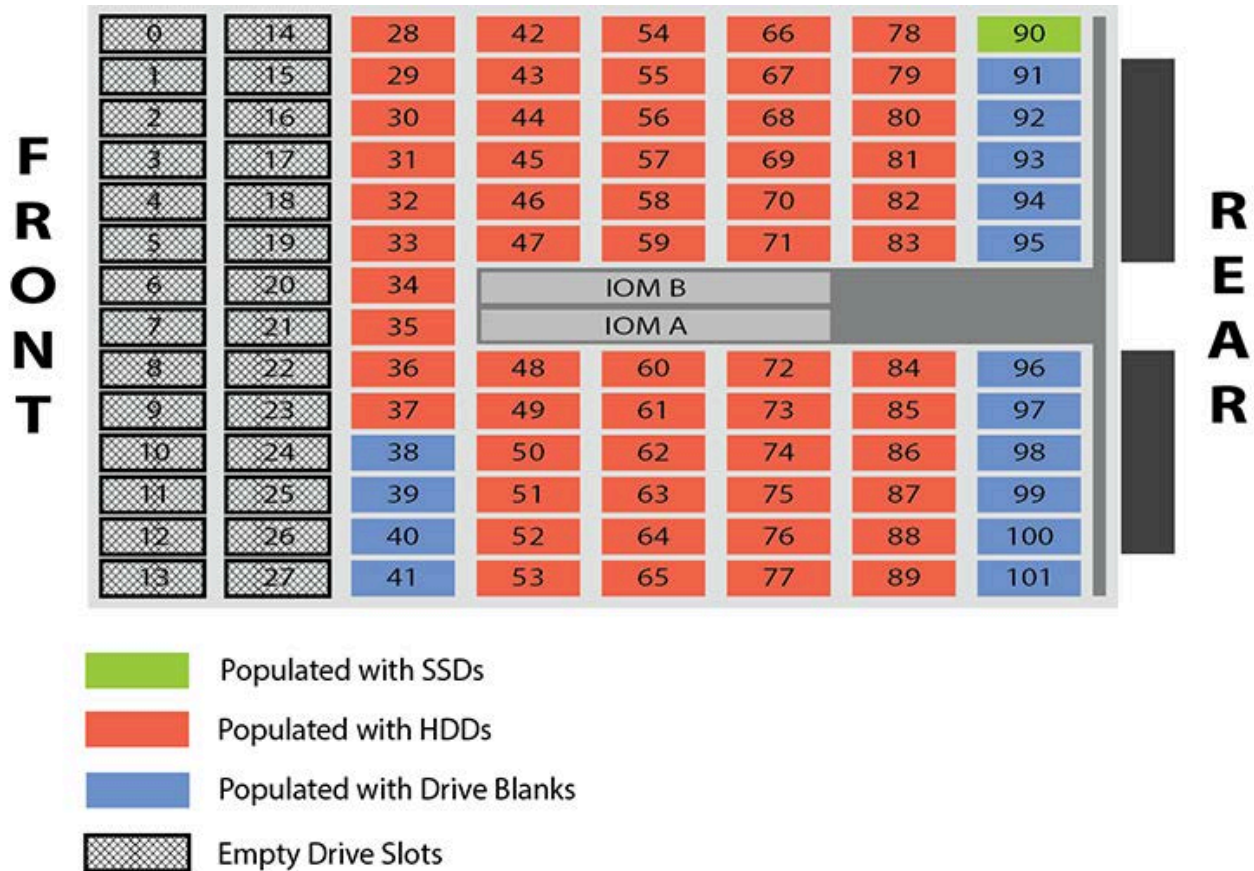
Figure 223: Minimum HDD and Minimum SSD Partial Population
