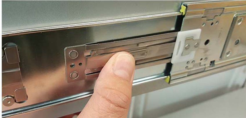
Figure 74: Inner Rail Safety Latch Release
