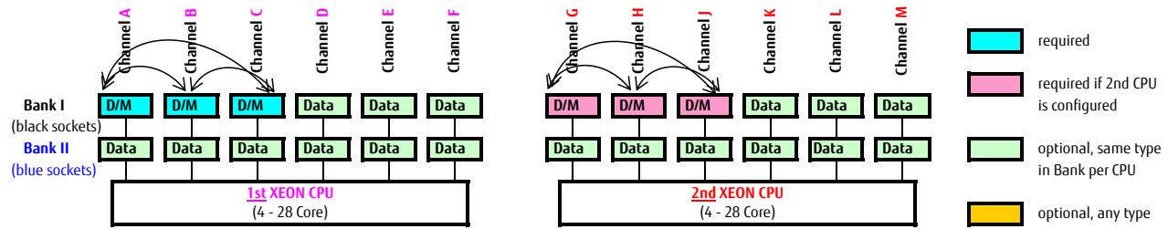
Mirrored Channel Mode (3 DIMMs per CPU) requires identical modules on channel A, B & C (1st CPU) or channel G, H & J (2nd CPU) 50% of the capacity is used for the mirror => the available memory for applications is only half of the installed memory. If this mode is used, a multiple of 3 identical modules has to be ordered.
