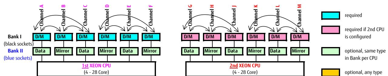
Mirrored Channel Mode requires identical modules on channel A, B, C, D, E, F (1st CPU) or channel G, H, J, K, L and M (2nd CPU) 50% of the capacity is used for the mirror => the available memory for applications is only half of the installed memory. If this mode is used, a multiple of 6 identical modules has to be ordered.
