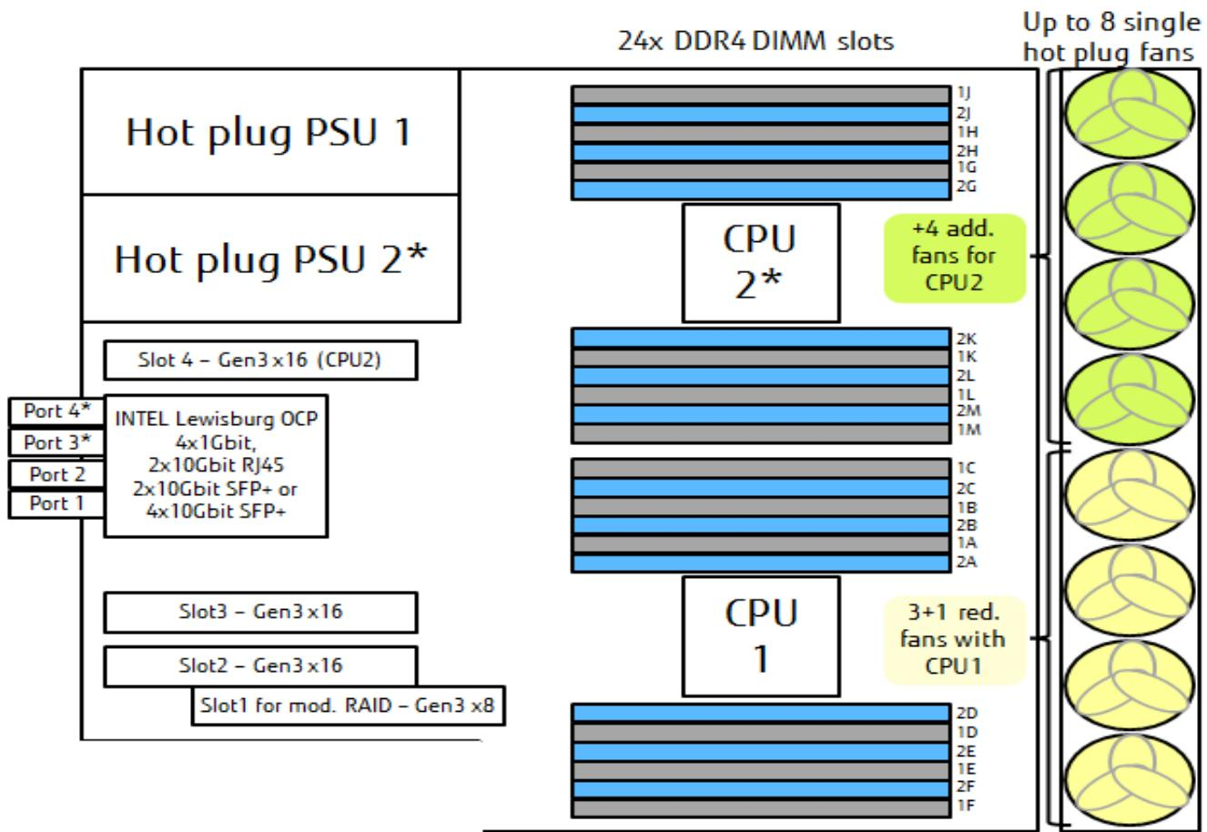
**PRIMERGY RX2530 M4 rear view with PSU, PCIe slots and dynamic LoM**
