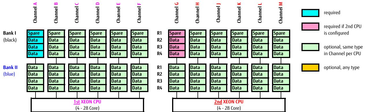
Rank Sparring Mode requires identical modules (same capacity and technology) within the same channel. The available memory for applications will vary depending on configuration. Please refer to the spreadsheet above "Effective Memory capacity with active Rank Sparring Mode". Population rule for Rank sparing mode is to achieve max. available memory, e.g. 4 DIMMs will be spread across two channels, each with 2DPC
