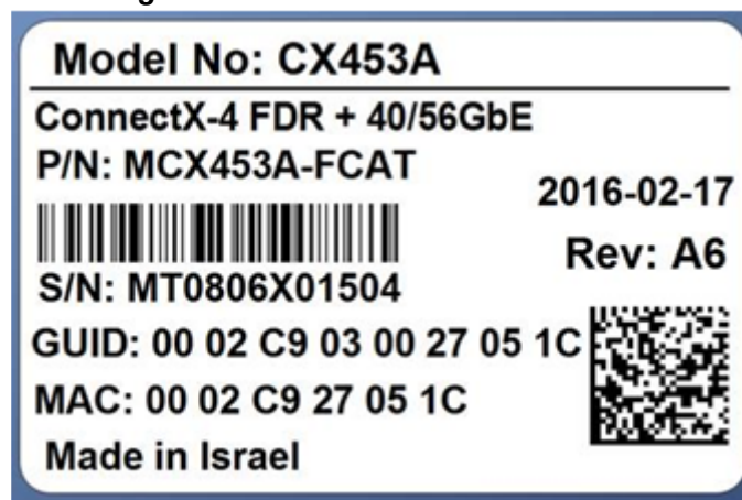
Figure 11: MCX453A-FCAT Board Label
