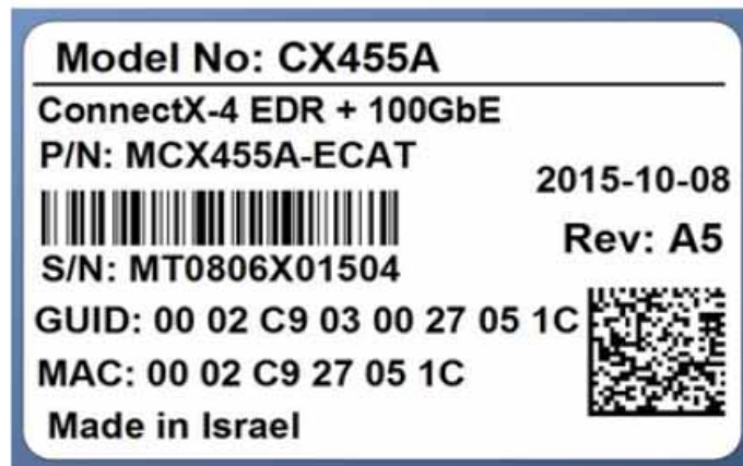
Figure 15: MCX455A-ECAT Board Label
