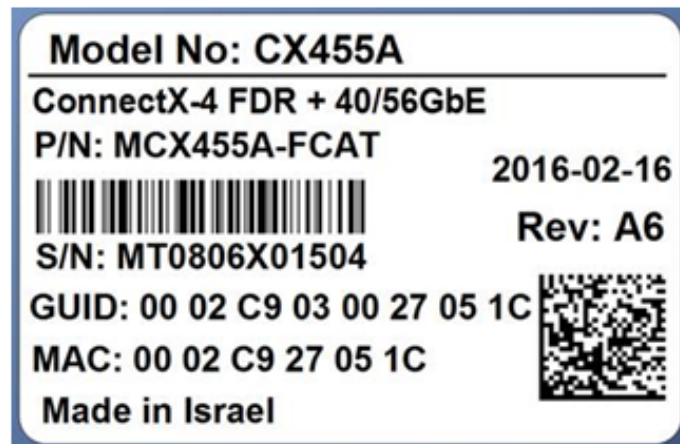
Figure 13: MCX455A-FCAT Board Label
