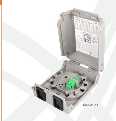
The 169F Fiber Interface Device/Slack Storage Unit is a compact enclosure which is designed to provide a demarcation and transition point between fiber drop cable and the customer premise fiber cable. Designed as an adapter plate for Tii's 169 Sealed Wire Terminal Enclosure, the unit can be factory installed with industry standard single, dual or quad fiber adapters. The internal fiber routing system allows for proper bend radius and slack storage of bend insensitive fiber.
